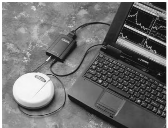
Figure 2. A receiver and antenna for the Inmarsat-D high-penetration messaging system. The receiver is shown connected to a laptop computer. (Reprinted with permission from Skywave Mobile Communications, Inc.)
