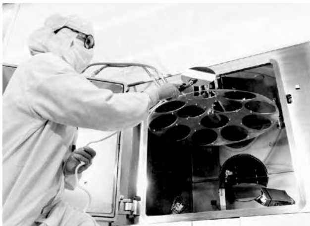
Figure 9. Evaporation system for metallizing semiconductor wafers.
