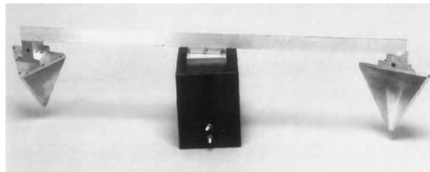
Figure 23. A motorized set of trihedrals provides a moving target for W band. Note the angle offset between the support arm and the trihedrals. This offset was designed so that the “flash” from the arm, as it becomes normal to the radar wave, will not occur at the same time as the peak of the trihedral response.
