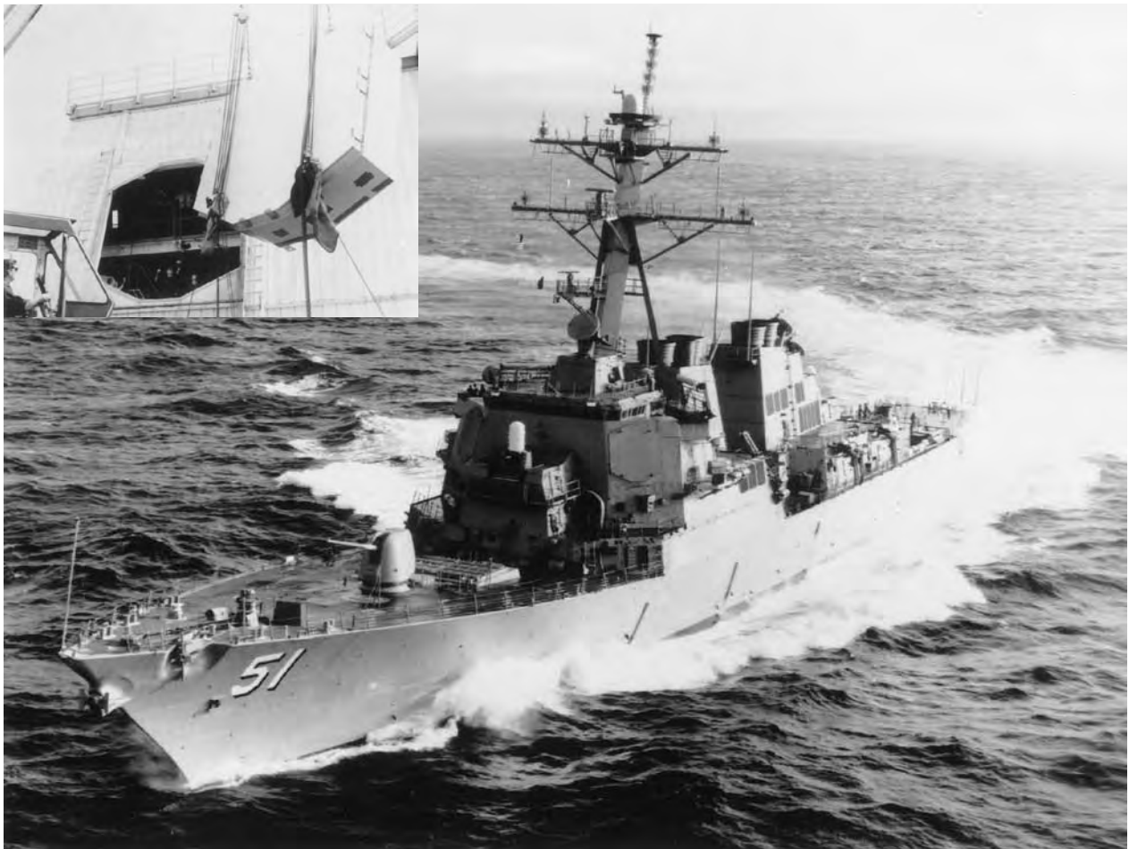
Figure 28. The Arleigh Burke (DDG-51) Aegis system is based on the AN/SPY-1D multifunction phased-array S-band radar. The SPY-1 antennas are the octagonal panels on the corners of the deckhouse. The inset in the upper left shows an antenna being installed in a deckhouse. (U.S. Naval Institute collection.)
