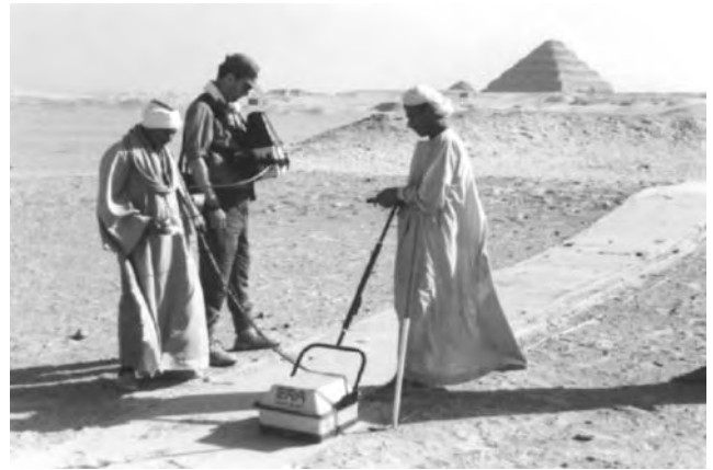
Figure 10. GPR system in use for archaeological surveying in Saqqara, Egypt. (Courtesy of ERA Technology.)
