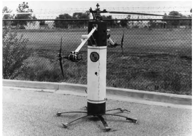
Figure 23. EAGER shipboard-tethered decoy in field trials.
