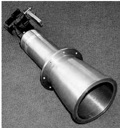
Figure 38. Monopulse tracking feeds: (a) multifeed array (From Lee and Chu [95], courtesy of IEEE); (b) multimode monopulse feed.
