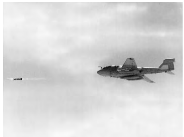
Figure 4. HARM missile (shown after separation from an EA-6B aircraft) is an EW weapon for physically destroying the source of hostile radiation.
