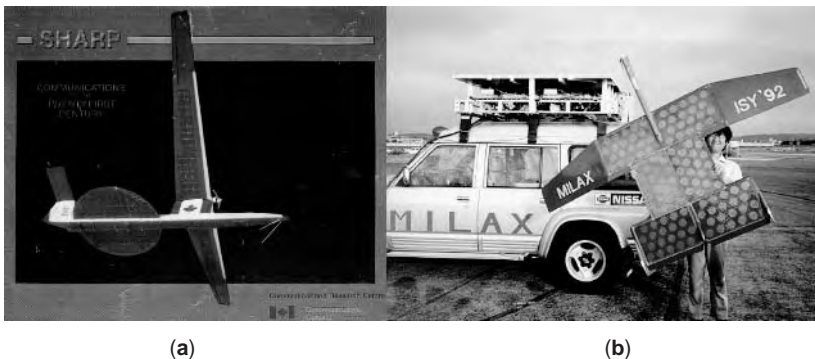
Figure 15. MPT applied to unmanned remotely powered model aircraft: (a) SHARP; (b) MILAX.
