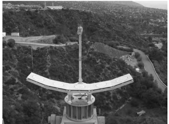
Figure 15. Drawing and photo of the piecewise flat reflectarray for space application.
