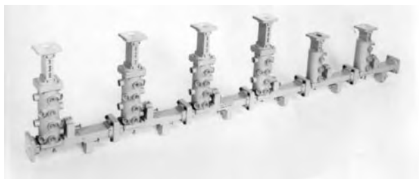
Figure 16. Waveguide channel dropping multiplexer for communication application. The bandpass channel filters are dual-mode and are connected to the common manifold, isolated using band-stop filters between each bandpass channel.
