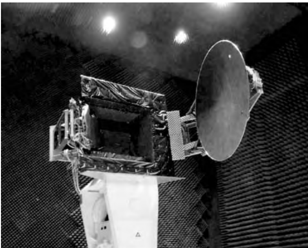
Figure 7. International C-band Tx hemizone antenna system mounted on a satellite mockup during compact range tests. (Courtesy of EADS Astrium.)
