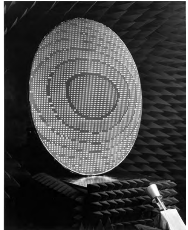
Figure 10. Ku-band reflectarray with shaped contour beam capability (courtesy of Professor Dave Pozar, Univ. Massachusetts). (This figure is available in full color at http://www.mrw.interscience.wiley.com/erfme .)
