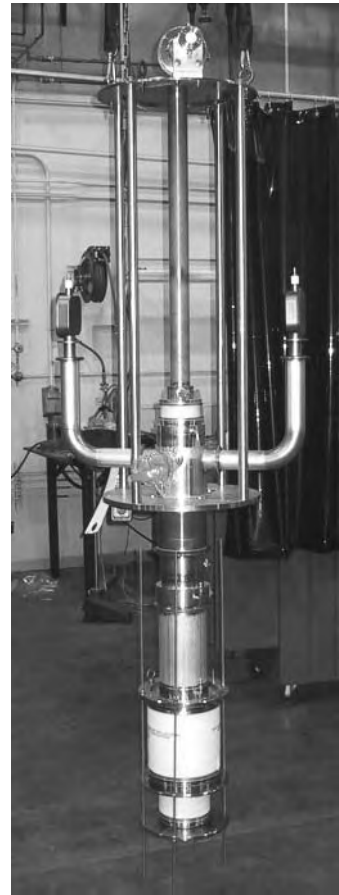
Figure 9. A 10-MW, 91-GHz gyrokyklystron under development for high-power accelerator research.
