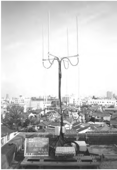
Figure 57. An example of practical base-station adaptive antenna. (From [1] with permission from Wiley.)
