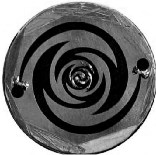
Figure 16. Photographs of unconventional four-arm (a) and two-arm (b) sinuous antennas with sketched lossless cavity backing. (This figure is available in full color at http://www.mrw.interscience.wiley.com/erfme .)
