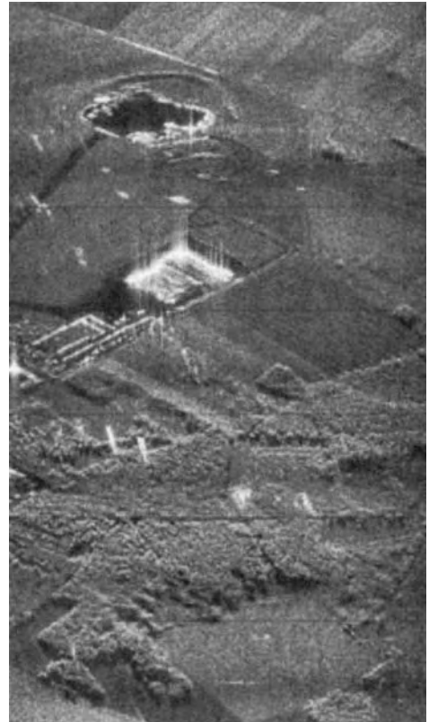
Figure 14. An example of an ESAR-2 stripmap SAR image. It is processed by the range-migration algorithm. [The ESAR-2 data were made available by courtesy of the German Aerospace Research Establishment (DLR).]
