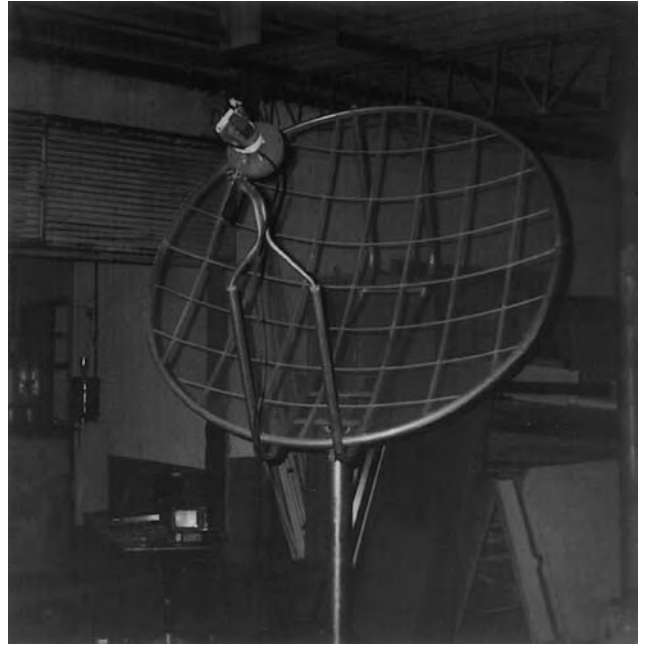
Figure 10. Just fully offset parabolic reflector antenna built and tested for satellite TV reception at C band. (Courtesy of Carlos Muller, Univ. Brasilia.)
