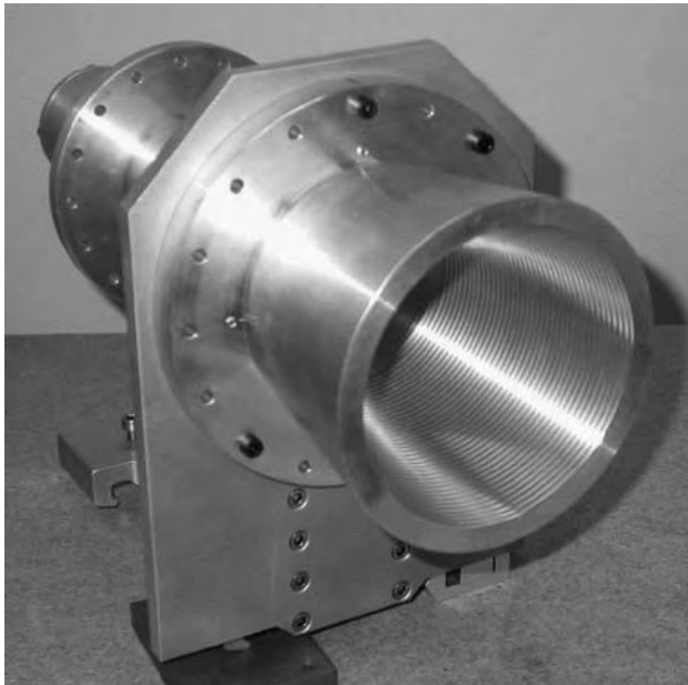
Figure 15. High-gain feed horn at 32 GHz (Courtesy of the Institute of Radioastronomy of the Italian National Research Council.)
