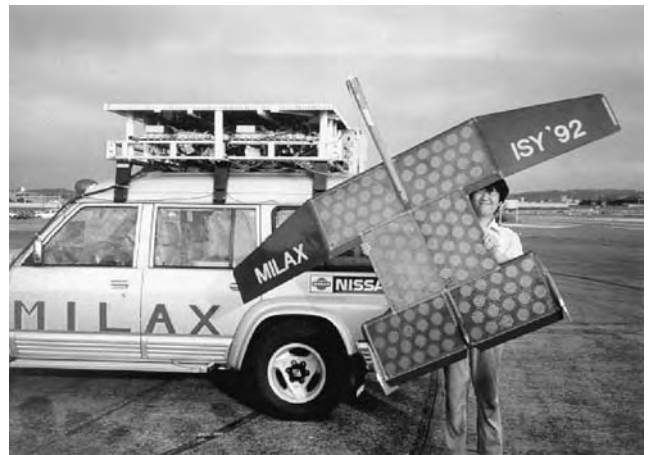
Figure 12. Application of microwave power transmission to microwave-driven airplane (MILAX fuel-free flight experiment).
