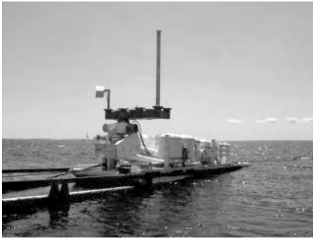
Figure 24. SSTP (with a mast system mounted topside) transiting on guiderails toward test position in Long Island Sound, NY. The frequency range of testing is 100 MHz–18 GHz.
