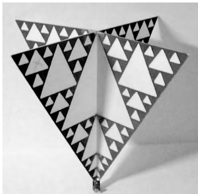
Figure 14. 3D antenna solution used to tailor the antenna patterns at different frequency bands. The antenna is built with two planar structures based on the Sierpinski fractal.
