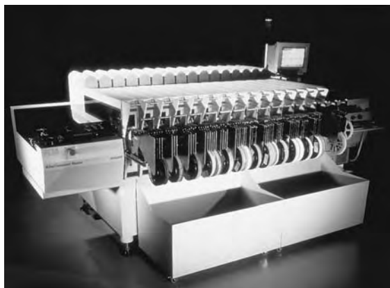
Figure 3. Example of high-speed chip placement equipment with placement rates in excess of 60,000 devices per hour. (Figure of Philips FCM courtesy of North American Philips.)
