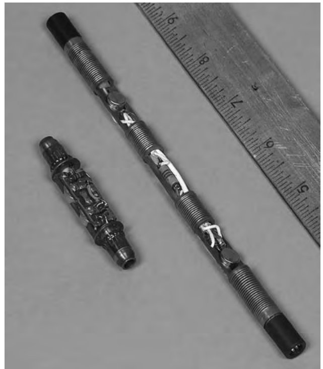
Figure 16. Solid-state inline amplifiers for a buoyant cable antenna: left —rigid chassis design (ca. 1970); right —flexible bellows model (1980–present).
