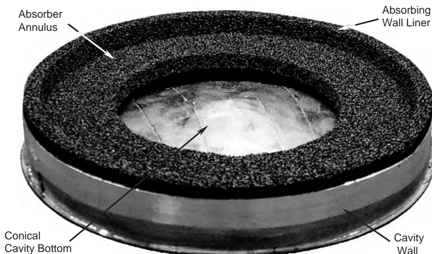
Figure 19. Photograph of a realized conical cavity with vertical and radial absorber liners.
