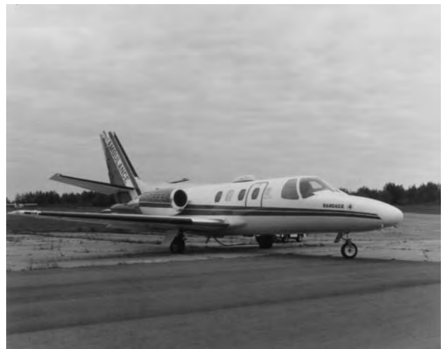
Figure 6. A Cessna Citation jet aircraft, operated by the Ontario Air Ambulance Service, equipped with a mobile satellite communications terminal. The antenna subsystem can be seen mounted on top of the fuselage.
