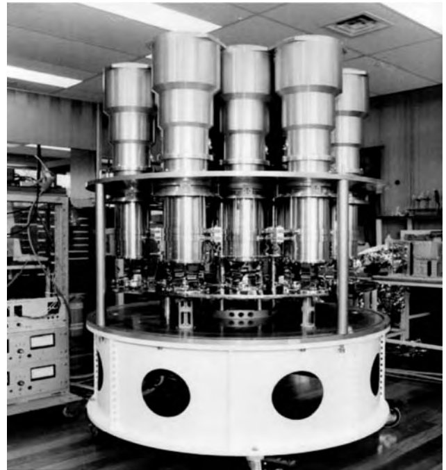
Figure 14. The 13-element multibeam feed system for the Parkes (Australia) radio telescope.
