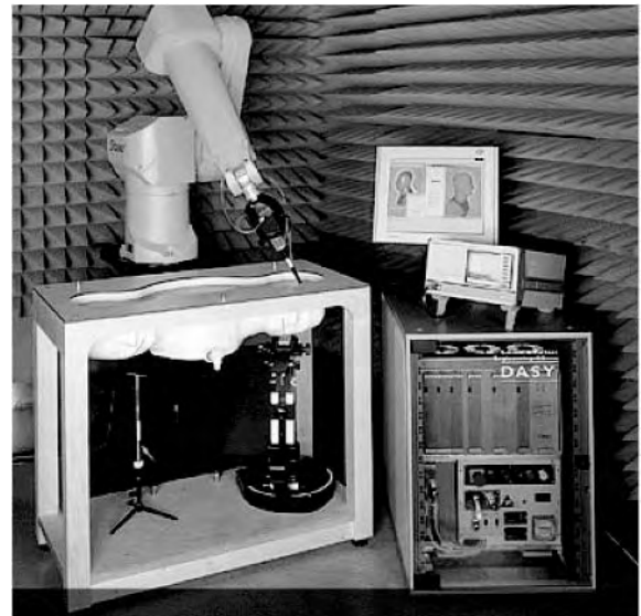
Figure 3. Commercial instrument used to measure SAR distribution produced by a mobile telephone in model of a human head. The robot arm moves an electric field probe inside a phantom model filled with a liquid whose electrical properties resemble those of a tissue. (From Ref. 3 with permission; available at http://www.dasv4.com/welcome.html .)
