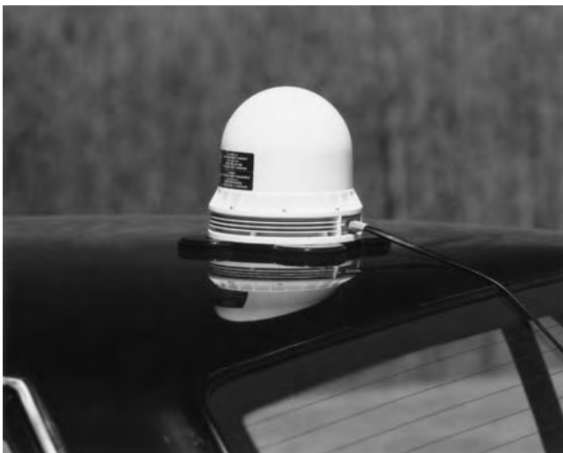
Figure 4. The antenna for a Mitsubishi MSAT telephone terminal, mounted on the roof of a car.
