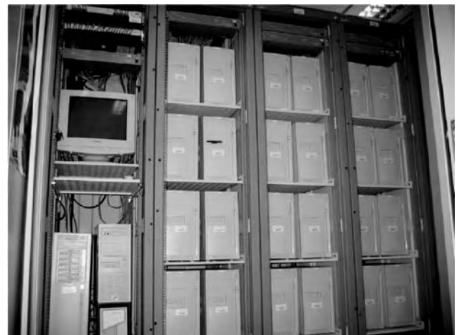
Figure 2. Fourth generation of Beowulf Linux cluster in Wireless Communications Research Center, City University of Hong Kong.
