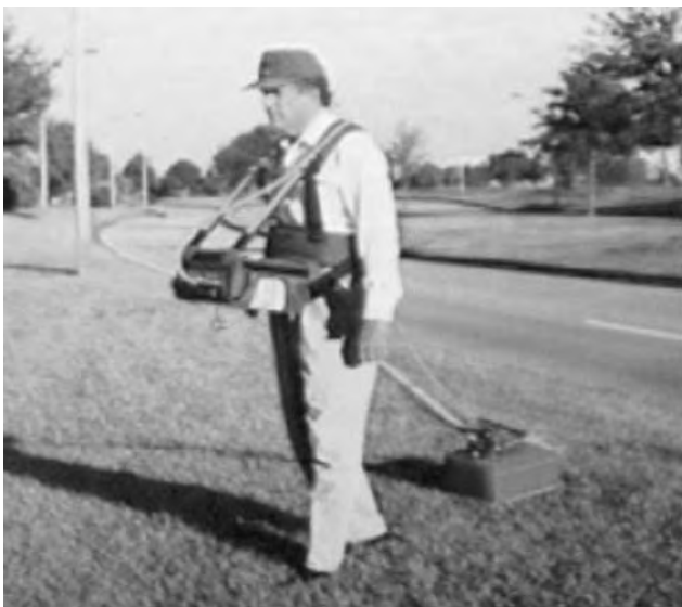
Figure 2. Shallow ground-penetrating radar surveys. (Source: http://www.geomodel.com/ )
