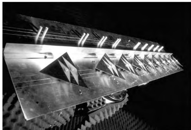
Figure 16. A dual-band microstrip array for GSM 900 and 1800 using a modified version of the Sierpinski geometry [3,4].
