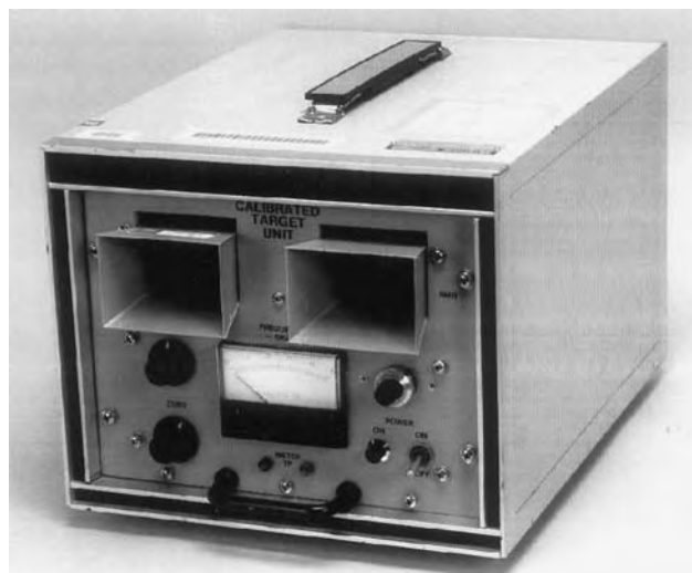
Figure 24. A K_u -band electronic moving-target simulator. One horn receives the transmitted signal, which is mixed down with one STALO and mixed back up with another matched STALO. A discriminator circuit provides a visual indication of target Doppler frequency and direction. An attenuator provides control over the radar cross section of the return signal.
