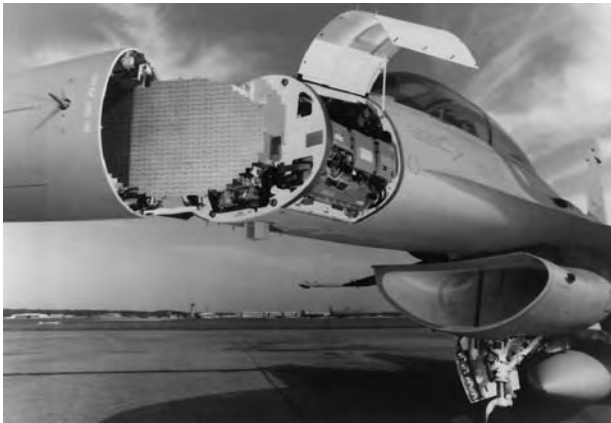
Figure 12. The electrically driven antenna of an F-16 equipped with one of Northrop Grumman's APG-66/68(V) family of coherent radars. The radar supports 25 air-to-air, air-to-ground, and mapping modes that provide target detection, acquisition, and tracking in both benign and hostile electromagnetic emissions environments. (Photo courtesy of Northrop Grumman Corporation.)
