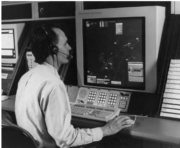
Figure 32. A modern synthetic radar display that allows overlay of map data, weather data, air traffic controller to pilot datalinks, and IFF information to generate a powerful airspace management tool. (Photo courtesy of Northrop Grumman Corporation.)
