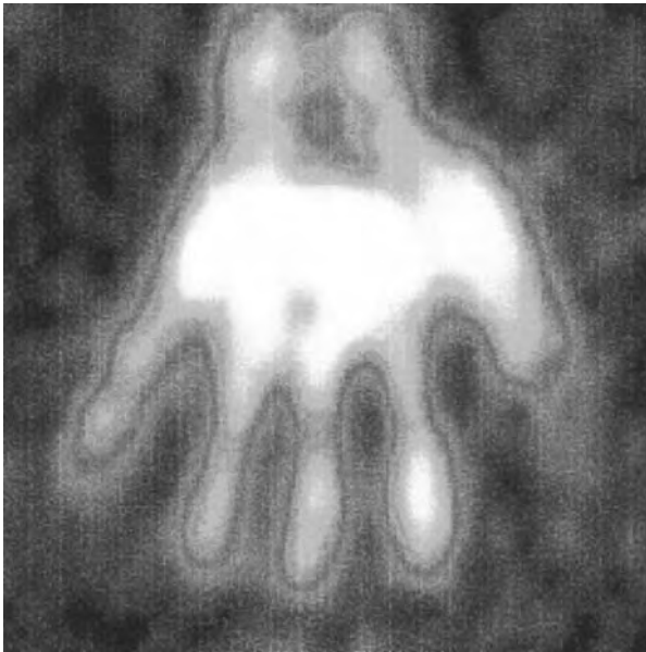
Figure 13. Microwave tomographic picture of a hand taken in the 2.45 GHz camera depicted in Fig. 7. (Courtesy of Supelec/CNRS.)
