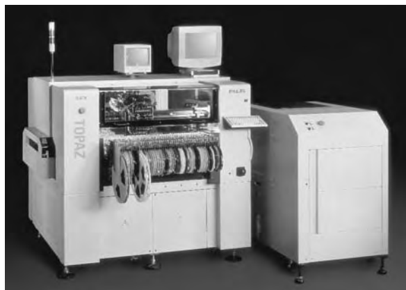
Figure 4. Example of medium-speed flexible placement machine with placement rates in excess of 14,000 devices per hour. (Figure of Philips Topaz courtesy of North American Philips.)
