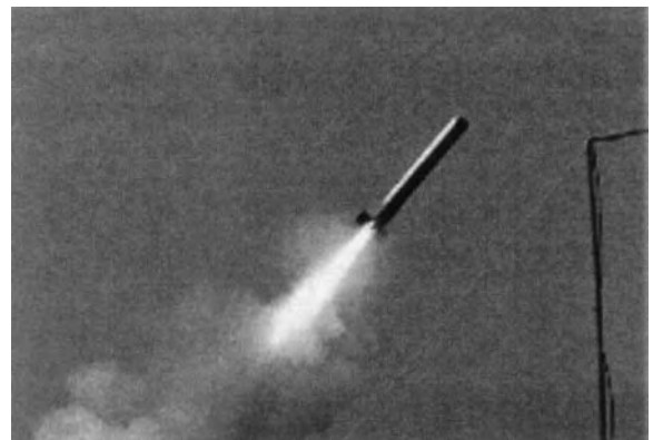
Figure 20. NATO Sea Gnat MK-216 distraction decoy deployed from a rocket launcher.
