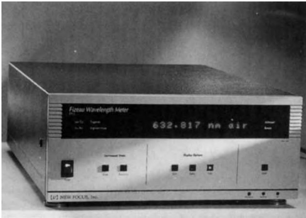
Figure 10. Front view of the New Focus Fizeau-based wavelength (courtesy of New Focus).
