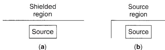
Figure 2. Examples of open shield geometries: (a) flat plate shield, (b) inverted channel shield.
