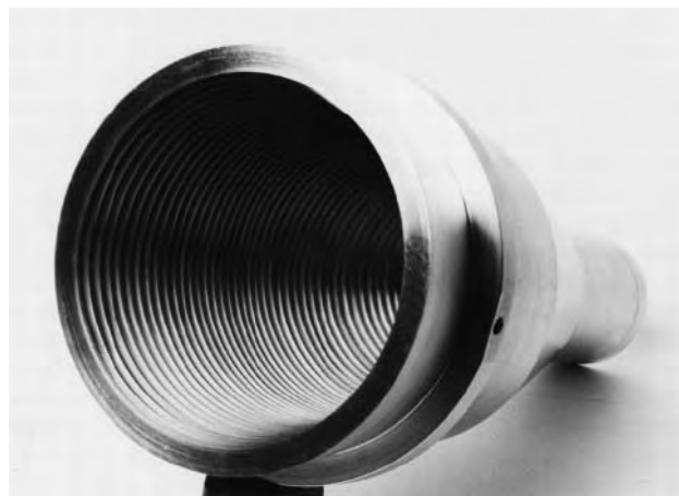
Figure 18. Dual-profile corrugated horn at 22 GHz (Courtesy of the Institute of Radioastronomy of the Italian National Research Council.)
