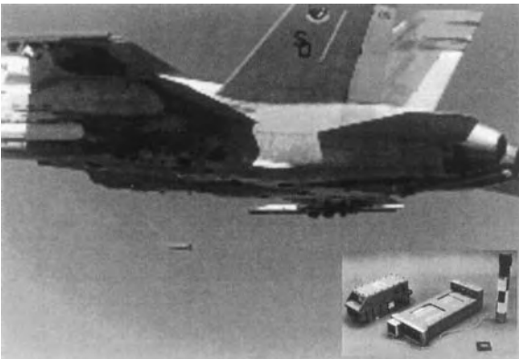
Figure 22. AN/ALE-50 towed decoy deployed from a tactical aircraft in flight.
