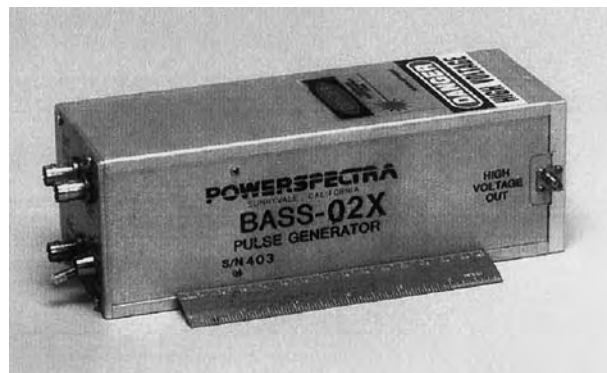
Figure 19. The PowerSpectra BASS-02X is a bulk avalanche semiconductor switch activated by a semiconductor laser. Rise-times are about 150 ps with a falltime of approximately 2 ns. Peak output power is approximately 2 MW, and average power is approximately 1.5 W. Prime power is 28 VDC, and the unit weighs approximately 2 kg. (U.S. Army photo.)
