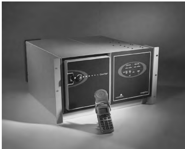
Figure 14. Rack-mountable superconducting receiver front end that incorporates superconducting filters and cooled low-noise amplifiers inside a cryogenic vacuum vessel.
