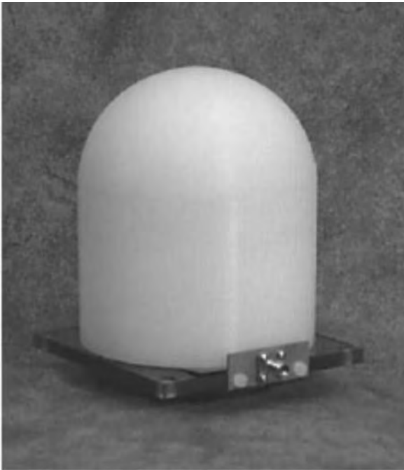
Figure 13. Photograph of a mm-wave aperture stacked patch mounted on an extended hemispherical lens.
