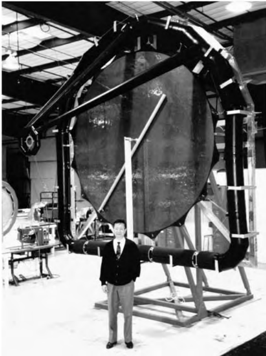
Figure 8. A 3-m Ka-band inflatable reflectarray (the shining structure in front of the aperture is the surface flatness measurement device).
