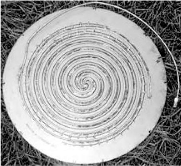
Figure 12. Two-arm slot spiral with coaxial Dyson balun feed.
