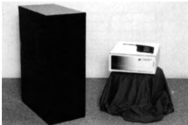
Figure 11. A comparison between a conventional dielectric resonator transceiver (left) and an HTS transceiver (right).
