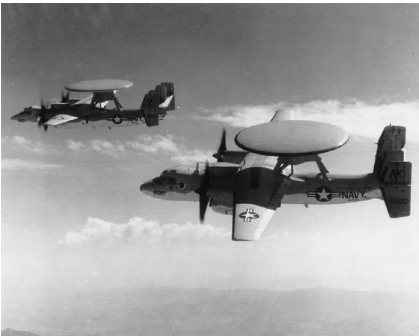
Figure 26. A pair of Northrop Grumman E-2C Hawkeyes are easily identified by their distinctive 7.3-m (24-ft)-diameter rotodomes, which contain both the low-side lobe radar antenna and the IFF antenna. A Lockheed Martin An/APS-145 radar system automatically detects, identifies, and tracks targets at ranges exceeding 300 mi. (U.S. Naval Institute collection.)
