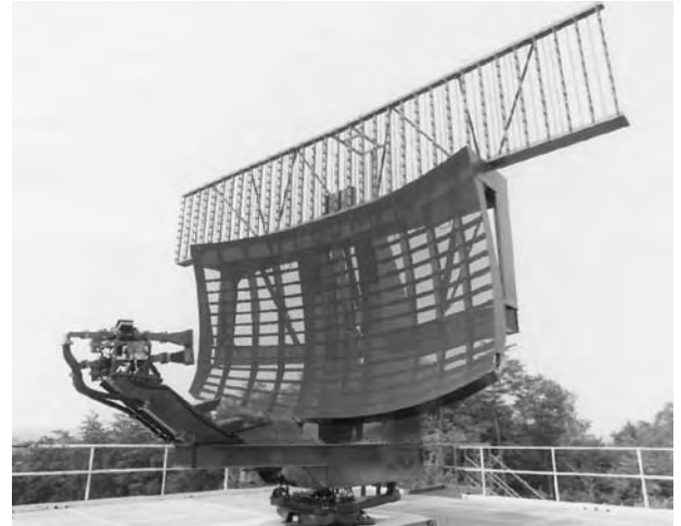
Figure 13. The Northrop Grumman ASR-12 is a modular, fully solid-state, S-band airport surveillance radar. It uses a moving-target detection scheme that combines adaptive Doppler filter and fine-scale clutter mapping to enhance the returns from tangential targets. (Photo courtesy of Northrop Grumman Corporation.)
