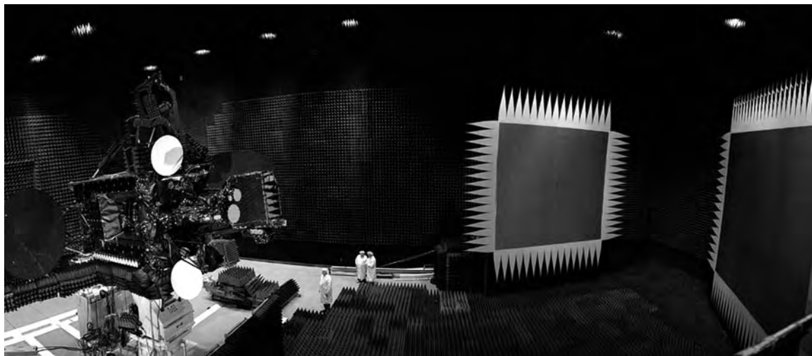
Figure 19. Intelsat-9 satellite during system tests in the compact antenna testing range (CATR), an indoor antenna measurement range that directly measures the far-field patterns of an antenna either by itself or on the satellite (courtesy of Space/Systems Loral and Intelsat).
