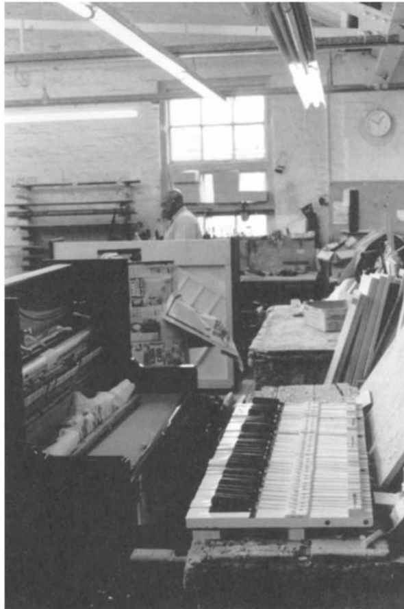
Fig. 45. A set of keys rests on the keyframe prior to being installed in an upright. Photo by Elaine Richards Hellmund. Courtesy Whelpdale, Maxwell & Codd.
