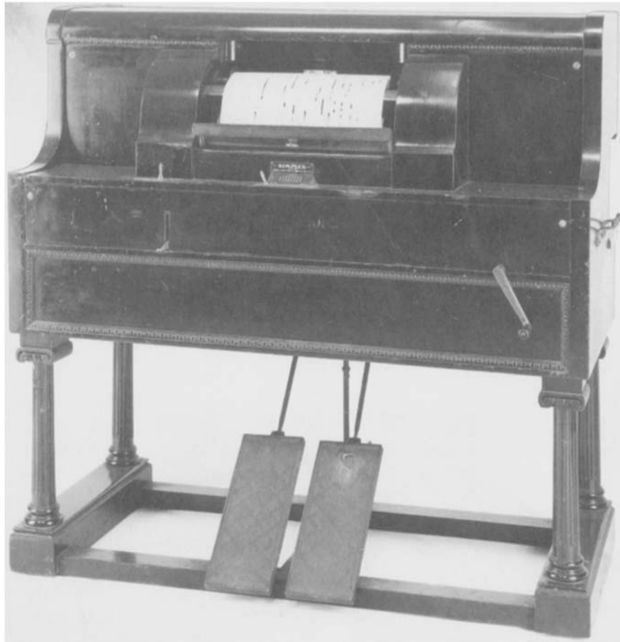
Fig. 59. Piano-players or “push-up players” were simple, yet rather bulky cabinets that were placed in front of an ordinary piano keyboard and a row of felt-covered fingers at the back of the player operated the keys. This is an early example.
