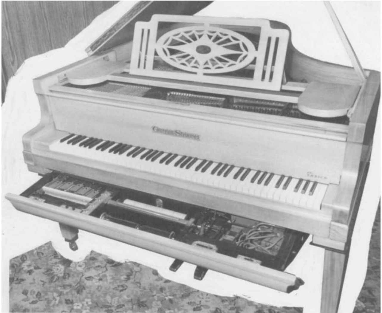
Fig. 23. One of the most successful of all reproducing pianos was the American Ampico. Electrically operated, the action was fitted into some of the finest pianos in the world. Shown here is an installation in a Grotrian-Steinweg. The player action is contained in a drawer which can be pushed back to be out of sight under the keyboard.
