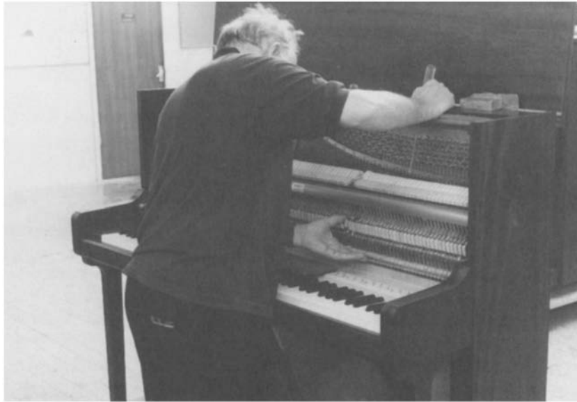
Fig. 64. A piano technician regulating the action of a nearly completed piano. Photo by Elaine Richards Hellmund. Courtesy Whelpdale, Maxwell & Codd.
