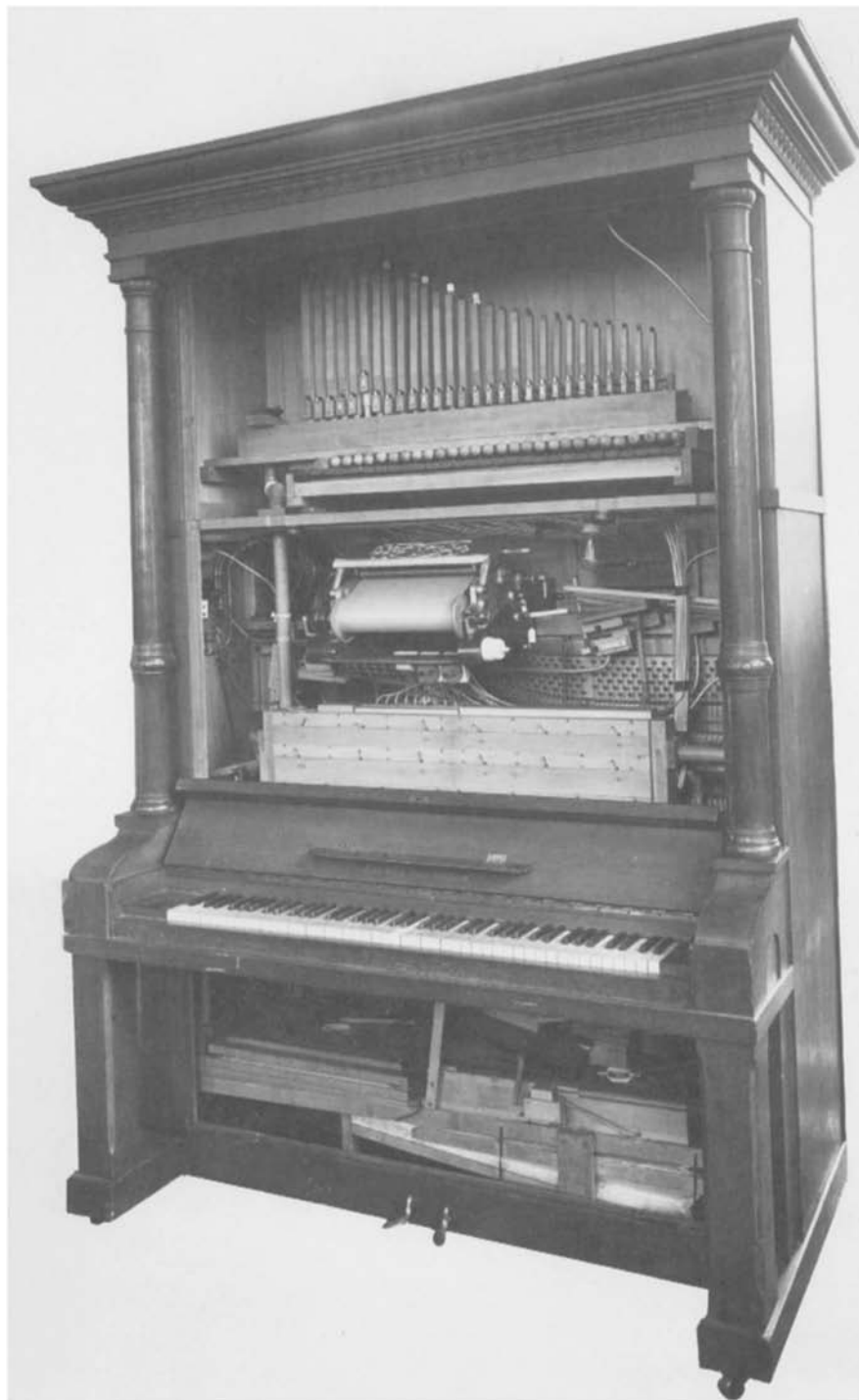
Fig. 49. Automatic pianos with orchestral effects were very popular between the beginning of the 20th century and the outbreak of the 1914–1918 war. This instrument is made by Weber in Waldkirche and comprises a fine expression piano to which is added a 28-note rank of violin-toned organ pipes.
