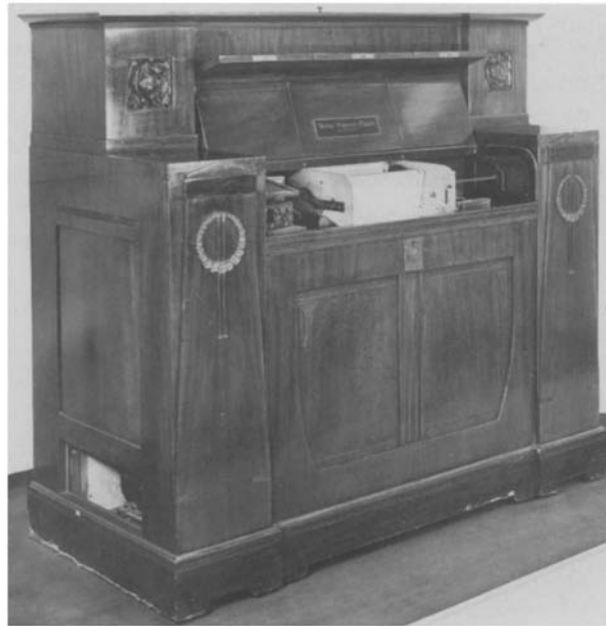
Fig. 85. Despite containing a top-quality piano, the Welte reproducing cabinet piano was merely for playing prerecorded music rolls and had no keyboard. Contained in a richly-styled cabinet that might grace any home and masquerade as an expensive sideboard, the instrument was both very expensive and a commercial disaster since it could only be played by music roll. It was replaced by models that had keyboards as well.
