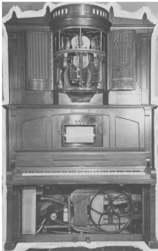
Fig. 82. Most spectacular of the pre-World War I instruments was the Hupfeld Phonoliszt Violina made in Leipzig. Built around a quality Hupfeld full-expression piano, the upper portion of the case contained three violins. Very popular in cafes and restaurants, these high-quality instruments were also very delicate and as a consequence few have survived. Electrically driven and pneumatically operated, the Phonoliszt marked the pinnacle of the great era of mechanically produced music.
