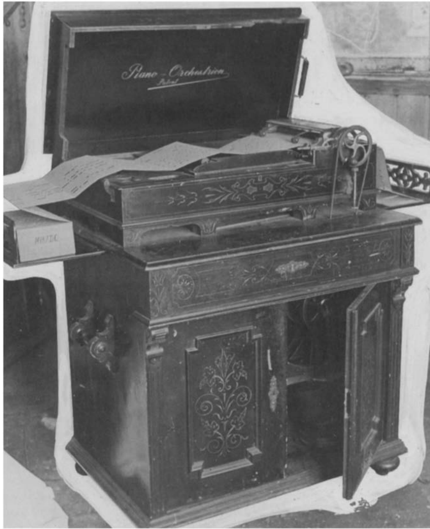
Fig. 70. Unusual amongst the mechanical pianos of the closing years of the nineteenth century was this Piano-Orchestion made in Bologna, Italy, by Giovanni Racca. Playing music by means of perforated cardboard, the reiterating mechanism produced a sound not unlike that of a mandolin or balalaika. Power to drive the mechanism came from a small hot-air engine contained in the cabinet beneath the piano.
