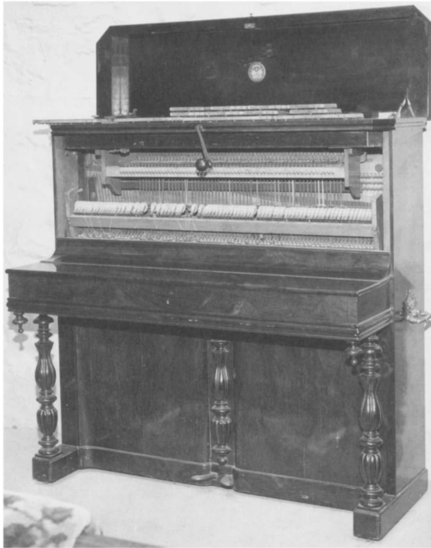
Fig. 55. Debain Piano Mécanique. In this form the fallboard is closed and the top of the piano case opened to reveal the mechanism by which the music is played automatically by the turning of the large handle. A pile of the music boards or planchettes can be seen awaiting playing. The two rows of piano hammers can be seen, those for manual playing being drawn forward to clear those being used for automatic performance.
