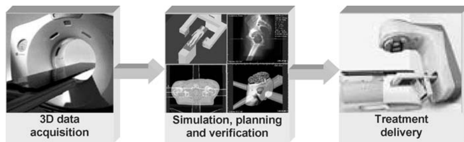
Figure 1. A schematic diagram showing the process of 3D conformal RT using a CT simulator: (a) Three-dimensional patient data acquisition through a RT dedicated CT scanner; (b) CT simulation, treatment planning and verification; (c) Treatment delivery via a LINAC.
