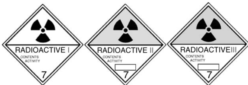
Figure 3. Labels for radioactive packages based on the activity contents and radiation levels outside as given in Table 15.
