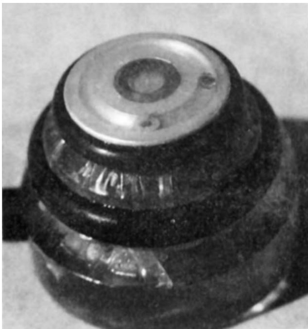
Figure 13. Photograph of combined pO_2 - pCO_2 electrode with teflon membrane (48).
