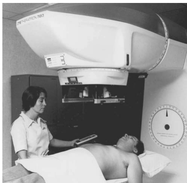
Figure 6. An isocentric mounted cobalt unit of the Theratron series produced by Atomic Energy of Canada Ltd., installed at the Ontario Cancer Institute in Toronto in the 1970s and 1980s.
