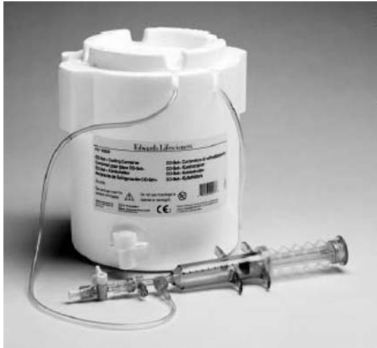
Figure 4. A closed injection system for cold injectate, by Edwards Lifesciences. A cooling coil rests in a Styrofoam ice bucket, the syringe serves as a piston pump to draw up a known volume of pre-cooled injectate from the coil and to force it into the injection lumen of the catheter. The closed system reduces the risk of nosocomial contamination associated with traditional injectate delivery methods. CO-Set+ System improves reproducibility and accuracy through its in-line temperature probe and volume-limited syringe. (Photograph courtesy of Edwards Lifesciences, Irvine, CA.)
