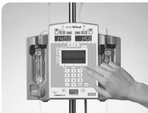
Figure 7. Signature Edition Gold infusion system by ALARIS. A range of infusion programs can be selected to save nursing time and meet sophisticated administration requirements including: Loading Dose, Multi-Dose and Multi-Step.
