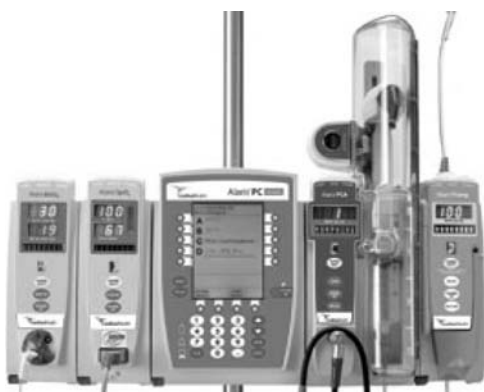
Figure 8. The Medley medication Safety System by ALARIS is a modular point-of-care computer that integrates infusion, patient monitoring and clinical best practice guidelines in a single platform for optimal outcomes.
