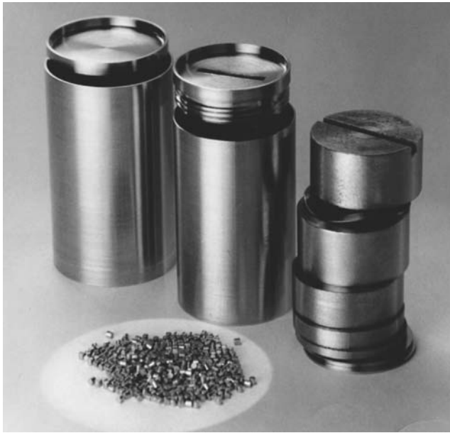
Figure 3. Cobalt pellets and source capsule with components.
