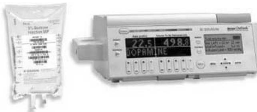
Figure 9. Outlook Safety Infusion System with DoseScan and DoseGuard by B|BRAUN technologies helping to ensure that the Right patient receives the Right medication in the Right dose from an authorized clinician at point of care.
