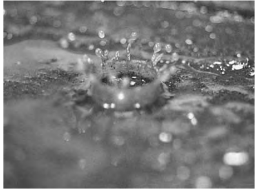
Plate 126 A simulated raindrop hitting a moist sandy surface. The kinetic energy of the impacting raindrop causes the formation of an impact crater, around which the water rebounds as a corona. The process occurs very quickly – this photograph was shot at 1:2,000 of a second
