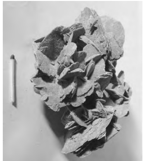
Plate 59 Example of a desert rose, the most commonly recognized form of gypsum. It forms with the evaporation of shallow ground water into a sandy substrate around a pan or sabkha margin
