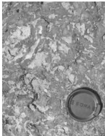
Plate 47 Indurated 'tubular' laterite sample from the top of an in situ weathering profile near Bunbury, Western Australia
