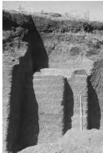
Plate 45 Laterite quarry near Bidar, south-east Deccan, India (with 1 m scale in lower right). Material beneath the indurated duricrust of a laterite profile is excavated, cut into large bricks, and allowed to harden in the sun. This is similar to the material first named 'laterite' by Buchanan (1807)
