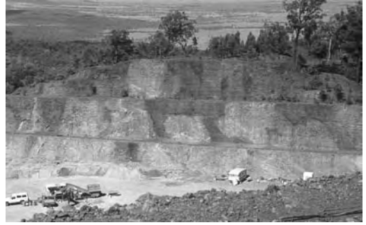
Plate 113 A very deep weathering profile formed in ultra-mafic rocks at Marlborough in central Queensland, Australia. About 40 m of the profile is exposed, but no fresh rock occurs in this pit. The total profile depth is up to about 100 m. The bulk of the material in the photo is saprolite composed of clay minerals, mainly nontronite and talc with \text{Fe}^{3+} oxides, goethite and haematite and secondary silica as chrysoprase and chalcedony. The upper part of the profile is transported debris that in places has filled karstic channels in the upper saprolite. The hill is capped by siliceous duricrust derived from silica mobilization during the weathering of the ultra-mafic rocks
