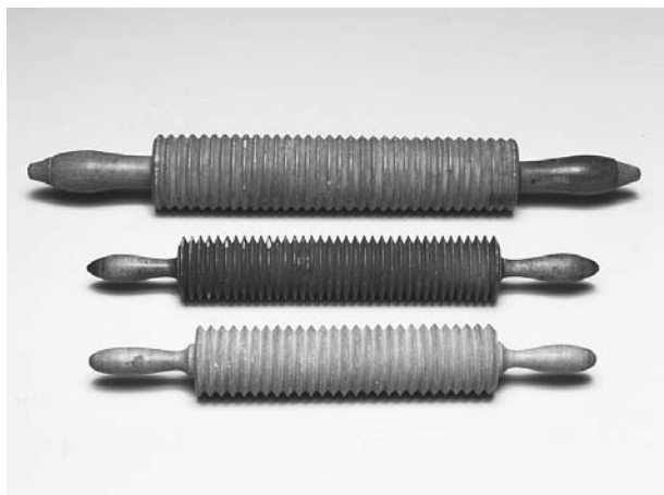
Three examples of a Nudelholz , an old tool for cutting pasta into thin strips by means of a ridged rolling pin. Made in southwest Germany, circa 1850 to 1870. This very ancient tool dating to Roman times was used in traditional culture to cut pasta or pastry into strands resembling modern linguini. ROUGHWOOD COLLECTION. PHOTO CHEW & COMPANY.
