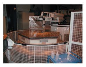
■ segmented mirror The mirror of the Gran Telescopio Canarias is made up of 36 hexagonal segments measuring 936 mm (36.85 in) on each side. The thin segments, one of which is seen here being polished, combine to form a large, flexible surface that would not be achievable with a single mirror.
