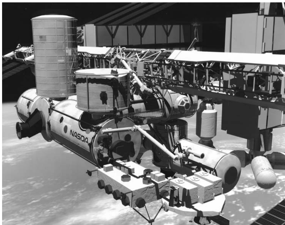
Figure 24. A view of the station showing the Japanese experiment module (JEM), complete with external payloads and remote manipulator arm. Note the windowed cupola module at center, which will be supplied by Europe. [Source: Courtesy of NASA.]
