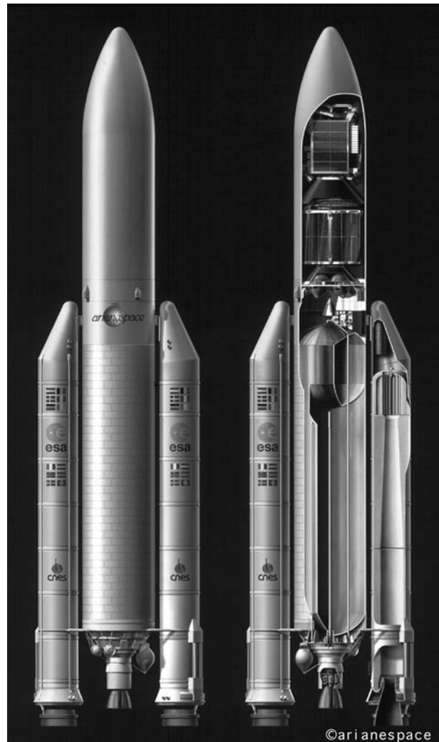
Figure 22. A cutaway of the Ariane-5 launch vehicle showing two satellites under the payload fairing and the strap-on solid propellant motors. [Reproduced with permission from ArianeSpace.]
