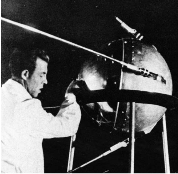
Figure 1. The Sputnik-1 satellite on a rigging truck in the assembly shop in the fall of 1957 as a technician puts finishing touches on it. [Credit: Courtesy of NASA.]
