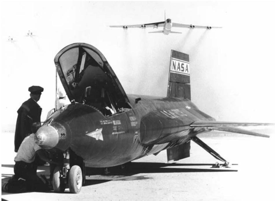
Figure 29. An X-15 rocket plane after landing. As ground support personnel begin post-flight activities, the NASA B-52 launch aircraft and two F-104 chase aircraft provide an aerial salute. (Photo courtesy of NASA.)
