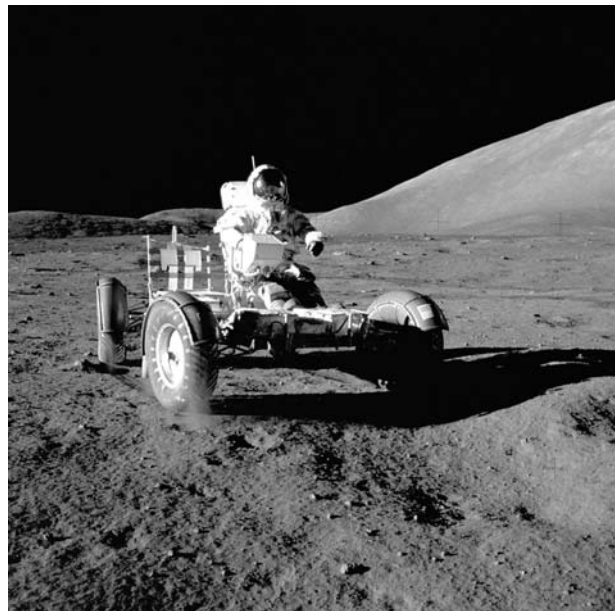
Figure 19. Astronaut Eugene A. Cernan, Apollo-17 mission commander, makes a short checkout of the lunar roving vehicle during the early part of the first Apollo-17 extravehicular activity. This view of the “stripped down” Rover is prior to load-up. The mountain in the right background is the east end of South Massif.
