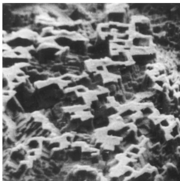
Figure 4. An early visual image (of etched aluminum surface) produced with the first Cambridge SEM; 5-second scan; angle of incidence of 16 kilovolt electrons = 25 degrees; horizontal field width = 37 micrometers.
