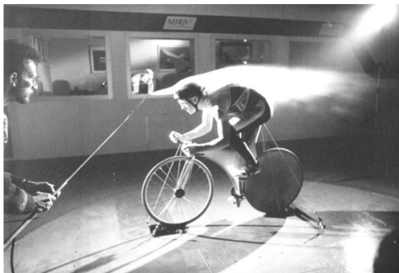
Figure 16. Wind tunnel test of the Lotus Sport Superbike ridden by Chris Boardman. [Source: QED: The Bike , BBC Education, 1993.]
