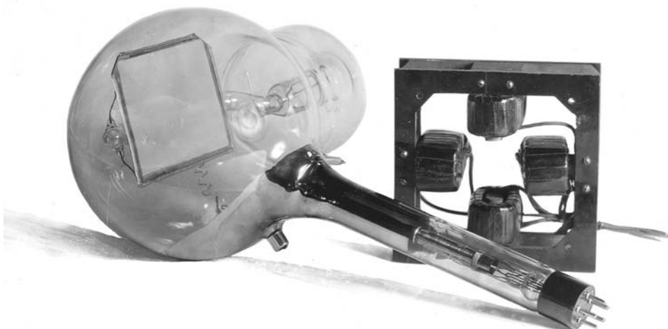
Figure 2. Iconoscope and deflecting electromagnets. [Courtesy of the David Sarnoff Library.]
