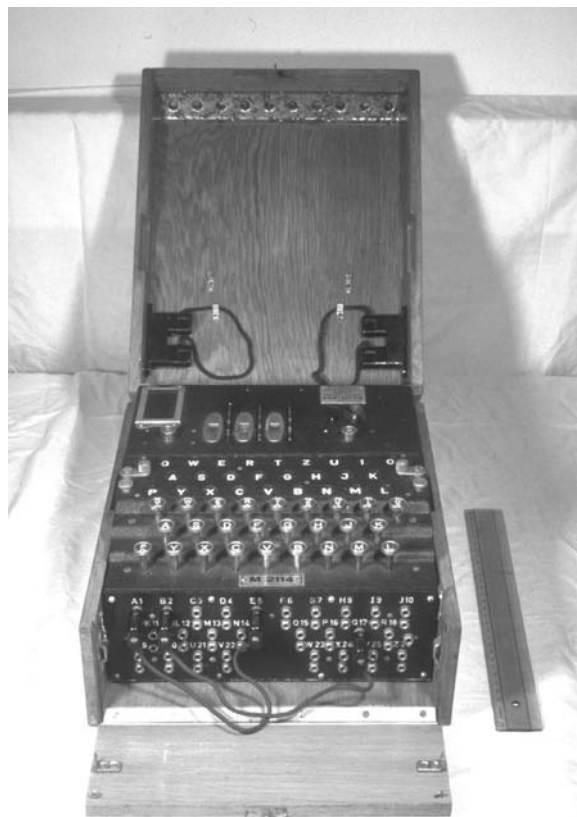
Figure 1. Marine version of an Enigma ciphering machine invented by Germany during World War II. [Courtesy of the photographer, Morton Swimmer, and the Bundesamt für Sicherheit in der Informationstechnik.]
