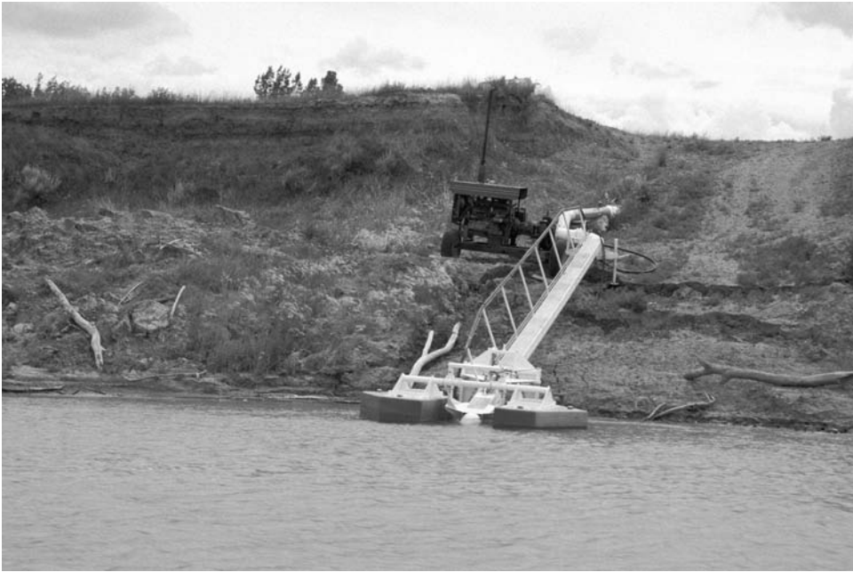
Figure 8. Because the water level of the river varies, farmers along the Missouri River use floating pumps like this one to collect irrigation water without the pump clogging. Another concern is streambank stability, which is now more manageable thanks to an online guide developed by scientists.
