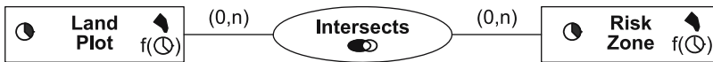
Modeling and Multiple Perceptions, Figure 11 An example of a topological relationship that links spatial object types with deforming geometries
