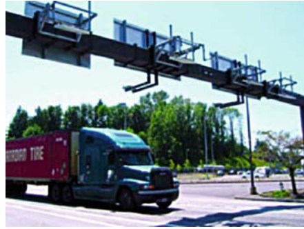
Radio Frequency Identification (RFID), Figure 6 Truck transponder sends data to roadside RFID reader via overhead antennae. (Source: FHWA)
