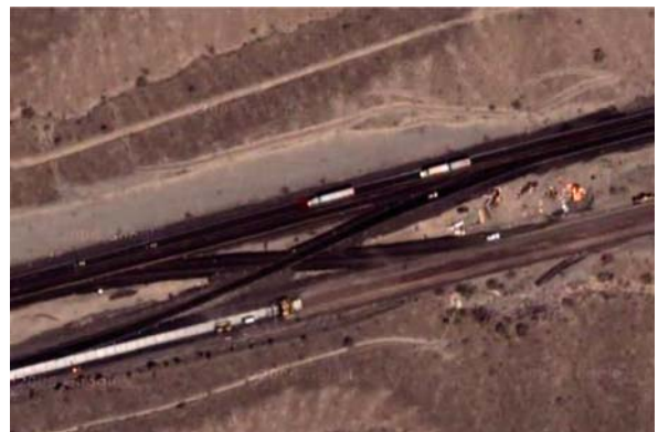
Contraflow in Transportation Network, Figure 9 Use of contraflow for highway construction on I-10 in Arizona (source: map.google.com)
