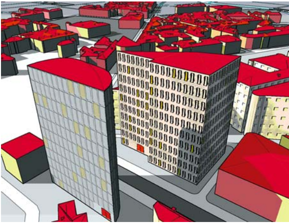
Visualization, Photorealistic and Non-photorealistic, Figure 6 Example of a non-photorealistic depiction of a virtual 3D city model based on real-time rendering techniques for image-space edge enhancement, shadowing, and n-tone shading
