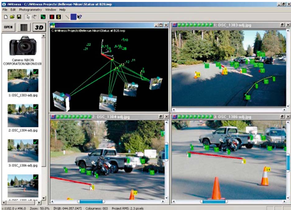
Photogrammetric Applications, Figure 6 Accident scene recording and photogrammetric processing (Photomatrix)
