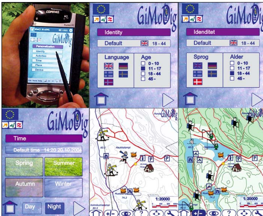
User Interfaces and Adaptive Maps, Figure 5 The GiMoDig service delivers adaptive maps in real-time to the mobile devices
