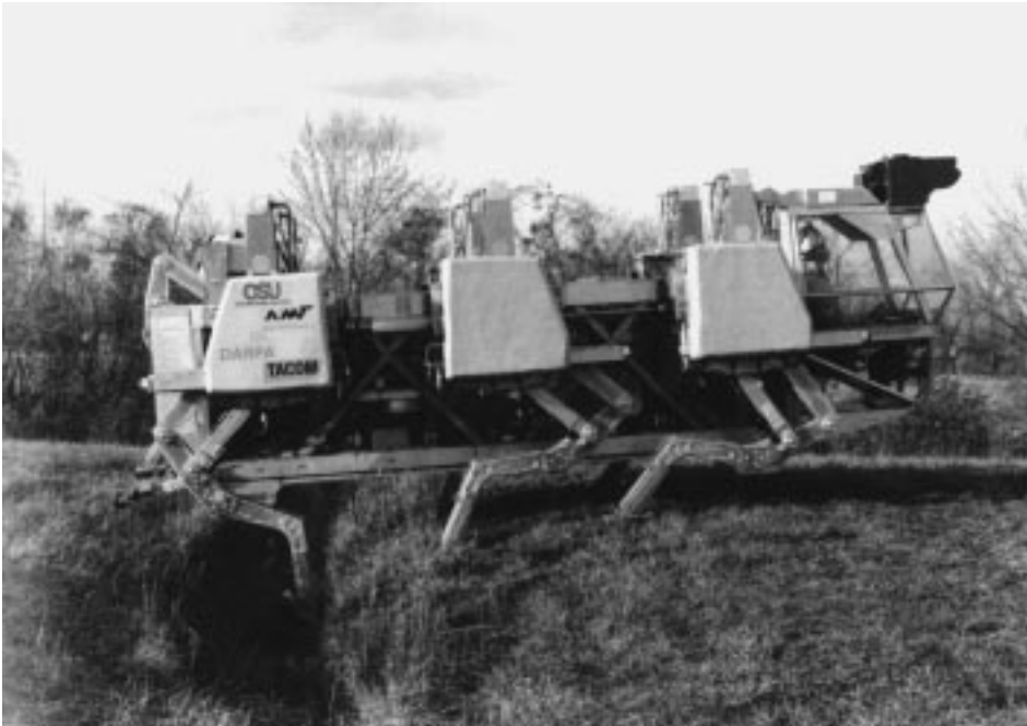
Figure 1. The Adaptive Suspension Vehicle crossing uneven terrain. Photograph reprinted by permission of The Ohio State University.
