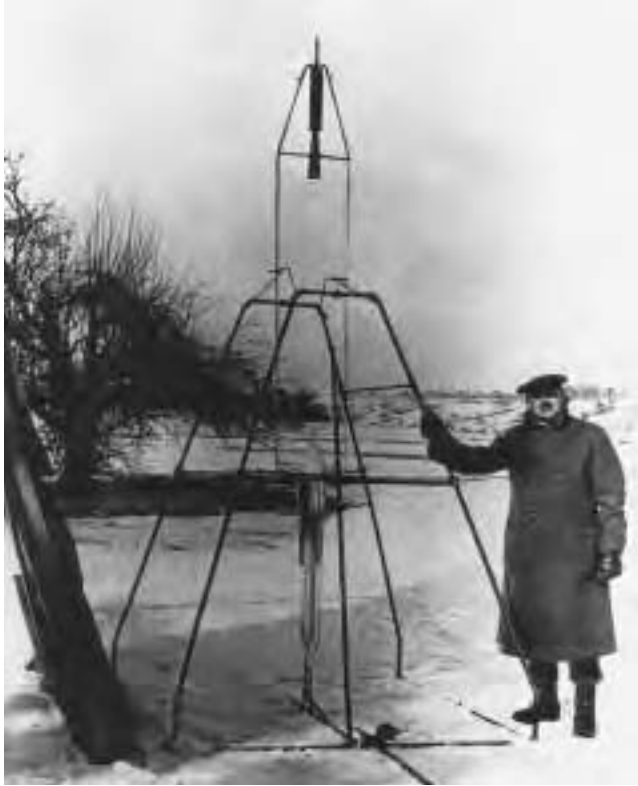
Robert H. Goddard and the liquid-oxygen–gasoline rocket in the launch frame from which he fired it on March 16, 1926, in a snow-covered field at Auburn, Massachusetts. The event represents the birth of the liquid-propellant rocket. (Courtesy of NASA)
