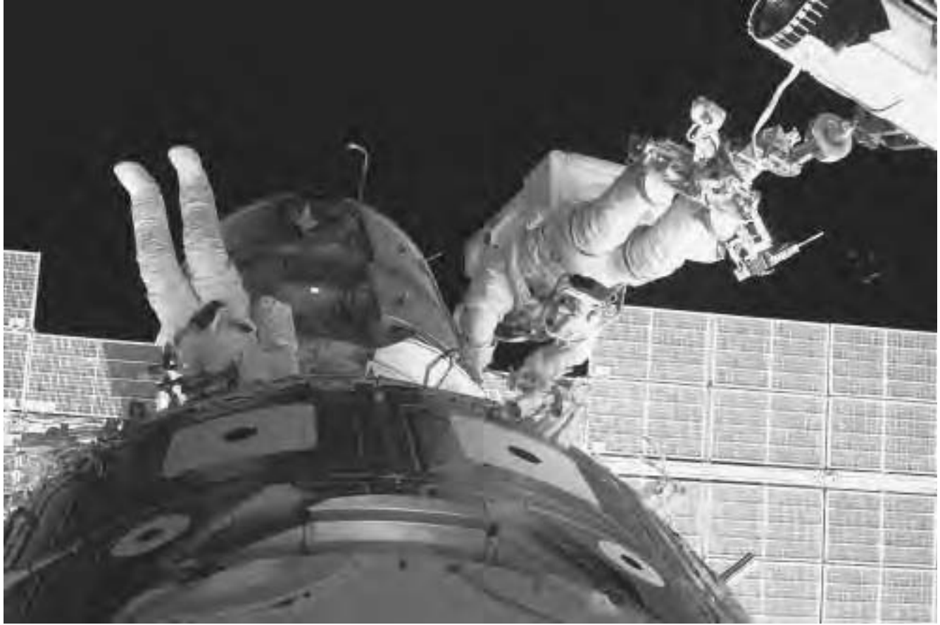
In December 1998 the space shuttle Endeavour supported the first on-orbit assembly mission of the International Space Station (ISS). As shown here, NASA astronauts James H. Newman (left) and Jerry L. Ross (right) worked between the Zarya and Unity (foreground) modules of the ISS during an extravehicular activity conducted as part of the STS-88 mission. Newman was tethered to the Unity module, while Ross was anchored at the feet to a mobile foot restraint device, which was mounted to the end of the shuttle's robot arm (called the remote manipulator system, or RMS). (Courtesy of NASA/JSC)
