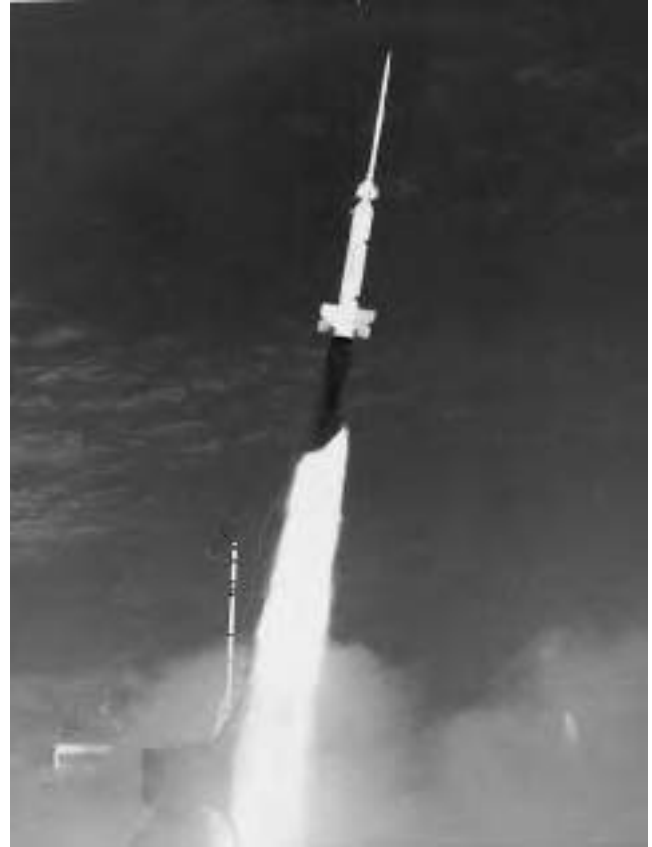
A Nike-Apache sounding rocket blasts off from NASA's Wallops Flight Facility, Wallops Island, Virginia, in 1965. In its seven-minute, ballistic trajectory flight over the Atlantic Ocean, this rocket's scientific payload, designed to make measurements within the ionosphere, reached a maximum altitude of approximately 180 kilometers. (Courtesy of NASA)
