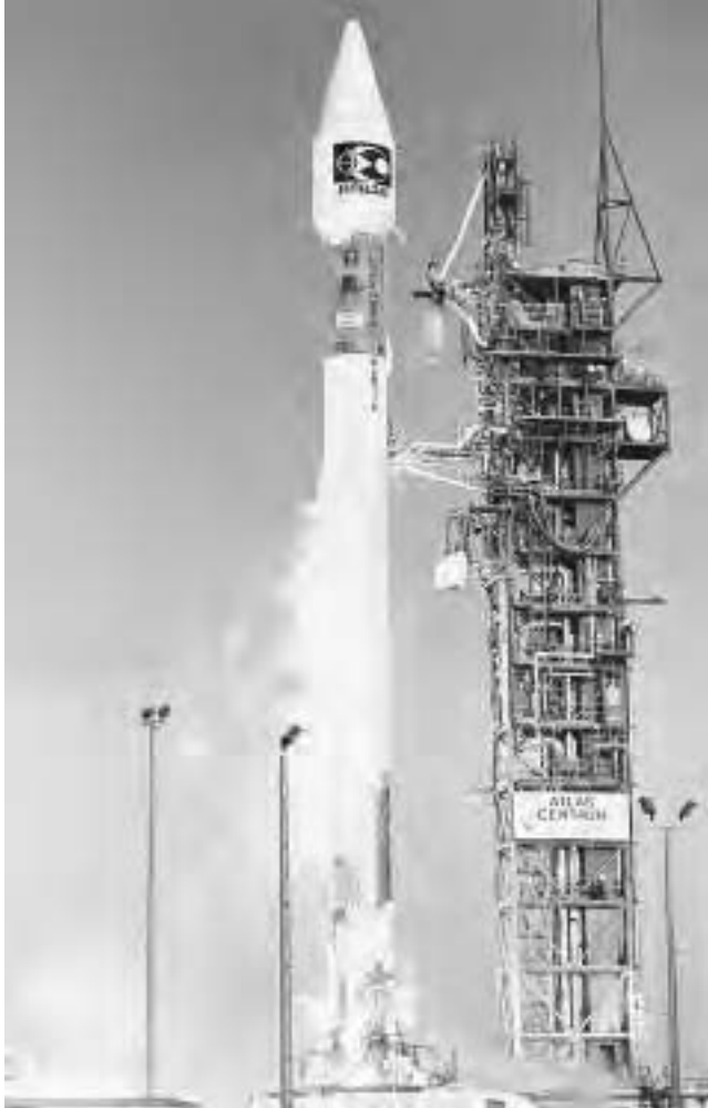
The Atlas III expendable launch vehicle made its debut at Cape Canaveral Air Force Station in Florida on May 24, 2000. The rocket's successful liftoff was powered by a new Russian RD-180 engine. (Courtesy of U.S. Air Force and Lockheed-Martin)
