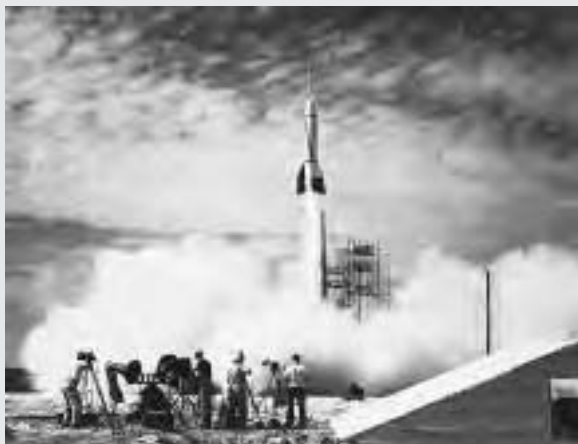
The first rocket launch from Cape Canaveral took place on July 24, 1950. The Bumper 8 rocket, shown here lifting off, was a modified German V-2 rocket with a WAC Corporal second stage. (Courtesy of the U.S. Air Force)
