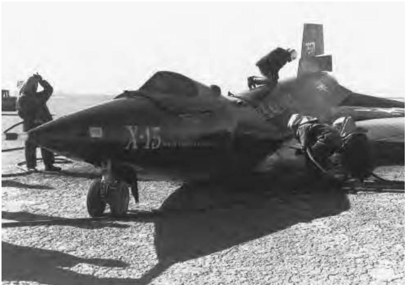
Emergency crew personnel examine a crumpled NASA X-15 rocket plane after a hard landing on the dry lakebed at Edwards Air Force Base in California in 1963. The pilot, Scott Crossfield, survived the rough landing, but the X-15 rocket plane suffered a broken airframe. (Courtesy of NASA/Dryden Flight Research Center)
