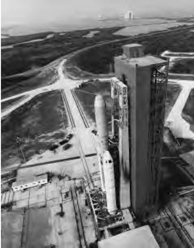
A Titan 34D space launch vehicle is shown ready for launch from Complex 40 at Cape Canaveral AFS, Florida (ca. 1982). Other portions of the U.S. Air Force's Integrated Transfer Launch Facility (ITLF) appear in the background. (Courtesy of the U.S. Air Force and Lockheed-Martin Company)
