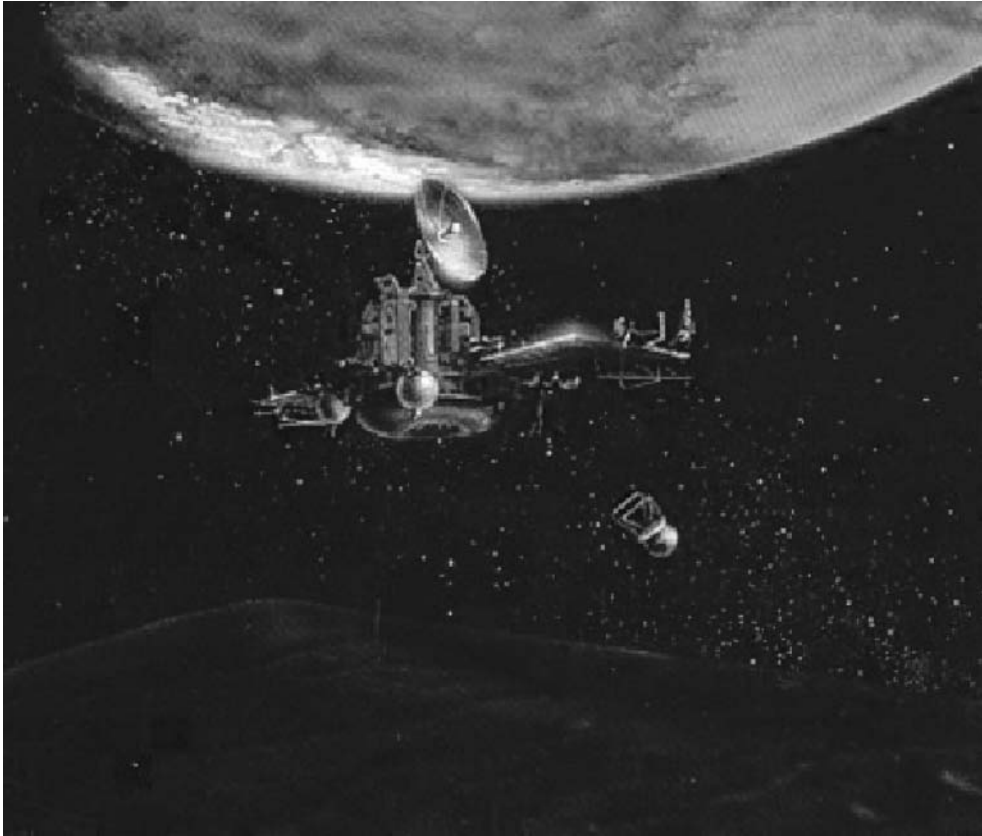
Figure 9. This artist's concept depicts the Phobos 1 & 2 spacecraft destined for Mars. They were the next-generation in the Venera-type planetary missions, succeeding those last used during the Vega 1 and 2 missions to comet P/Halley. (Courtesy of NASA's National Space Science Data Center.) This figure is available in full color at http://www.mrw.interscience.wiley.com/esst .
