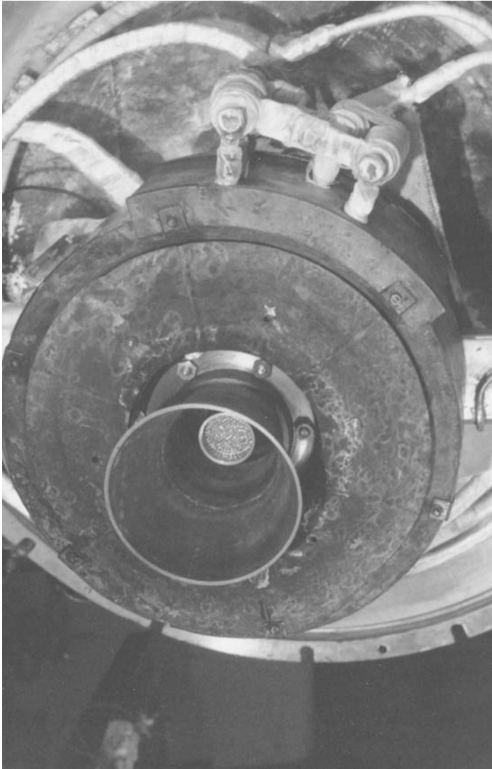
Figure 18. Photograph of a MPDT with power of up to 200 kW. The anode diameter at the end is 160 mm. This figure is available in full color at http://www.mrw.interscience.wiley.com/esst .
