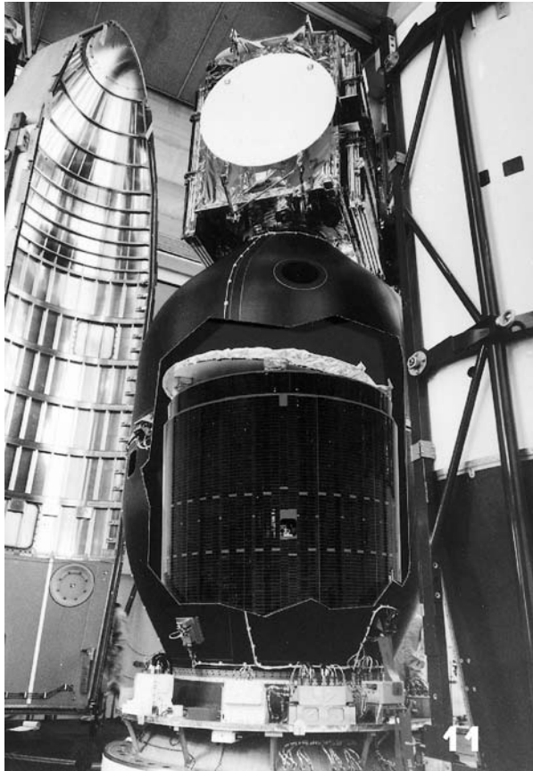
Figure 4. SYLDA, Ariane dual-launch system. This figure is available in full color at http://www.mrw.interscience.wiley.com/esst .
