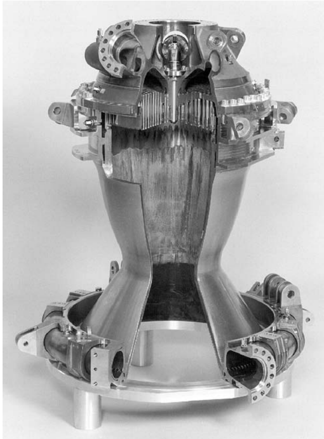
Figure 11. Photo of regeneratively cooled thrust chamber (Vulcain). This figure is available in full color at http://www.mrw.interscience.wiley.com/esst .
