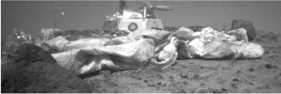
Figure 10. Rover view of the lander on the surface of Mars. Notice how far the airbags retracted. (Image courtesy of JPL/NASA.)
