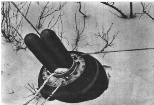
Figure 2. Returned capsule of Luna 20 with lunar samples inside landed in snows of Western Siberia. The two extended features in the top part of the capsule are inflated antennae sending signals to the recovery teams.
