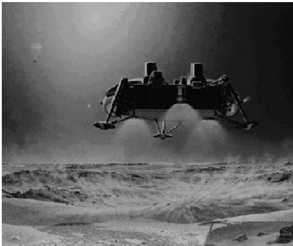
Figure 8. Captured in this rendering is a Viking lander just before it touched down on the Martian surface. The parachute and upper aeroshell can be seen in the upper left corner of the image. At this stage of the descent, the lander's terminal descent propulsion system (three retro-engines) had slowed the craft down so that velocity at landing was about 7 miles per hour (2 meters per second). Seconds after the lander reached the surface it began transmitting images back to the orbiter for relay to Earth. (Courtesy NASA/JPL.) This figure is available in full color at http://www.mrw.interscience.wiley.com/esst .
