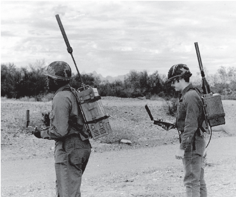
Figure 8. The original GPS “Manpack” cost more than $50,000 each and was quite heavy. It did, however, satisfy the original mandate to produce an inexpensive device that could navigate. Modern-day receivers are much smaller and much less expensive. Today, one can buy both a watch and a cell-phone that has GPS built in. An inexpensive GPS receiver can be purchased for less than $100. This figure is available in full color at http://www.mrw.interscience.wiley.com/esst .
