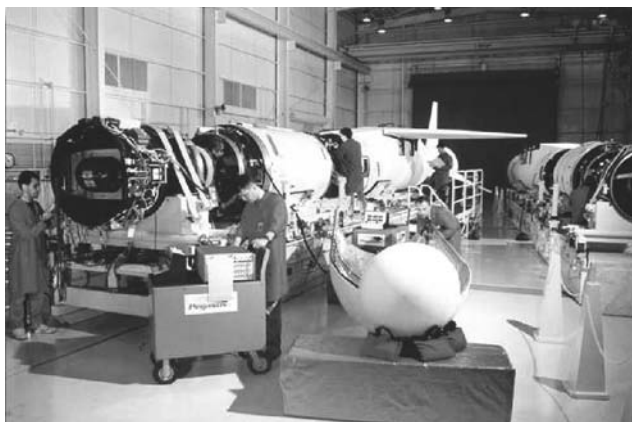
Figure 3. Horizontal integration of Pegasus launch vehicle. This figure is available in full color at http://www.mrw.interscience.wiley.com/esst .
