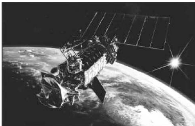
Figure 5. The Defense Meteorological Satellite Program (DMSP) has been collecting weather data for U.S. military operations for almost four decades. At all times, two operational DMSP satellites are in polar orbit at about 458 nautical miles (nominal). The primary weather sensor on DMSP is the Operational Linescan System which provides continuous visual and infrared imagery of cloud cover over an area 1600 nautical miles wide. Figure courtesy USAF Space Command. Picture can be found at http://www.peterson.af.mil/hqafspc/Library/FactSheets/FactSheets.asp?FactChoice=4 . This figure is available in full color at http://www.mrw.interscience.wiley.com/esst .
