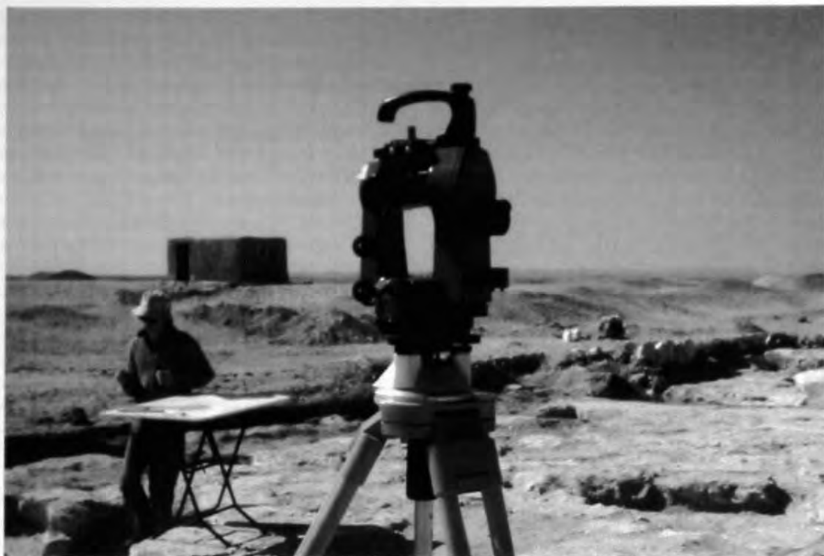
ARCHAEOLOGY. Careful recording necessitates measurements. A theodolite, a surveying instrument, measures vertical and horizontal angles, as used at the excavations of Dieter Arnold in el-Lisht, 1989. (Courtesy Dieter Arnold)
