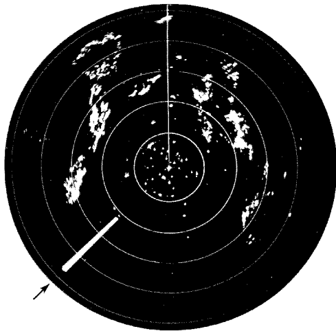
Figure D55 PPI display for maritime radar, with range rings 5 nmi apart (from Skolnik, 1970, p. 31.33, reprinted by permission of McGraw-Hill).
