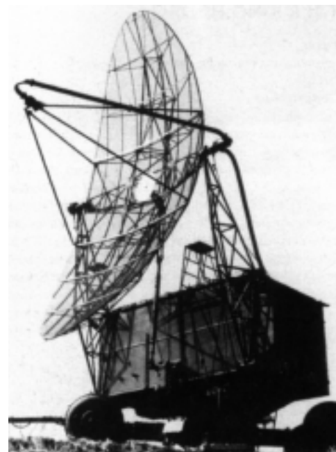
Figure H1 A Russian S-band nodding height-finder radar (from Jane's Radar and Electronic Warfare Systems , 1993-94).
