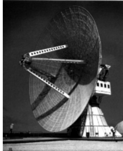
Figure R36 Tradex reentry instrumentation radar.
