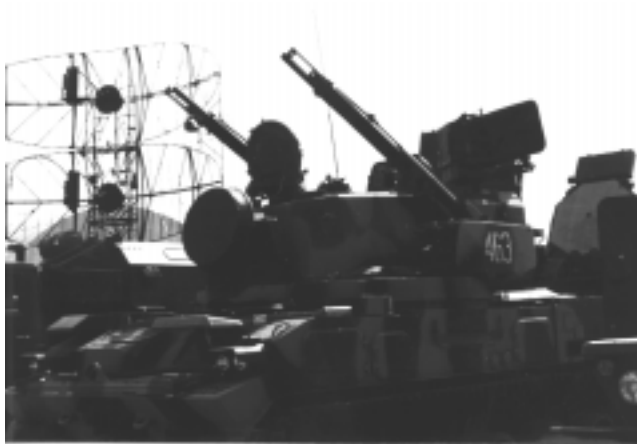
Figure R21 Russian anti-aircraft gun and missile system, using S-band search and K_u -band fire control radar.
