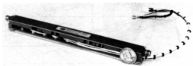
Figure P9 Combined coaxial-line-waveguide phase shifter (from Skolnik, 1970, Fig. 23, p. 12.25, reprinted by permission of McGraw-Hill).
