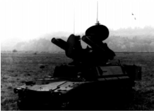
Figure R20 Roland short-range missile system, using monopulse tracking and guidance radar.
