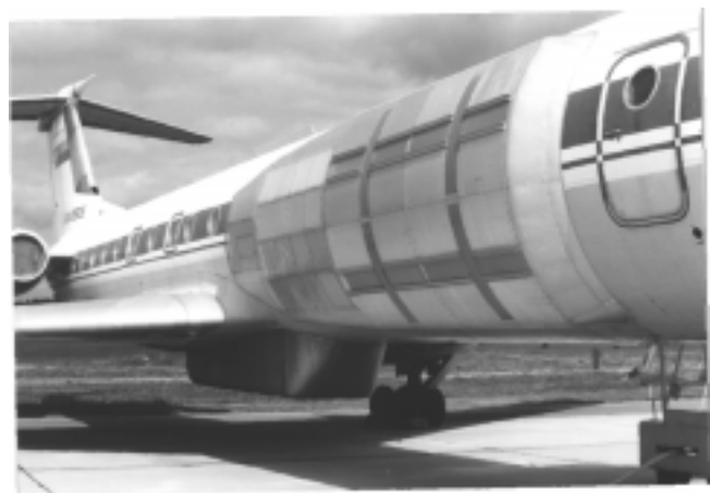
Figure R28 Multifrequency airborne earth resources remote sensing radar, at 1993 Moscow air show.
