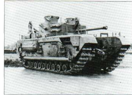
The Churchill AVRE Mark II featured a fixed turret mounting a dummy gun. It could carry a front-mounted dismountable jib crane or a rear jib with a higher lift capacity. There was also a powerful front-mounted winch that could be used in conjunction with the jibs, and an earth anchor was mounted at the rear.
