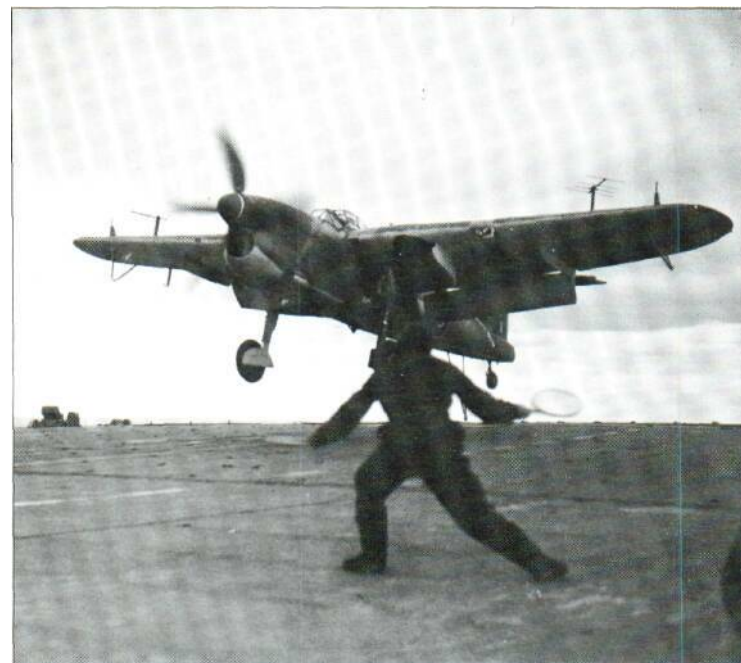
Fairey Barracuda Mk II of the Fleet Air Arm, complete with anti-submarine radar and underwing depth bombs.
