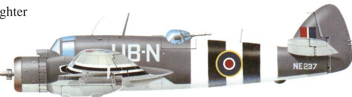
Bristol Beaufighter TF.MkX of No. 455 Sqn armed with eight underwing, unguided rockets.
