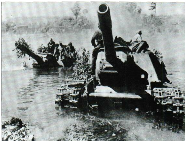
An ISU-152 crosses a river during the latter stages of World War II. These vehicles appear to be carrying their crewmembers on the roof, but in action they would be carrying squads of 'tank descent' assault infantry instead. Note the size of the howitzer's muzzle brake.
