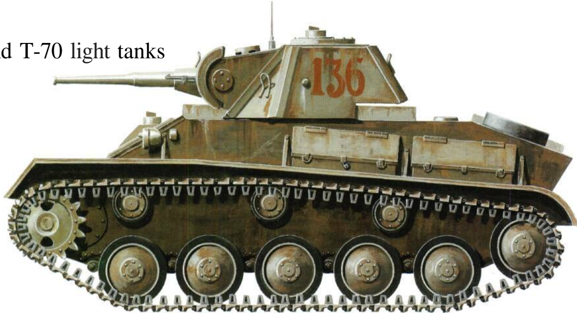
Above: The T-70 light tank was a useful reconnaissance vehicle, but it had only a 45-mm (1.77-in) main gun and was thus of little use in combat against heavier German tanks. In action it proved to be adequate but unexceptional.
