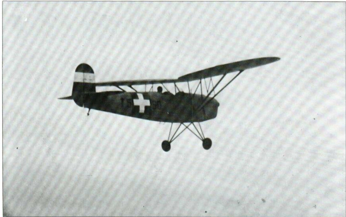
The Levante II was used on the Eastern Front as a communications and liaison aircraft by the Hungarian air force. It was powered by a licence-built Hirth 4-cylinder engine, giving a maximum speed of 180 km/h (112 mph).
