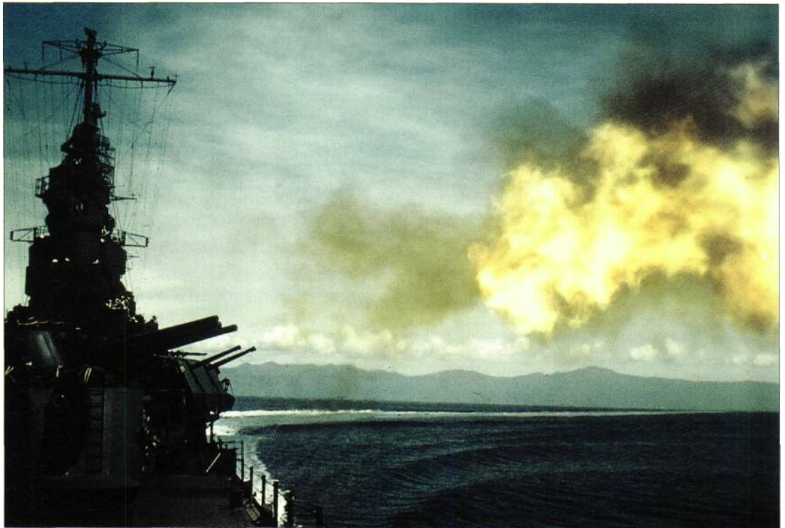
USS Biloxi of the Cleveland class firing her 152.4mm (5in) guns, of which she had 12 in four triple turrets. Twenty-six Cleveland class entered service during the war.
