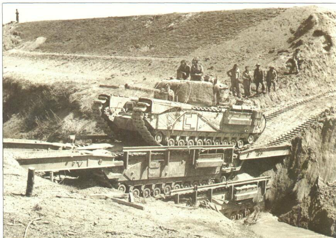
Two ARK Mk IIs are used to allow other vehicles to cross a deep ravine. The first ARK was driven into the ravine and the second ARK was then driven onto it, after which its ramps were lowered to form a bridge. The ravine was formed by the River Senio in Italy, April 1945.
