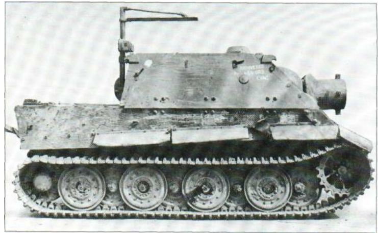
Above: This side shot of a Sturm-tiger shows the large armoured superstructure, mounting the 38-cm (14.96-in) rocket projector with the roof-mounted crane needed to load the projectiles in to the interior through a hatch at the rear.
