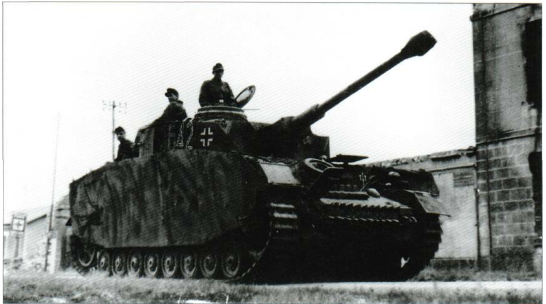
A German PzKpfw IV tank being held in reserve in anticipation of a call to action following the Allied landings at Normandy in June 1944. Note the side skirt.
