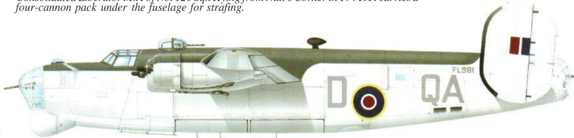
Liberator CRMkV of No. 224 Sqn in November 1942. This was the RAF version of the B-24C, and introduced greater range and armament over its predecessor.
