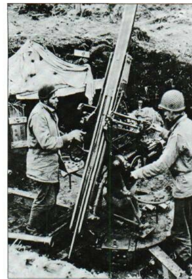
Above: The mount of a captured Type 88 75-mm gun is examined in the Pacific. Notice the five legs of the firing platform and the detached barrel at the bottom left of the photograph.
