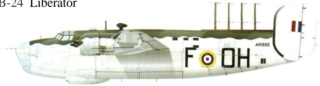
Consolidated Liberator Mk I of No. 120 Sqn flying from Nutt's Corner in 1941. It carries a four-cannon pack under the fuselage for strafing.
