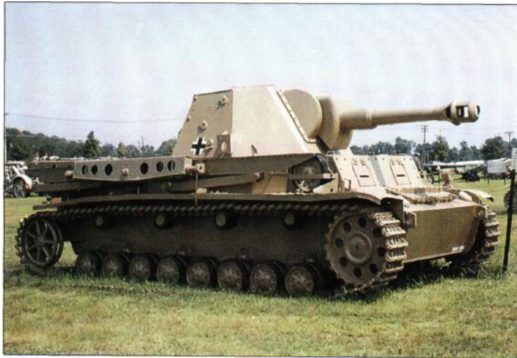
The Heuschrecke was one of a number of experimental German vehicles that were meant to carry an artillery piece to a firing site and then
