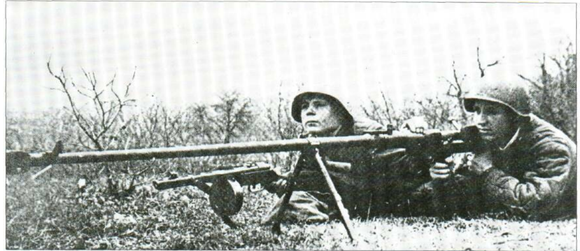
The Soviet 14.5-mm (0.57-in) PTRD 1941 anti-tank rifle has had a round loaded into the breech with the loader's left hand; a subsequent tap on the firer's helmet would then indicate that the rifle is ready to fire.
