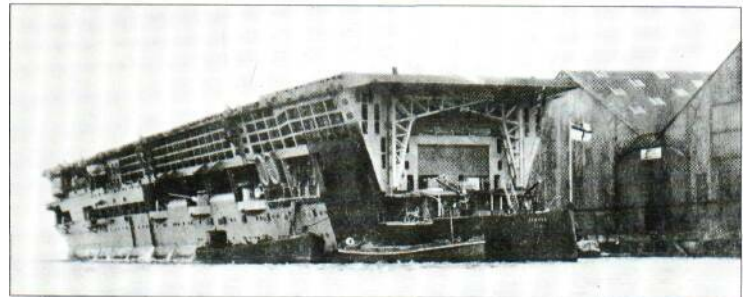
Right: HMS Furious in April 1927. The superstructure was removed in 1921 as it created serious turbulence problems. Further alterations took place in the 1930s, cross-deck arrester gear was fitted and the AA gun arrangement changed.
