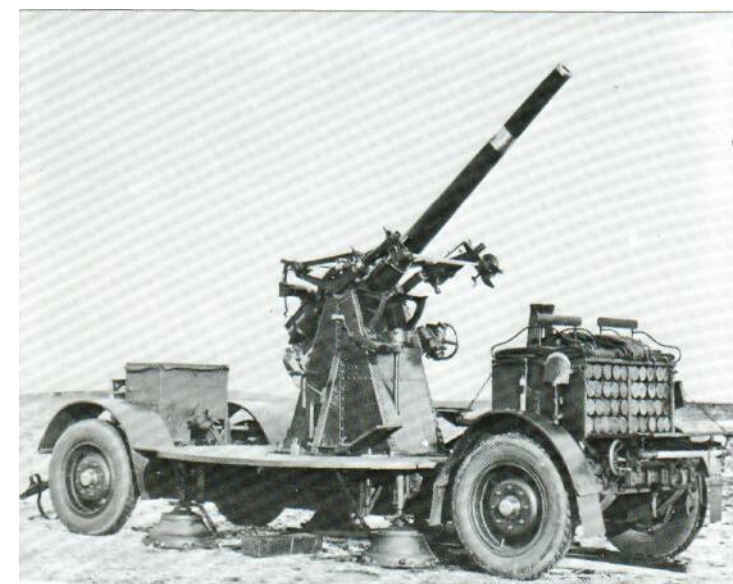
The usual model of the 3-in (76.2-mm) gun in use with the BEF in 1940 was this platform version, complete with twin axles. The platform used
