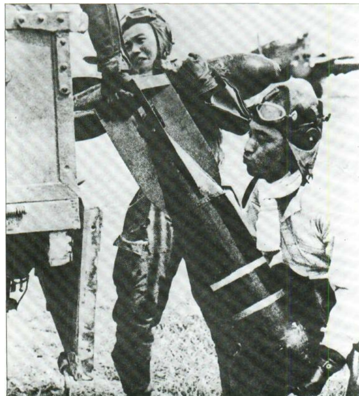
The Type 97 no. 6 59-kg bomb was a general-purpose weapon carried by a variety of Japanese aircraft, from heavy bombers to fighters.
