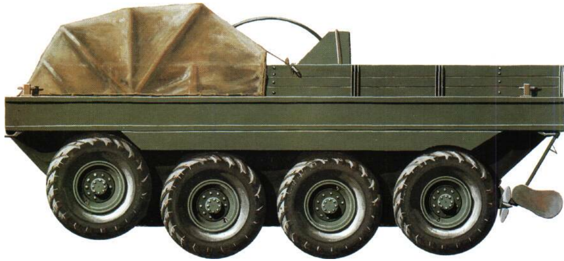
The Terrapin was powered by two Ford V-8 petrol engines and was driven in the water by two propellers at the rear. There were two cargo holds and the driver sat in the centre of the vehicle.
