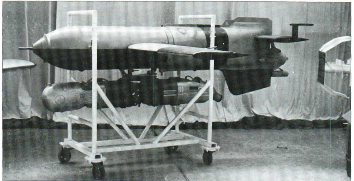
The Henschel Hs 293A stand-off guided bomb was dropped from the carrier aircraft on a parallel course to the target on the port side, and radio-guided to the target. A flare in the rear of the bomb gave visible evidence of the missile's position to the aimer.
