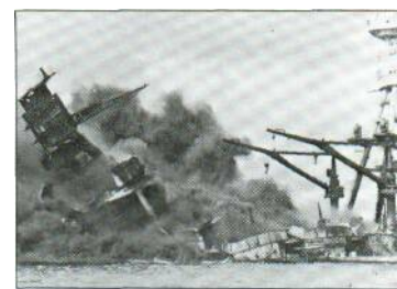
The Arizona's tripod masts sags slowly to port after the detonation of the forward 356-mm (14-in) magazine had wrecked the ship.
