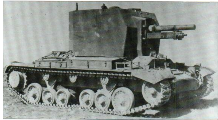
Above: This Bishop in 'factory's state clearly shows the high and bulky outline of the fixed turret mounting the 25-pdr gun. As this was a 'first
