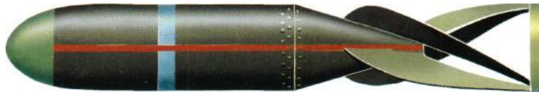
Above: The Type 99 no. 80 750-kg GP bomb was one of the largest bombs regularly employed by the Japanese.
