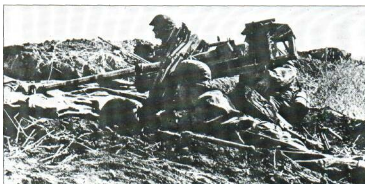
Above: The 2.8-cm schwere Panzerbüchse 41 was the smallest of the German taper-bore guns, and was produced in two forms: one had large road wheels while a special airborne version, shown here, had small wheels and a light tubular alloy carriage. In this form it was used by Luftwaffe Fallschirmjäger units.
