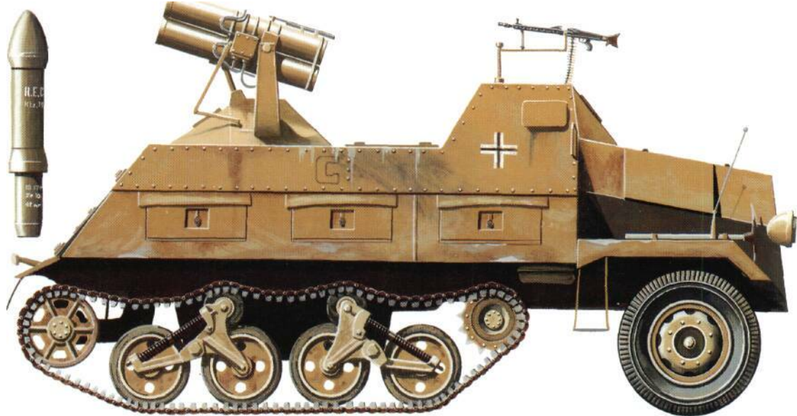
Above: The 15-cm Panzerwerfer 42 was not only more mobile, but more survivable; rockets betrayed their position the moment they fired, so to avoid enemy artillery fire they needed to change position rapidly.
