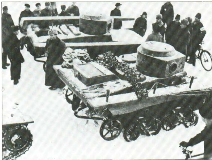
Disabled T-37 light amphibious tanks are seen in the snow of the Winter War against the Finns in 1939-1940. In this campaign the T-37s showed up badly, as they had only light armour. The front vehicle is a T-37(TU) command tank with the remains of an aerial showing.
