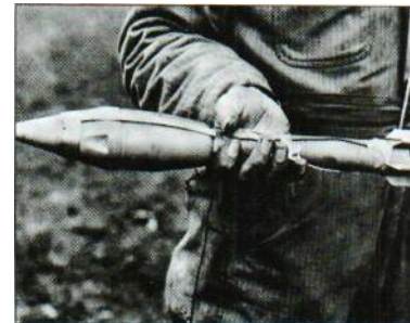
Above: The rocket fired from the American bazookas was fin-stabilized and weighed 1.53 kg (3.4 lb). It had a maximum range of 640 m (700 yards), but was accurate only to ranges much shorter than that.
