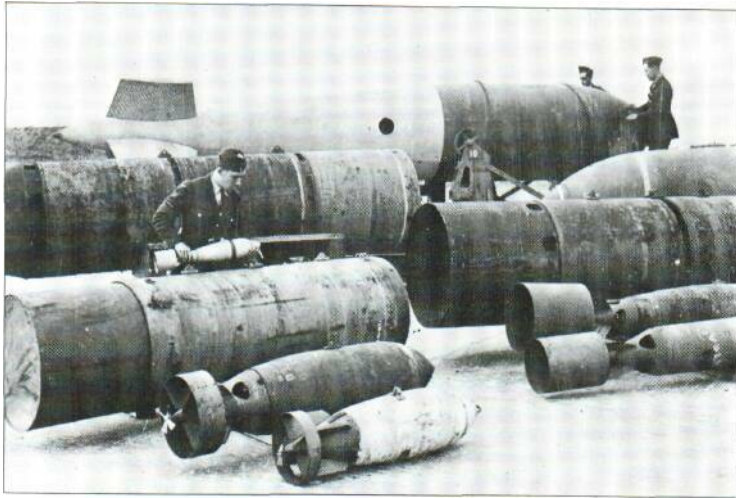
The bombs of the RAF. From the top: 9979-kg (22,000-lb) MC; 5443-kg (12,000-lb) HC; nose of 5443-kg (12,000-lb) MC; 3629-kg (8,000-lb) HC; 1814-kg (4,000-lb) HC; (right) 862-kg (1,900-lb) GP; 907-kg (2,000-lb) AP; (front) 454-kg (1,000-lb) and 227-kg (500-lb) GPs. The small bomb is 18 kg (40-lb).
