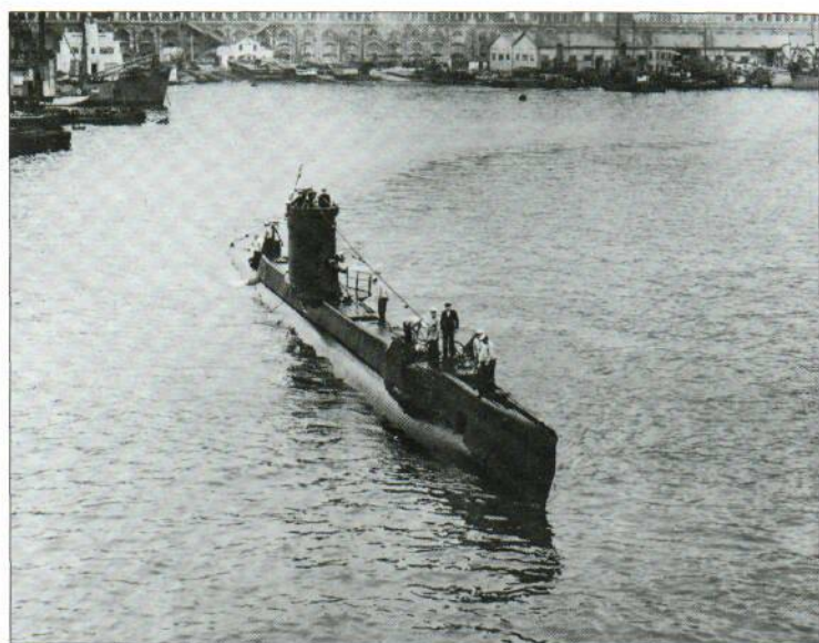
HMS Uproar shows the small size of these boats. In a short-range war, such as in the North Sea or the Mediterranean, endurance is much less important than manoeuvrability, and the 'U' class proved very handy, in spite of having been designed as a training boat.
