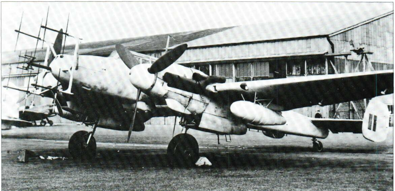
three and, with flame dampers and drop tanks as shown, had a maximum speed of typically 465 km/h (289 mph), barely faster than a Lancaster.
