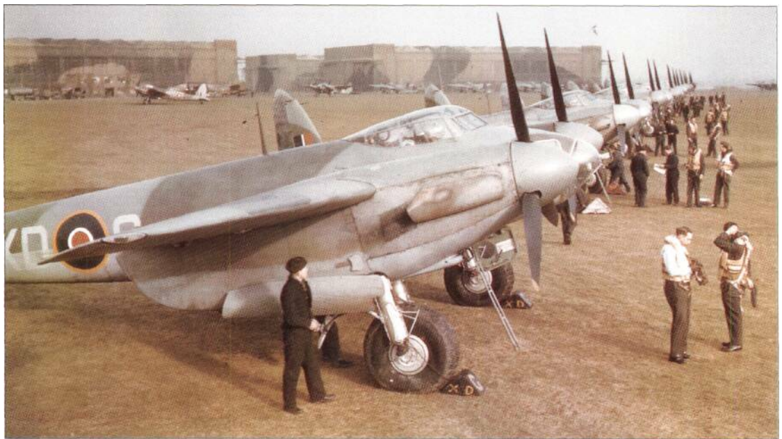
The wooden de Havilland DH 98 Mosquito was a legendary medium bomber which went into service in an extraordinary variety of configurations, including night fighter and reconnaissance.
