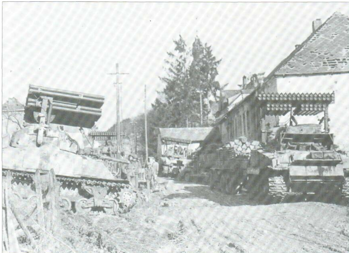
Left: M4 Sherman tanks sport the T-34 60-tube launcher known as Calliope. The tubes were made of plywood and could only be used a few times before disintegrating, but the launcher provided tank units with awesome close-range firepower.
