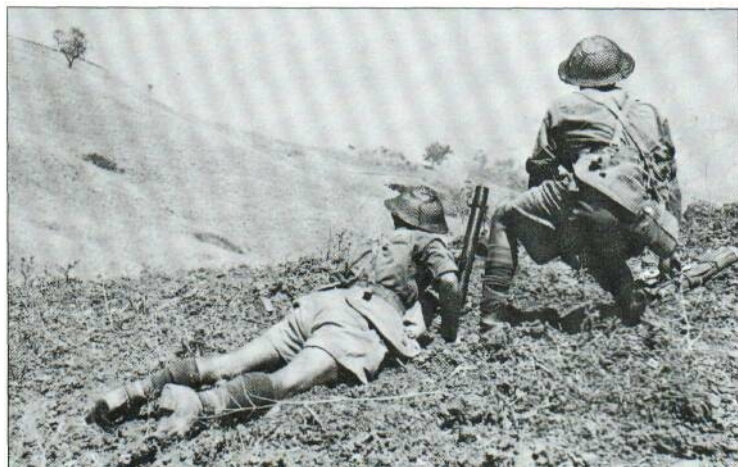
Soldiers of the 1st Battalion, The Hampshire Regiment, in action in Sicily in 1943, using a 2-inch Mortar. The mortar gunner is operating the trigger lever at the base of the barrel to actually fire the bomb while his partner observes the fall of the bomb.
