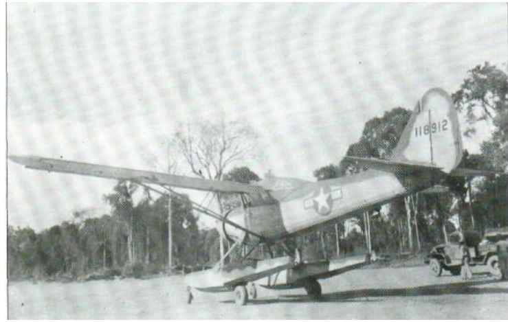
A United States Army Air Force L-1A is seen in Burma. Converted from a standard L-1A, it is metallic silver except for the top surfaces, which have been sprayed olive drab.
