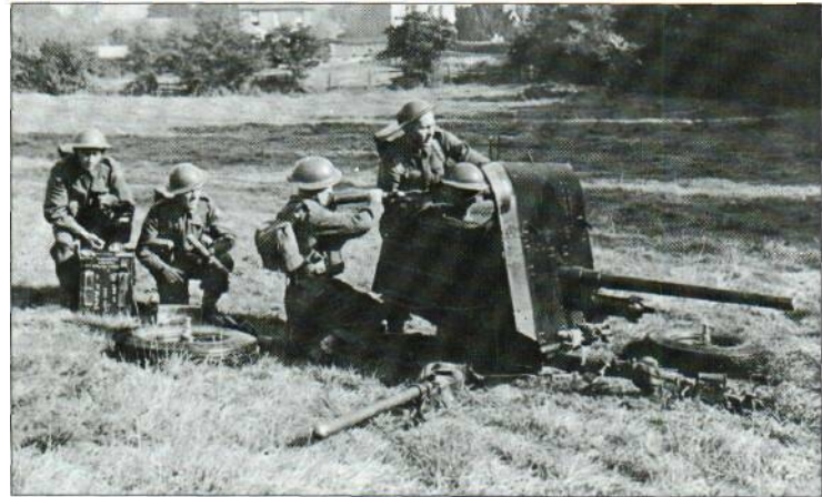
Right: A drill-book photograph of a 2-pdr gun and crew in action with the gun about to be loaded. Note that the ammunition is being passed from a box to the rear as the box on the gun shield was for emergencies only.
