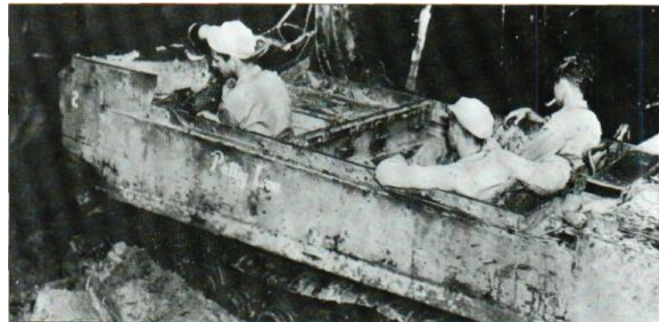
The M29C Studebaker Weasel was used as an amphibious cargo carrier, but could be used to carry personnel. Although small, it could carry useful loads over almost any type of terrain, and once in the water used its tracks to provide propulsion at slow but steady speed.
