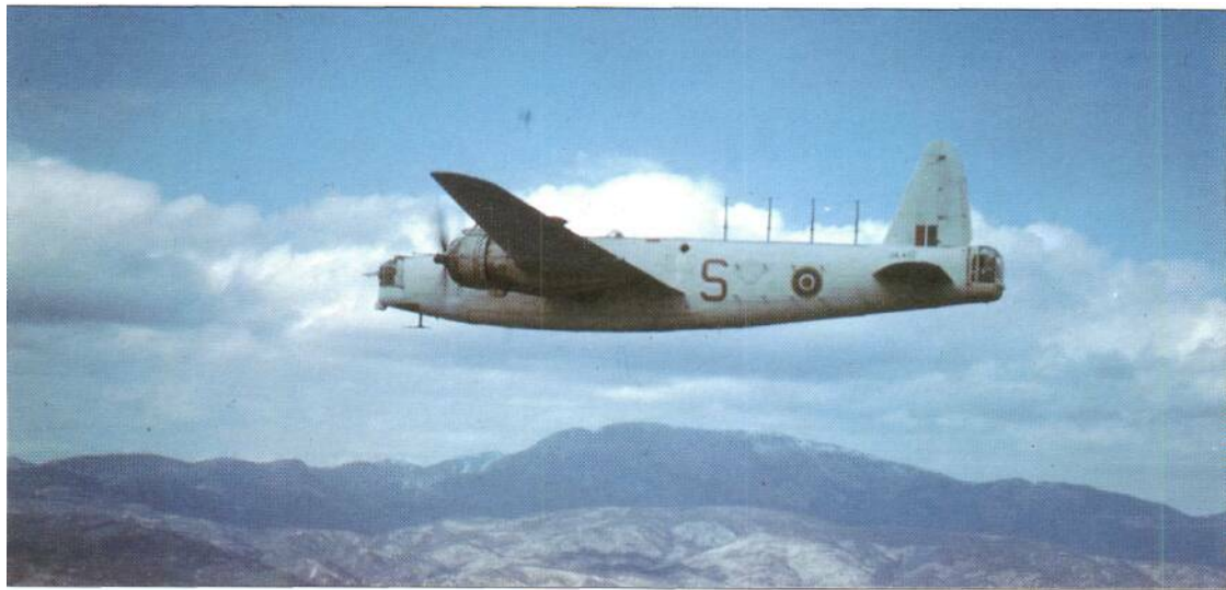
The Warwick GR.MkV did not enter service until late 1944. It carried ASV radar and a Leigh light and was used over the Bay of Biscay on anti-submarine patrols. This aircraft served with No. 179 Sqn.
