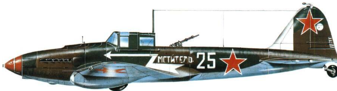
An Il-2m3 in late 1944 on the Eastern front. Soviet gunners often removed the rear cockpit canopy to give them a better field of fire.
