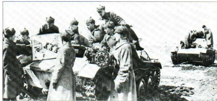
Right: The 20-mm gun armed T-60 light tank was not a great success in action, for it was too lightly armed and armoured and lacked power and mobility. It was kept in production simply to get some sort of vehicle to the Red Army following the disasters of the 1941 campaigns.
