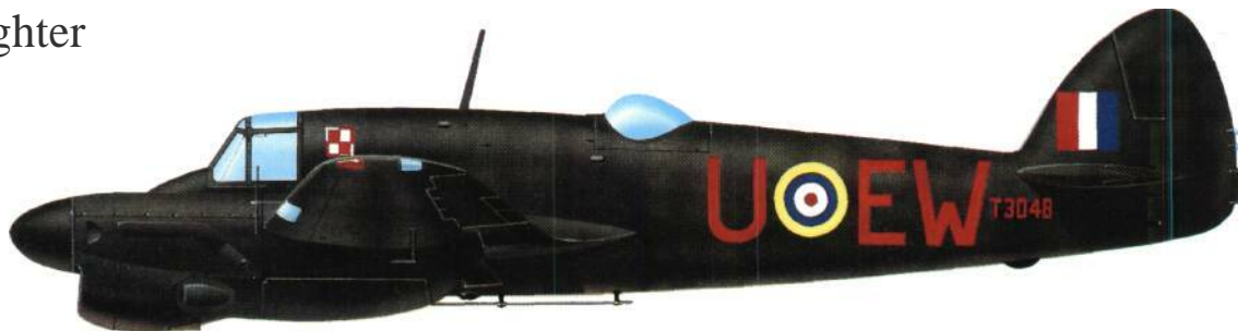
This Beaufighter Mk II served with one of the RAF's Polish squadrons, No. 307, from August 1941 until about mid-1942, when the Hercules-engined Beaufighter Mk VIF began to replace this Merlin-engined version.
