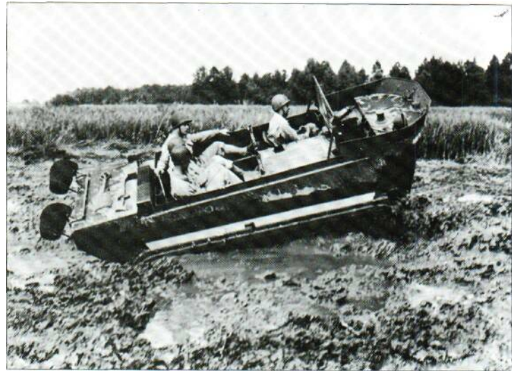
American personnel undergo a rather bumpy ride in an M29C Weasel over swampy terrain. The rear-mounted rudders can be clearly seen, and these were lowered once the vehicle actually entered the water.
