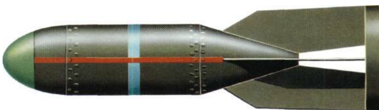
The Type 97 no. 6 59-kg bomb was a general-purpose weapon carried by a variety of Japanese aircraft, from heavy bombers to fighters.
