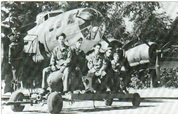
Armourers ride on two 454-kg (1,000-lb) GP bombs being brought up for loading in to Boeing B-17E day bombers of the United States Army Air Corps. The front bomb still has the transit plug fitted in the nose; this would have been replaced by the fuse and arming vane.
