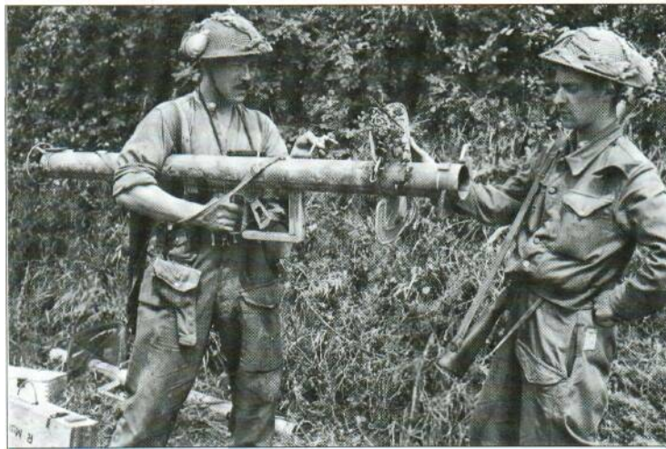
British troops examine a captured 8.8-cm (3.46-in) RP 54 in Normandy, July 1944. The shield can be seen, as can the main lever for the electrical generator used for firing; this looks like a large trigger under the tube. The RP 54/1 was essentially similar but used a shorter launching tube.
