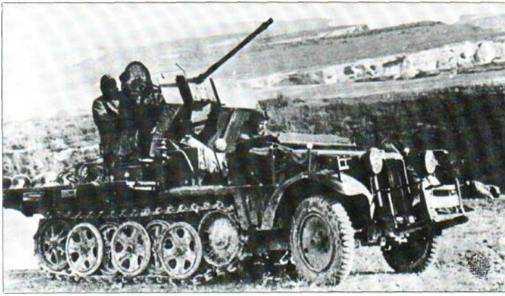
This SdKfz 10/4, a variant of the basic 1-tonne tractor, is fitted with a 2-cm (0.79-in) Flak 30 complete with its curved shield and with the sides folded down for action. Some of these vehicles were fitted with armoured cabs to protect the driver. Extra ammunition was usually carried in a towed trailer.
