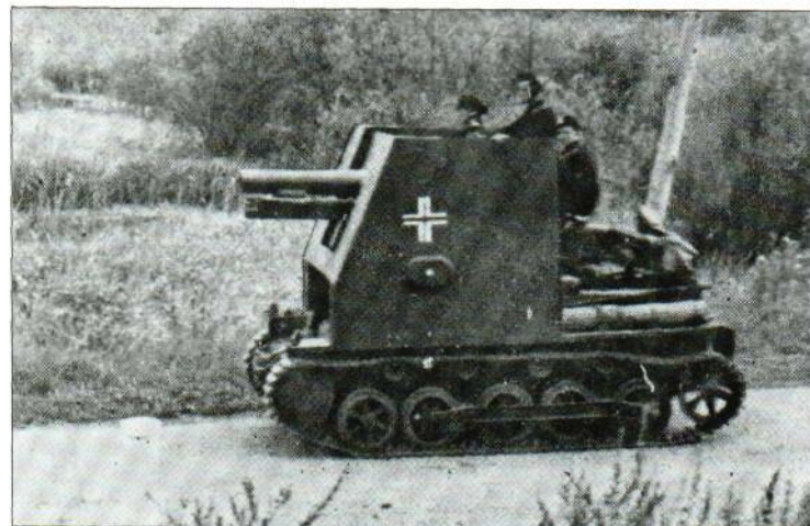
Taken from a German newsreel, this shot clearly shows how high and awkward the mounting of the 15-cm howitzer really was on the PzKpfw I chassis. The crew had only limited
