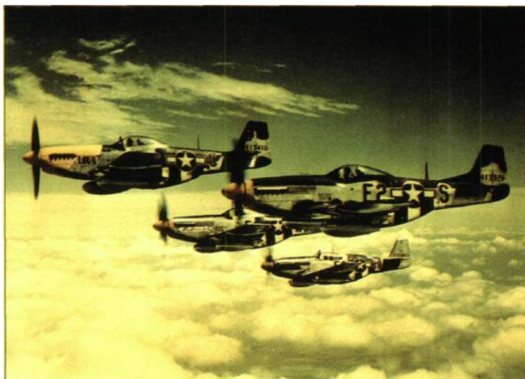
A group of USAAF long-range North American P-51 Mustang fighters - a superlative aircraft, believed by many to be the best of the war. It entered service in 1943 and achieved its 3347km (2080 mile) range by using wing drop tanks.
