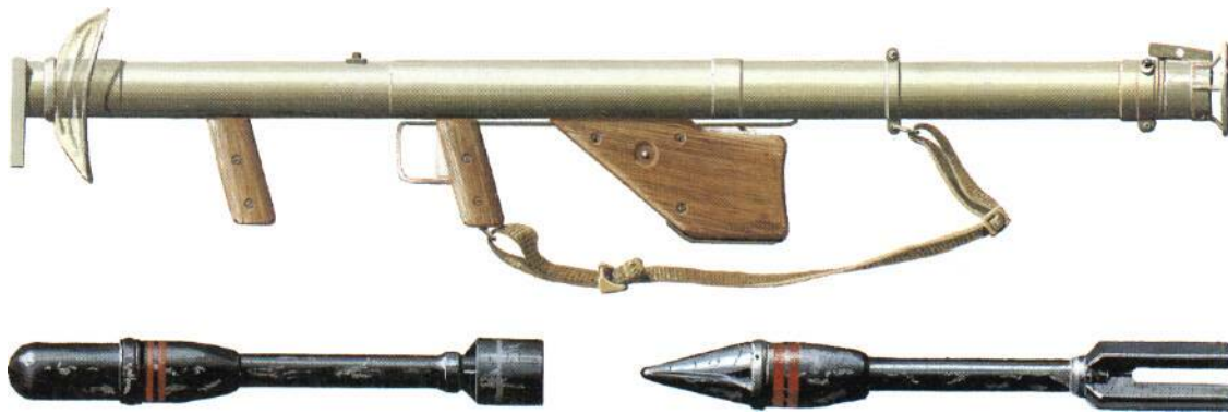
Above: The American 2.36 in (60 mm) Rocket Launcher M1 was the first of the bazookas and was used by the Germans as the original for their RP series. The M1 used a 'one-piece' barrel that could not fold and early versions (shown here) used a wire mesh shield around the muzzle to protect against rocket blast.
