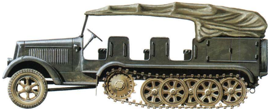
Famous as the main tractor for the 88-mm Flak 18, 36 and 37 guns, the SdKfz 7 also towed a wide variety of field artillery. Over 3,000 of these halftracks were in service by the end of 1942, and it was still in widespread use at the end of the war.
