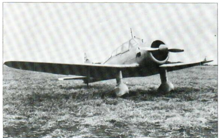
The Type 98 Chokusetsu-Kyodoki (Direct Co-operation Plane) was built by Tachikawa under the designation Ki-36. Trainer versions were designated Ki-55 and were used for kamikaze attacks late in the war.
