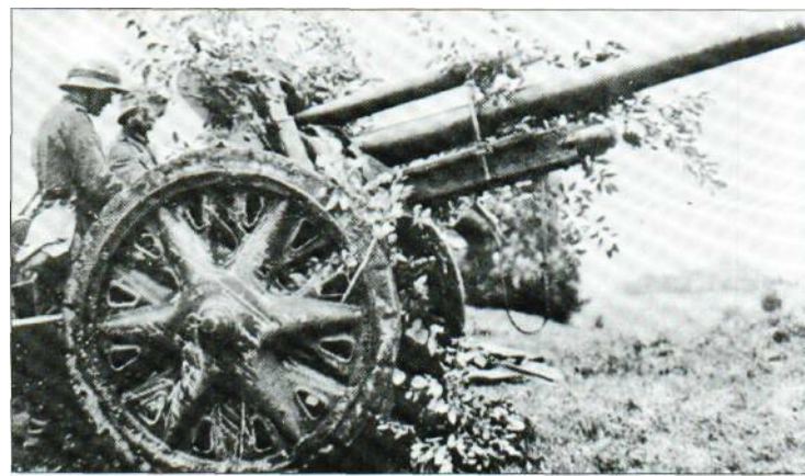
Above: Abandoned 10.5-cm leFH 18(M) howitzers in Normandy in June 1944. Note the obvious bulk and weight of the trail legs and spades that combined to make this howitzer too heavy for the mobile field role.
