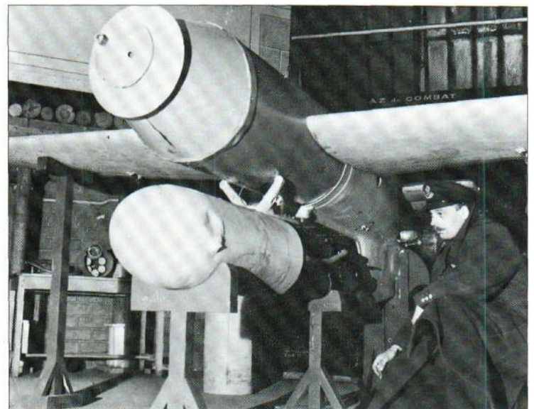
A Henschel Hs 293A stand-off guided bomb. This example was found near Paris in 1944 by Allied forces. The flat disc around the nose of the bomb prevented deep penetration before exploding.
