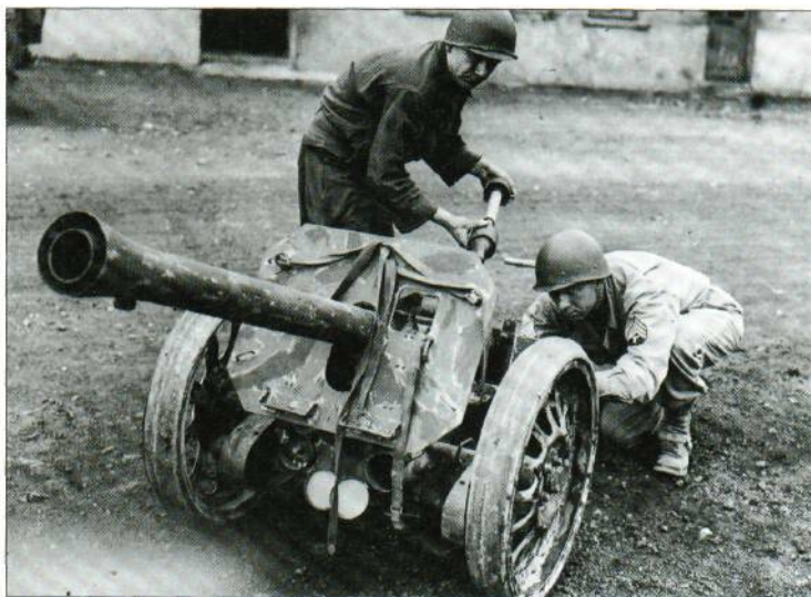
The 8.8-cm (3.46-in) Raketenwerfer 43 or 'Puppchen' was a form of anti-tank rocket launcher that was superseded almost as soon as it entered service in 1943 by the RP 43 series firing a very similar rocket. The RP 43 could be produced far more cheaply and quickly than the Puppchen, here being examined by Americans.
