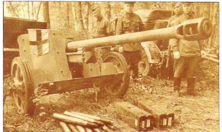
Soviet troops examine a captured Pak 38 early in the war. With tungsten-cored shot, the 5-cm weapon was the only German anti-tank gun capable of knocking out the Soviet T-34 tank. The gun was easily handled due to extensive use of light alloys in the manufacture of the carriage.
