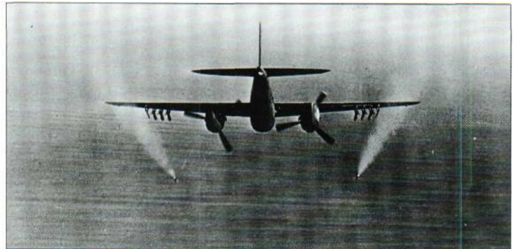
For use against 'soft' targets the 27-kg (60-lb) HE Type F shell was developed. This was a thick-walled shell, which exploded into small high-velocity fragments. Pilots using this weapon were warned not to use it under 550 m (600 yards) because of flying fragments.
