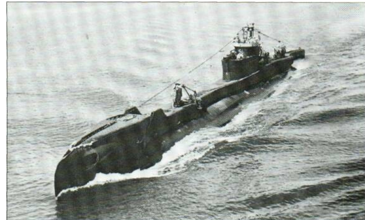
Below: HMS Tigris seen alongside a depot ship just before her final patrol. She was one of the original 'T' class boats, launched in October 1939, but she was lost in March 1943, probably to mines. Note the external tubes at the bow and amidships, and the unusual hull profile.
