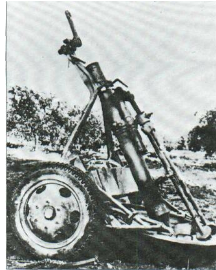
Above: The 120-HM 38 is seen on its wheeled travelling carriage, from which the mortar could be rapidly and easily emplaced. The wheeled carriage was often coupled to a limber that carried some ammunition. So successful was this mortar design that it is still in production.
