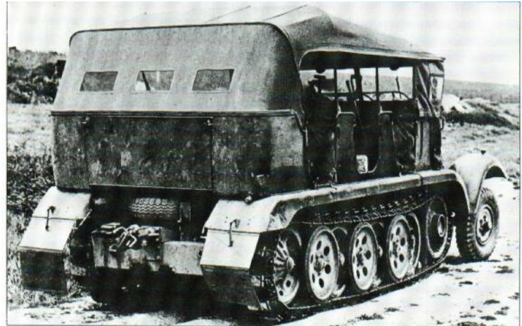
The SdKfz 6 was originally planned to tow the 10.5-cm (4.13-in) leFH18 howitzer, but was phased out of production in 1942 as lighter tractors
