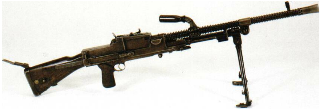
Above: The Czech ZB vz.26, one of the most influential designs of its day and the forerunner of the British Bren gun; this example has its straight 120- or 30-round box magazine missing.
