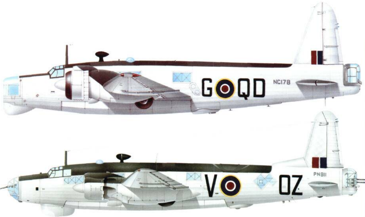
The Warwick GR.MkV did not enter service until late 1944. It carried ASV radar and a Leigh light and was used over the Bay of Biscay on anti-submarine patrols. This aircraft served with No. 179 Sqn.
