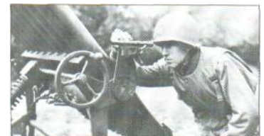
Above: A gunner checks the sights of the simple T-27 eight-tube launcher, generally fitted to CMC or Studebaker 2 1/2-ton trucks. The M8 was also fired from massive 120- or even 140-round launchers fitted to DUKW amphibious vehicles for beach assault.
