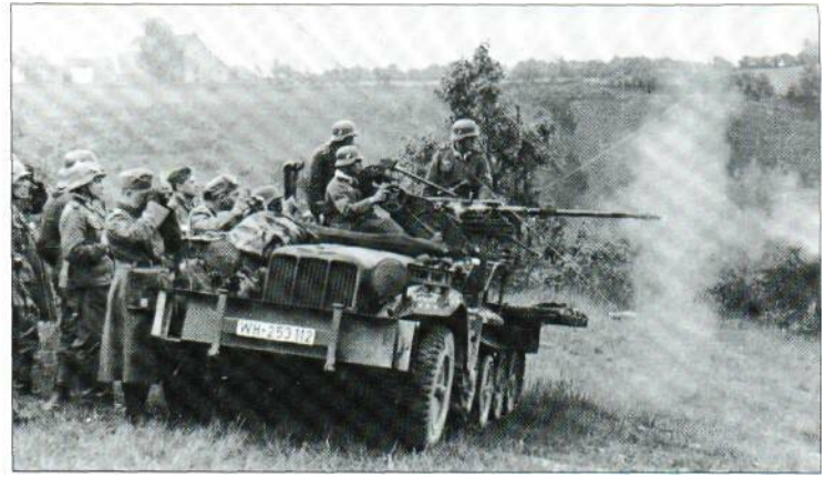
The light SdKfz 10 could mount either the 2-cm (0.79-in) Flak 30 or the Flak 38. These guns could be used against ground targets if required, as seen here. This is an SdKfz 10/4 with a Flak 30 and with the sides folded down to provide a firing platform.
