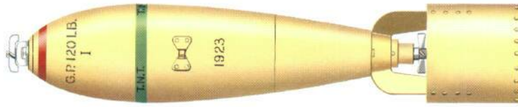
Left: The 54-kg (120-lb) GP HE bomb was one of a series of new, improved bombs of better aerodynamic shape than those used since World War I. This weapon replaced the old 50-kg (112-lb) GP bomb.
