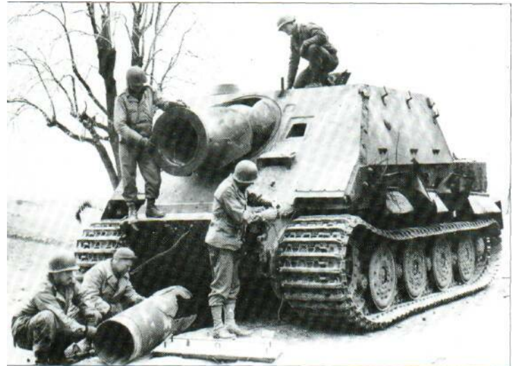
Above: This side shot of a Sturm-tiger shows the large armoured superstructure, mounting the 38-cm (14.96-in) rocket projector with the roof-mounted crane needed to load the projectiles in to the interior through a hatch at the rear.
