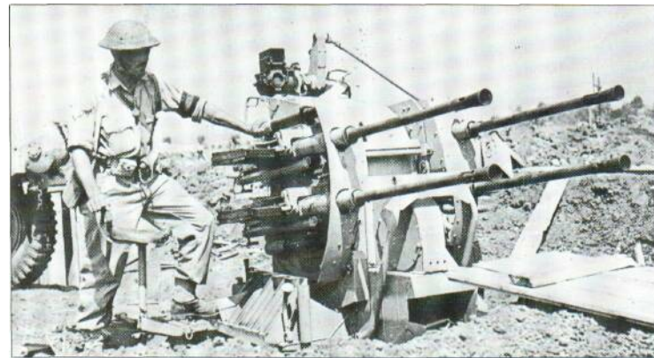
A British soldier examines a captured 2-cm (0.79-in) Flakvierling 38. The arrangement of the four barrels can be clearly seen, and the reflector sight is prominent. The
