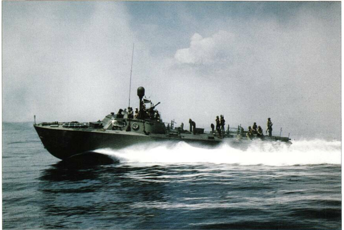
A US Navy PT boat intended for use in coastal waters, where its speed was put to good effect provided it had sufficient firepower - normally torpedoes and cannon.
