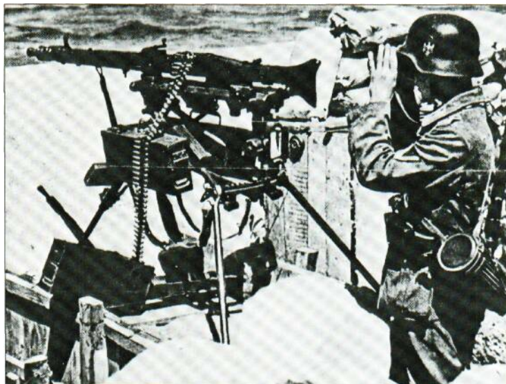
Above: An MG 42 mounted on the Lafette 42 for the heavy machine-gun role; this heavy tripod could be quickly adapted for the anti-aircraft fire role.
