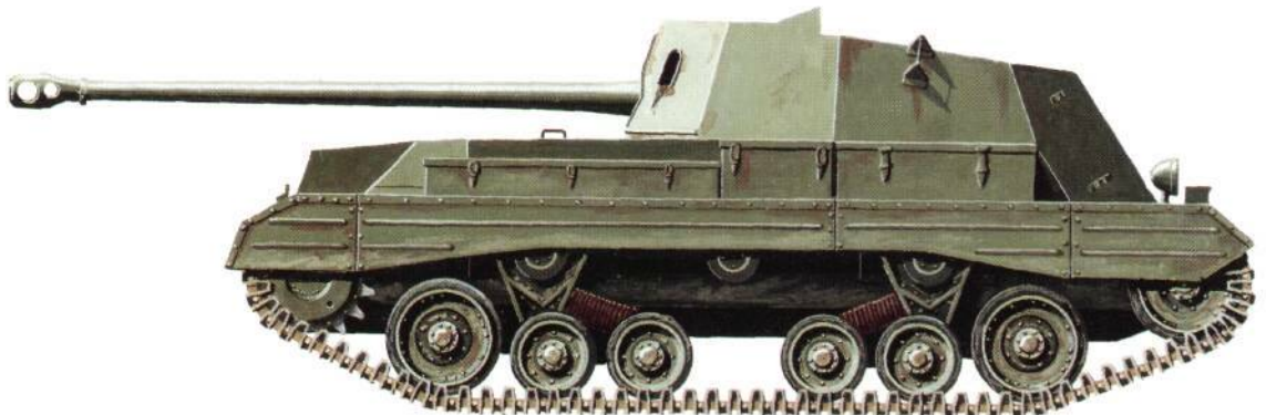
The British Archer was a conversion of the Valentine infantry tank to mount a 17-pdr (3-in/76.2-mm) anti-tank gun that fired over the rear hull.
