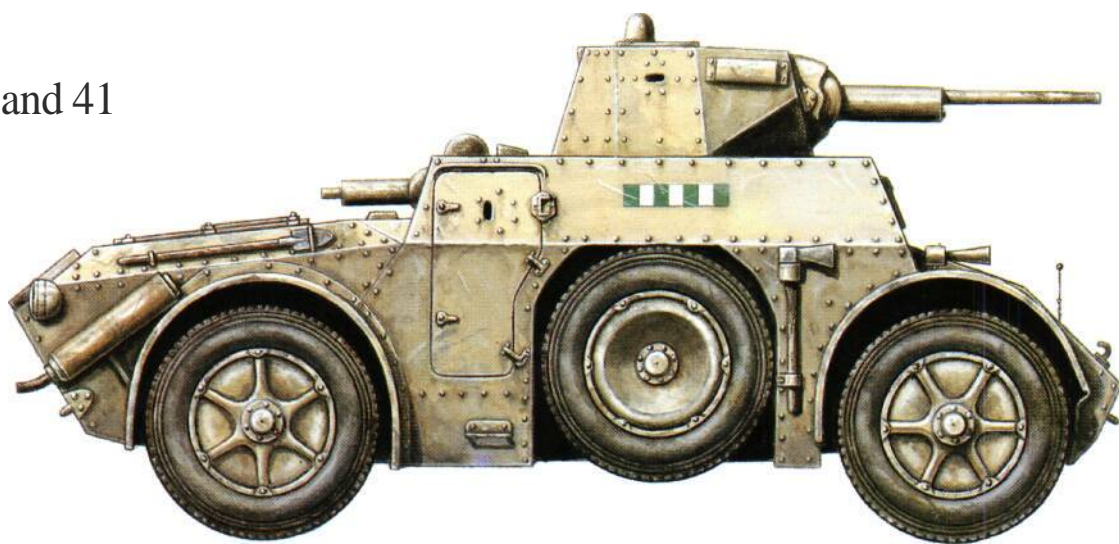
The Autoblinda 41, one of the most numerous of the Italian armoured cars, is shown armed with a turret-mounted 20-mm cannon and a machine-gun at the hull rear.
