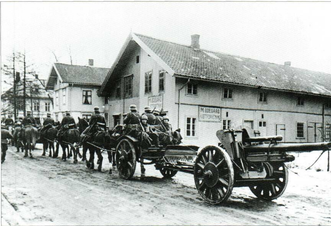
The German invasion forces in Norway in 1940. The horses are drawing a 105mm (4.13in) light howitzer or LeFH 18, a piece of field artillery that was overweight due to its solid construction.
