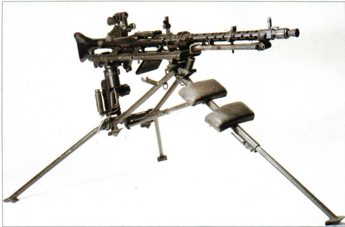
An MG 34 mounted for the heavy machine-gun role on a Lafette 34 tripod and complete with the indirect-fire sight; the pads on the front leg rested against the carrier's back when folded for transport.
