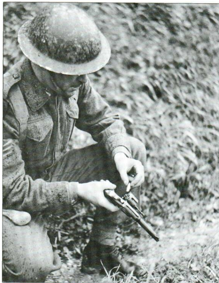
Above: A Canadian sergeant loads a Smith & Wesson 0.38/200 revolver. Empty cartridge cases were ejected by moving out the cylinder to the left and pressing a plunger normally under the barrel. All six spent cases were ejected together to allow each chamber to be reloaded one at a time, as seen here.
