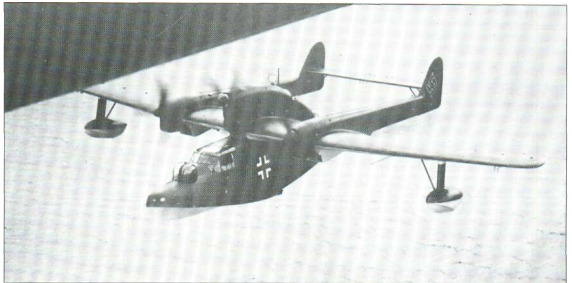
Blohm und Voss Bv 138 three-engine flying-boats replaced Dornier Do 18s of 6/MSGr 1 (previously Küstenfliegergruppe 506), this Bv138MS being based at Grossenbrode in the last year of the war.
