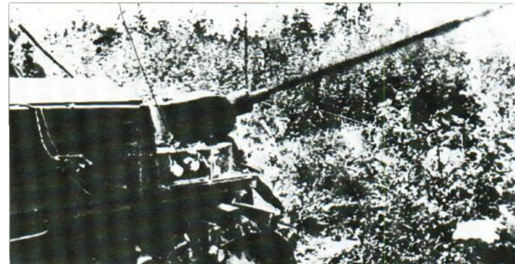
Above: One of the forward-mounted flame projectors carried by the Flammenpanzer II , which were mainly used on the Eastern Front although not many were actually produced. This projector is firing a rod of unlit fuel that could be ignited later when it lay on the ground.
