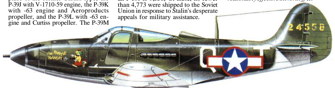
A Bell P-SBL Airacobra, operated by the 93rd FS, 81st FC in Tunisia in 1943. Successful in Soviet hands, the P-39 proved no match for the agile Zero in the Pacific, but was reasonably effective in North Africa.
