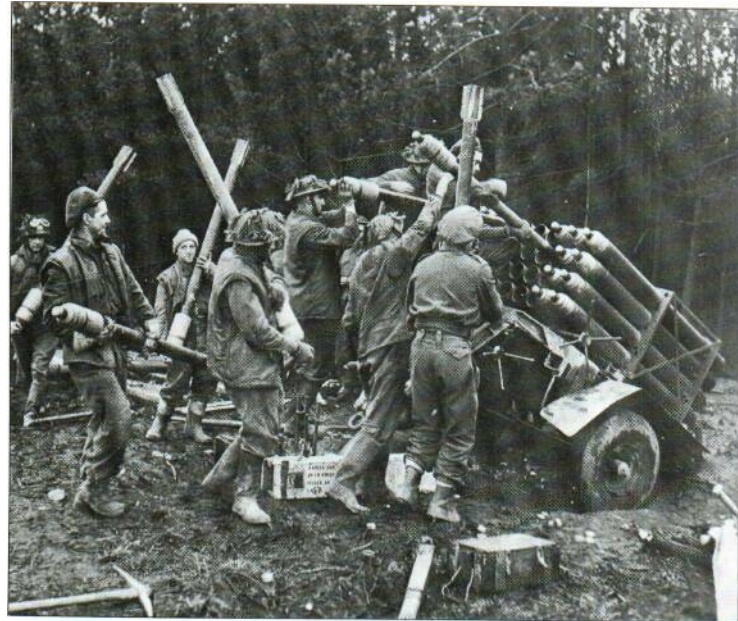
Above: Loading 30.5-kg (67-lb) rockets into the 32-round launchers was an exhausting job, but to be effective rockets had to be fired in
