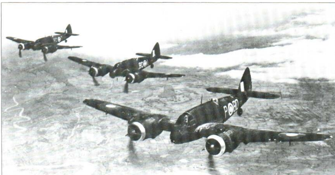
Three AI Mk IV-equipped Beaufighter Mk Is of No. 600 Sqn are seen here on a mission from Colerne during the winter of 1940-1.
