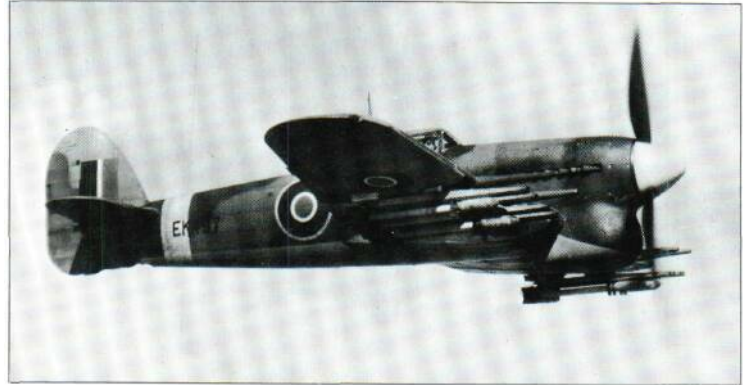
A Hawker Typhoon Mk1B, with the old 'car door' type canopy, carries 76.2-mm (3-in) rockets. The shells attached are the 27.22-kg (60-lb) SAP type. Other types used were the 27.22-kg (60-lb) T'fragmentation shell, 11.34-kg (25-lb) AP and 25-lb SAP shells, and concrete practice versions of these shells.
