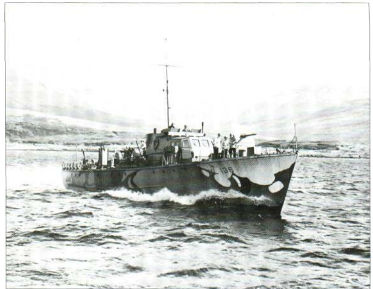
Above: ML 136 is seen on patrol off the Scottish coast early in her career. Armed with a Hotchkiss 3-pdr forward and two twin Lewis guns abaft the funnel, the class had room for more weaponry, and indeed six of the usual fit of 12 depth charges can be seen at the stern.
