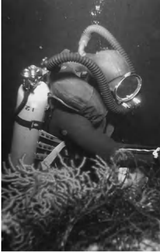
Fig. 1. A diver wearing a mixed-gas scuba, exposure suit, and face mask. Depth 300 ft (90 m) on the upper lip of Scripps Submarine Canyon, La Jolla, California. (U.S. Navy photograph, Naval Electronics Laboratory Center)
