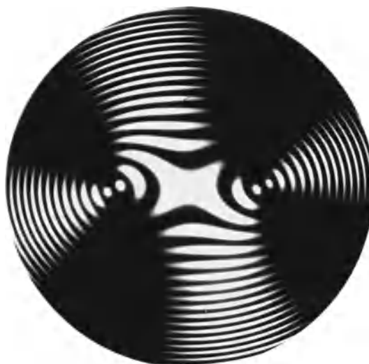
Fig. 6. Interference figure from Brazil topaz. (After M. Born and E. Wolf, Principles of Optics , 6th ed., Pergamon Press, 1980)
