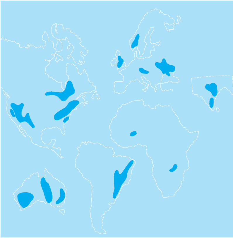
Fig. 3. Geographic distribution of 17 heat flow provinces where the linear relationship between measured heat flow and radiogenic heat production from near-surface rocks has been empirically determined. (After I. Vitorello and H. N. Pollack, On the variation of continental heat flow with age and the thermal evolution of continents , J. Geophys. Res. , 85(B2):983–995, 1980)
