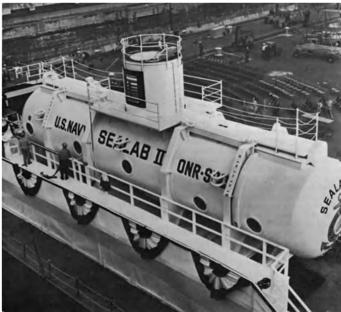
Fig. 3. Sealab II, an underwater station for deep-sea divers; 57 ft (17 m) long, 12 ft (3.7 m) in diameter. (U.S. Navy)
