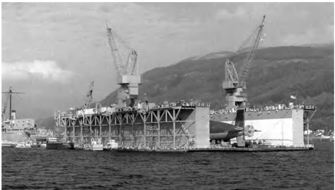
Fig. 3. USS Los Alamos (AFDB 7), a U.S. Navy floating sectional dry dock, at Holy Loch, Scotland (where it was located for many years), with a submarine docked in it. (U.S. Navy)
