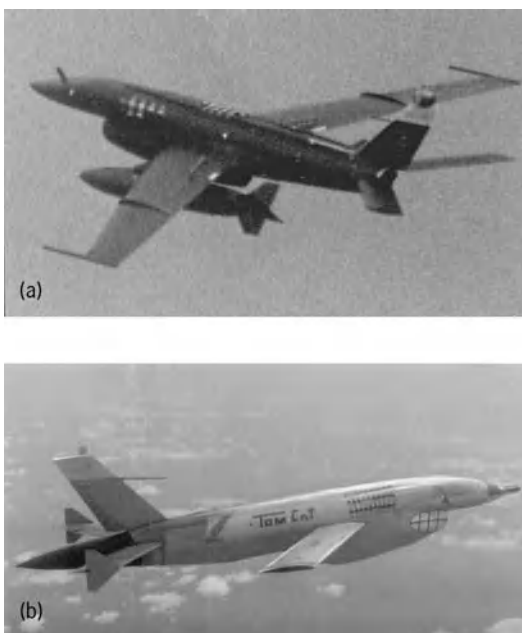
Fig. 2. Modified Ryan reconnaissance vehicles. (a) High-altitude version, with wing span of about 27 ft (8 m). It photographed from altitudes of 60,000 ft (18,000 m). (b) Low-altitude version with stretched fuselage, large wing tips, and end plates on horizontal stabilizer. It made photo runs at 1500 ft (450 m). (Teledyne-Ryan)
