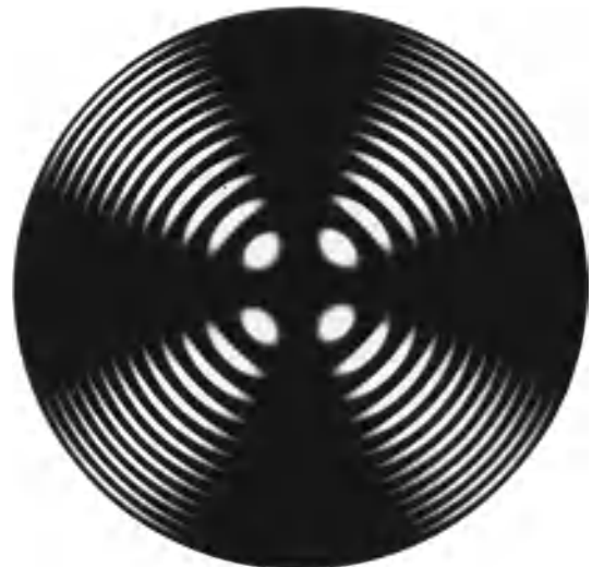
Fig. 5. Interference figure from flourspar that has been cut perpendicular to the optic axis and placed between crossed Nicol prisms. (After M. Born and E. Wolf, Principles of Optics , 6th ed., Pergamon Press, 1980)
