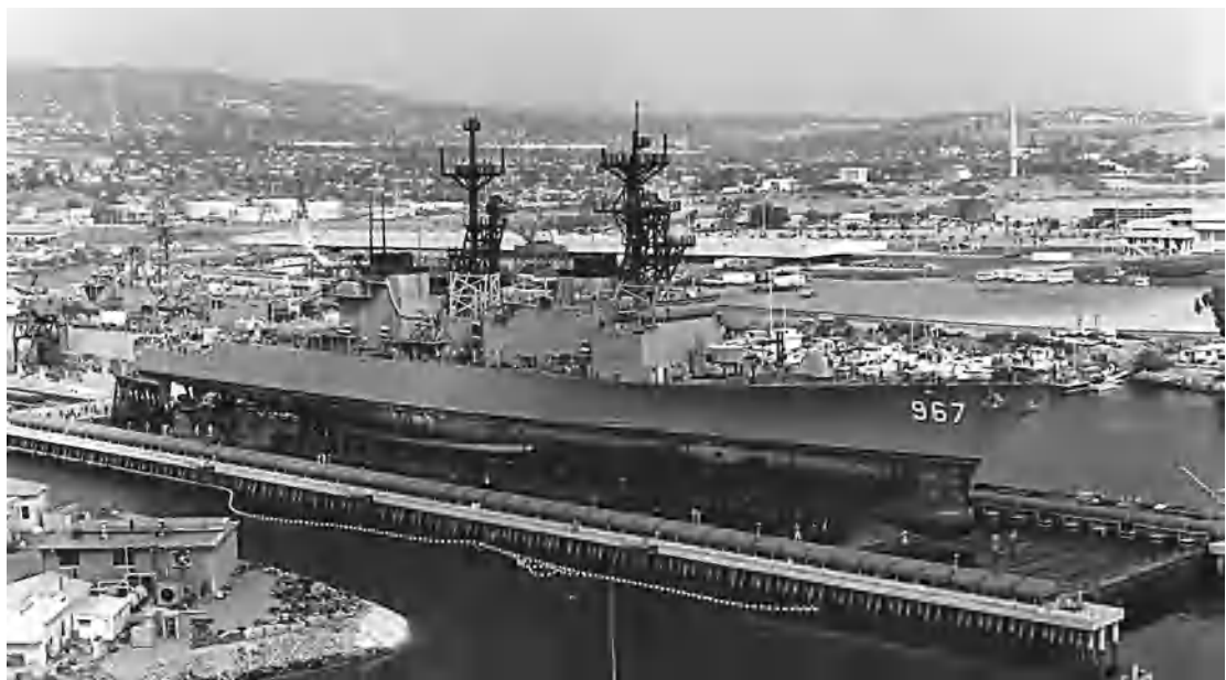
Fig. 7. USS Elliot (DD 967) on a mechanical or vertical lift at the Todd Pacific Shipyard at San Pedro, California, around 1984. When the shipyard closed in the early 1990s, the vertical lift system was disassembled and moved to Malaysia, where it is now operating (as of 2005). (Rolls-Royce Naval Marine Inc.)
