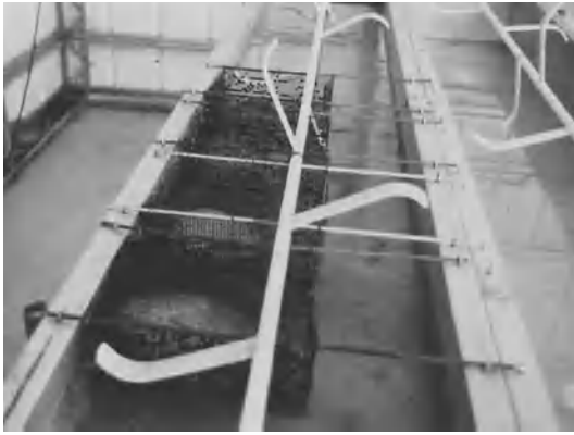
Fig. 4. Mechanized paddle troughs used in catfish aquaculture to provide aeration during egg incubation.
