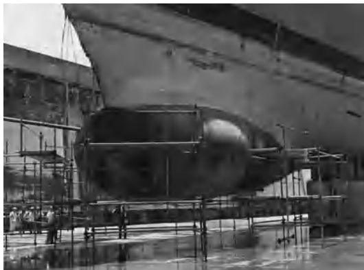
Fig. 1. SQS-26 low-frequency hull sonar, the largest U.S. hull sonar (the version onboard current surface ships, SQS-53, uses much the same sonar dome). Nearby workers give idea of scale. (U.S. Navy)
