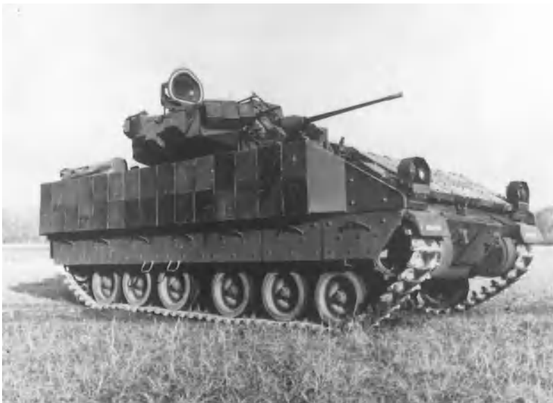
Fig. 10. M2 Bradley infantry fighting vehicle with M242 25-mm turret-mounted chain gun. (U.S. Army)
