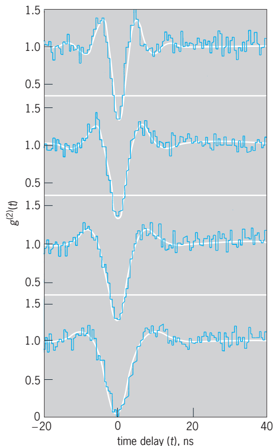
Fig. 9. Antibunching signal of a single \text{Mg}^+ ion for four different laser intensities. (After F. Diedrich and H. Walther, Nonclassical radiation of a stored ion , Phys. Rev. Lett. , 58:203–206, 1987)
