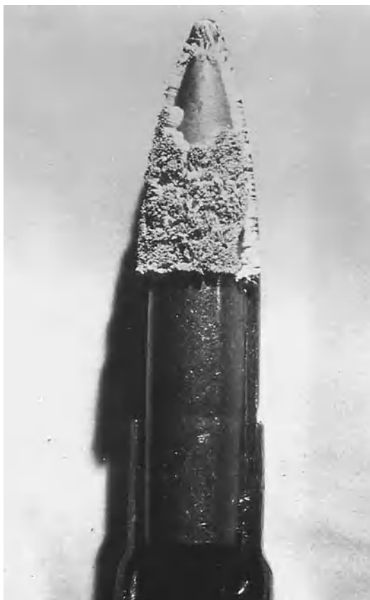
Fig. 5. Lead bullet with lead formate corrosion product formed by reaction with formic acid released from display case materials. (Smithsonian Institution)
