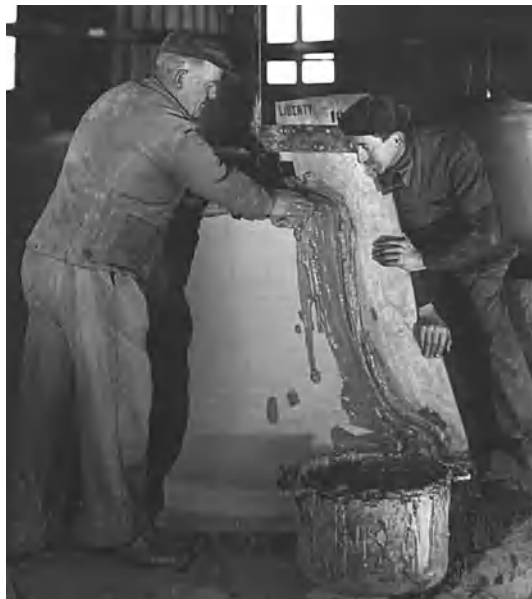
Fig. 1. Internal core of bell, which is shaped by revolving a strickle board. ( Les Fils de G. Paccard )
