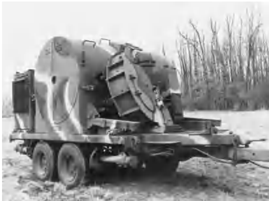
Fig. 14. Mine dispenser of GEMSS (ground-emplaced mine scattering system), mounted on flatbed chassis. (U.S. Army)
