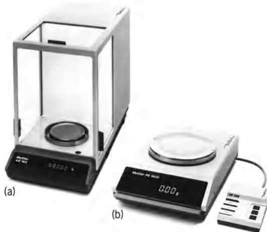
Fig. 4. Electronic balances. (a) Analytical balance. The weighing pan is nonpendulous and stabilized by a parallelogram linkage. Operating functions are controlled by single touch bar (integrated in readout panel) and include full-scale tare, automatic calibration, selection of weighing range, averaging period, and stability detector setting. (b) Electronic precision balance. Typically, balances reading to 1 mg or coarser require no enclosed weighing compartment, as they are less affected by air drafts than analytical balances. Operating features are similar to those of the analytical balance. The balance is operated through control bar along the front. (Mettler Instrument Corp.)
