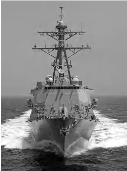
Fig. 6. Missile destroyer Forrest Sherman . With the demise of the Soviet Union, specialized antisubmarine ships no longer seem worthwhile. Forrest Sherman is a multirole destroyer designed to deal with air and underwater threats and to bombard land targets. Vertical launchers, one of which is set into the deck forward of the bridge, can fire vertically launched ASROC antisubmarine missiles as well as Standard anti-aircraft missiles and Tomahawk land-attack missiles. The radome atop the mast receives the data link from the LAMPS helicopter, which is used both to deal with submarines and to attack small surface craft. The anchor is located in the bow, instead of in the traditional position on the side, to clear the big sonar dome below water. (U.S. Navy)
