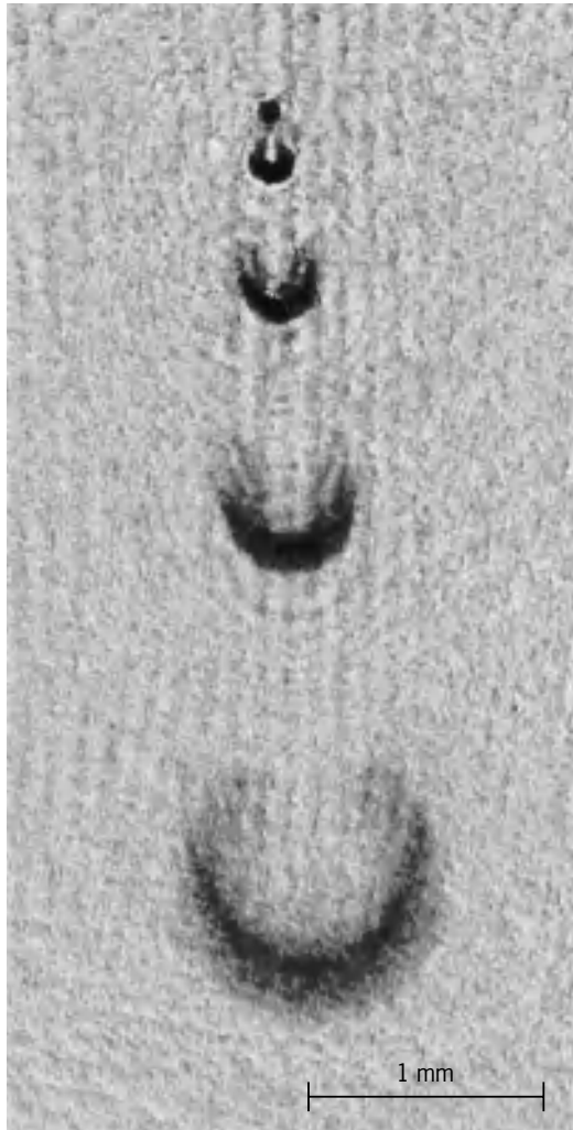
Fig. 2. Pulsed atom laser in operation, with pulses of coherent sodium atoms coupled out from a Bose-Einstein condensate that is confined in a magnetic trap.
