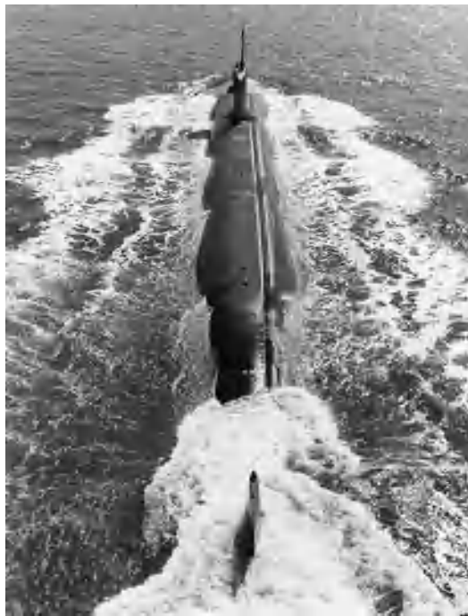
Fig. 3. Nuclear attack submarine USS San Francisco . The ridge running up the hull houses a towed array. (U.S. Navy)
