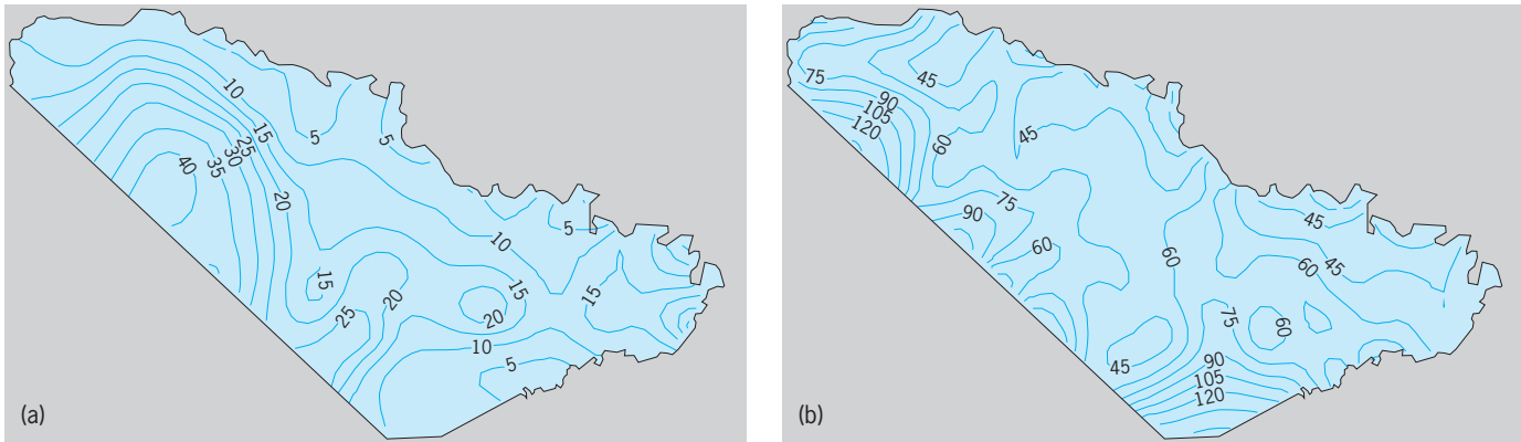
Fig. 24. Isarithm maps. (a) Map of actual sand content; values at the isarithms are in percent. (b) Map of the estimation variance of percent sand content; values at the isarithms are in percent squared.
