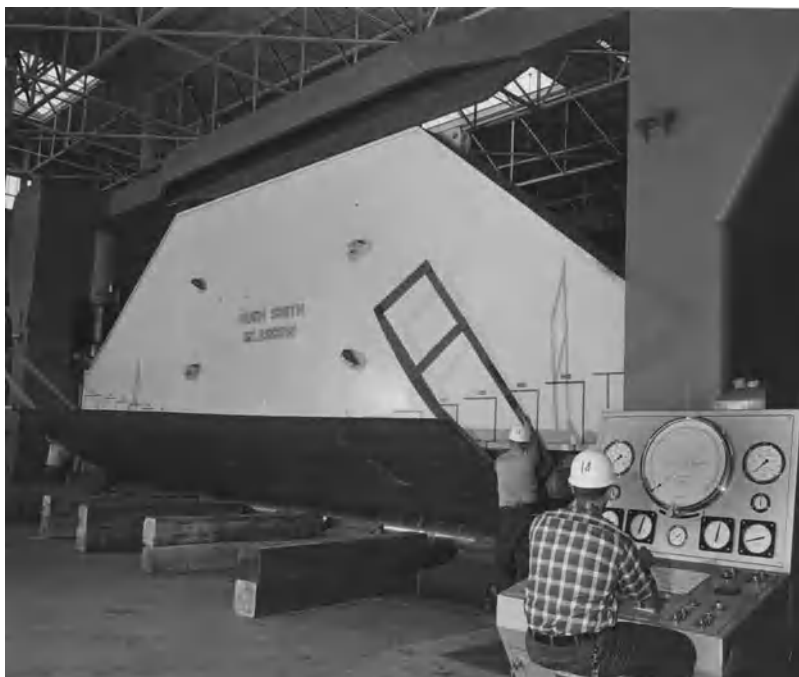
Fig. 5. Steel plate being formed in a roll press. (Newport News Shipbuilding)
