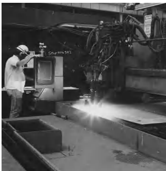
Fig. 4. Steel plate being cut to the desired configuration by a computer-driven cutting torch. (Newport News Shipbuilding)
