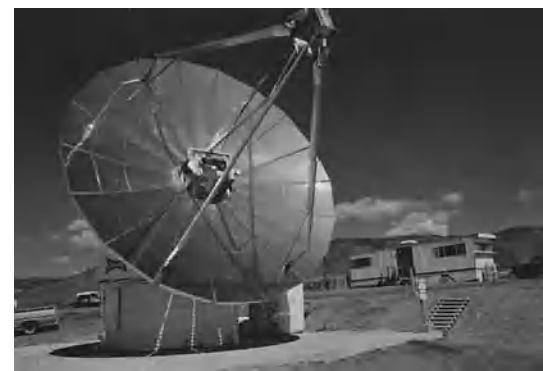
Fig. 7. Point-focus collector. (a) Schematic of collection process (after Jet Propulsion Laboratory, Fact Sheet on Parabolic Dish Systems: A Solar Thermal Concentrating Collector Concept , 5106-22/2, 1982). (b) Typical dish-receiver and engine module (Jet Propulsion Laboratory).
