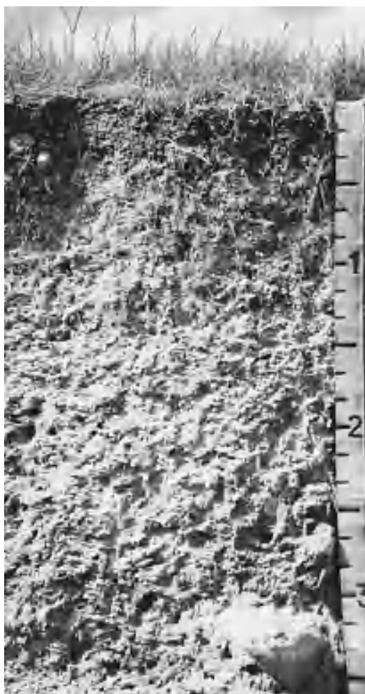
Fig. 11. Profile of an Aquept with thin, dark A horizons, fairly thick, light-gray B horizon, and stone in C horizon beside tape; numbers on scale indicate feet. 1 ft = 30 cm. (Photograph by R. W. Simonson)
