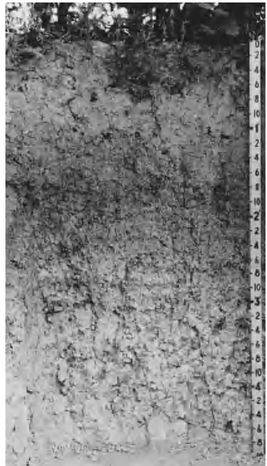
Fig. 6. Profile of a Udalf with A and E horizons 12 in. (30 cm) thick over darker B horizon with blocky structure grading into C horizon at a depth of about 4 ft (1.2 m); larger numbers on scale indicate feet. 1 ft = 30 cm. (Photograph by R. W. Simonson)
