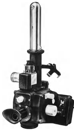
Fig. 2. Periscopic sextant for use in aircraft.
