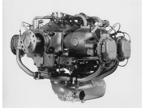
Fig. 6. IOL-200, four-cylinder, liquid-cooled engine used in the Voyager airplane during its nonstop, unrefueled circumnavigation of the globe. (Teledyne Continental Motors)
