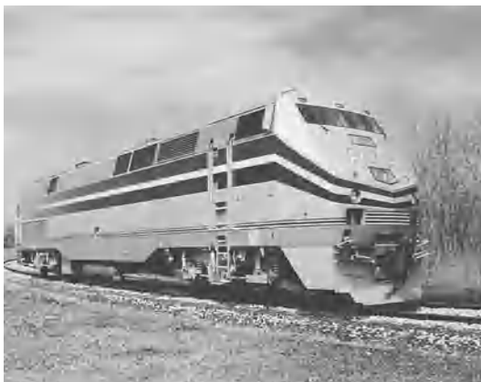
Fig. 4. The genesis, 4000-hp passenger locomotive capable of speeds up to 103 mi/h (165 km/h). (Amtrak)
