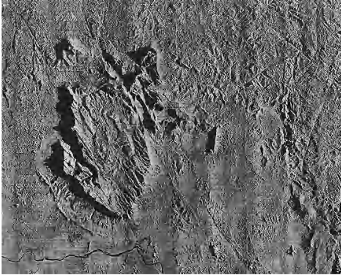
Fig. 8. Side-looking radar (SLAR) imagery of a portion of the jungle-covered Guayana Precambrian Shield of Venezuela. This imagery was acquired by a Goodyear synthetic-aperture X-band (3.12-cm) radar system mounted on board an Aero Service Caravelle aircraft. The flight altitude was 46,000 ft (14,030 m). The east-west dimension of the image mosaic is approximately 104 mi (168 km).
