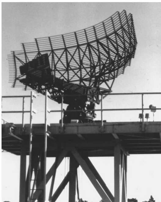
Fig. 6. AN/SPS-49 search radar antenna, which forms a vertical fan beam for the two-dimensional L-band radar widely used in the U.S. Navy. (Raytheon Co.)
