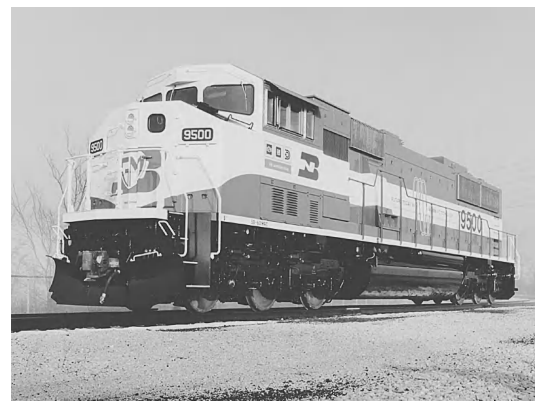
Fig. 2. Locomotive with ac asynchronous traction motors. (General Motors)
