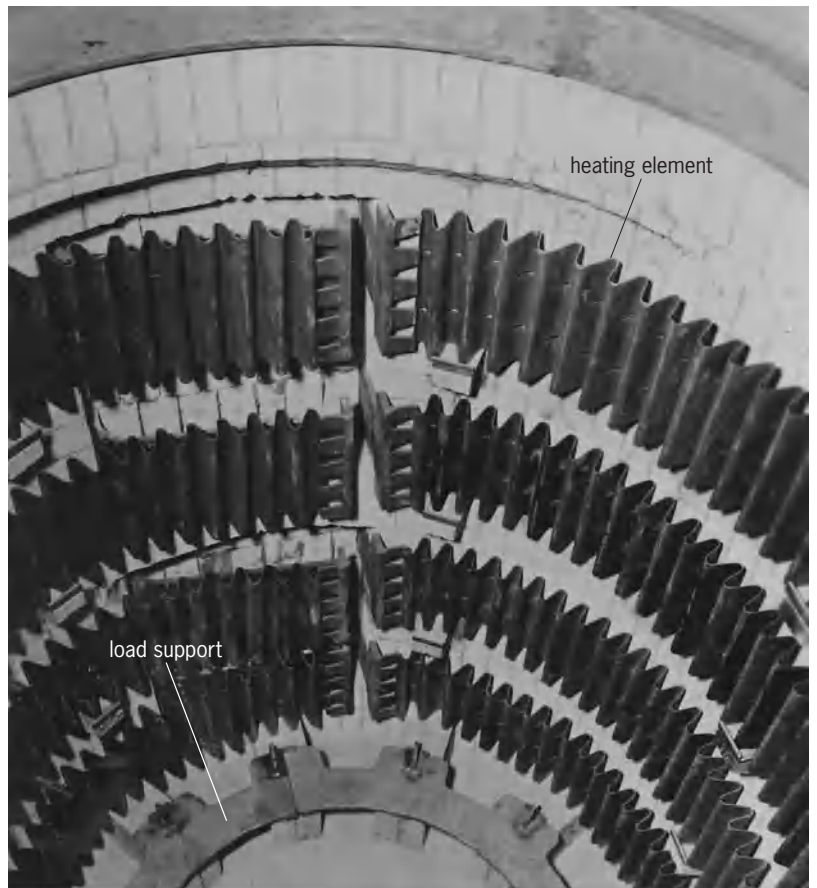
Fig. 6. Interior of high-temperature pit-type carburizing furnace, using radiant heating. (Lindberg Industrial Corp.)
