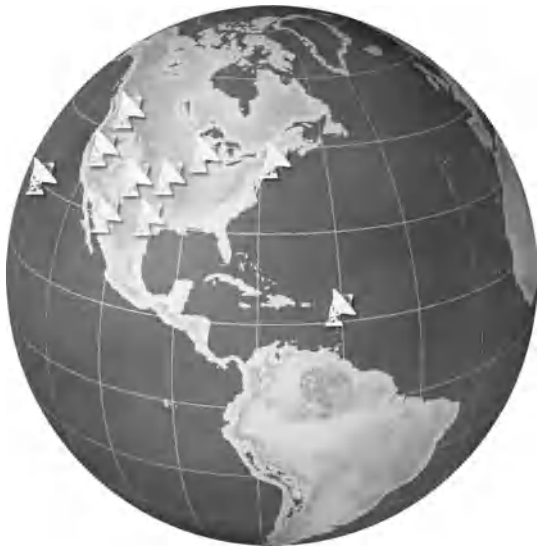
Fig. 4. Artist's conception of the 10-element Very Long Baseline Array. Signals from each of the 10 antennas are independently recorded on magnetic tape or disks which are then sent to the array headquarters in Socorro, for processing to form radio images with an angular resolution better than 0.001 arcseconds HST. (NRAO/AUI/NSF)
