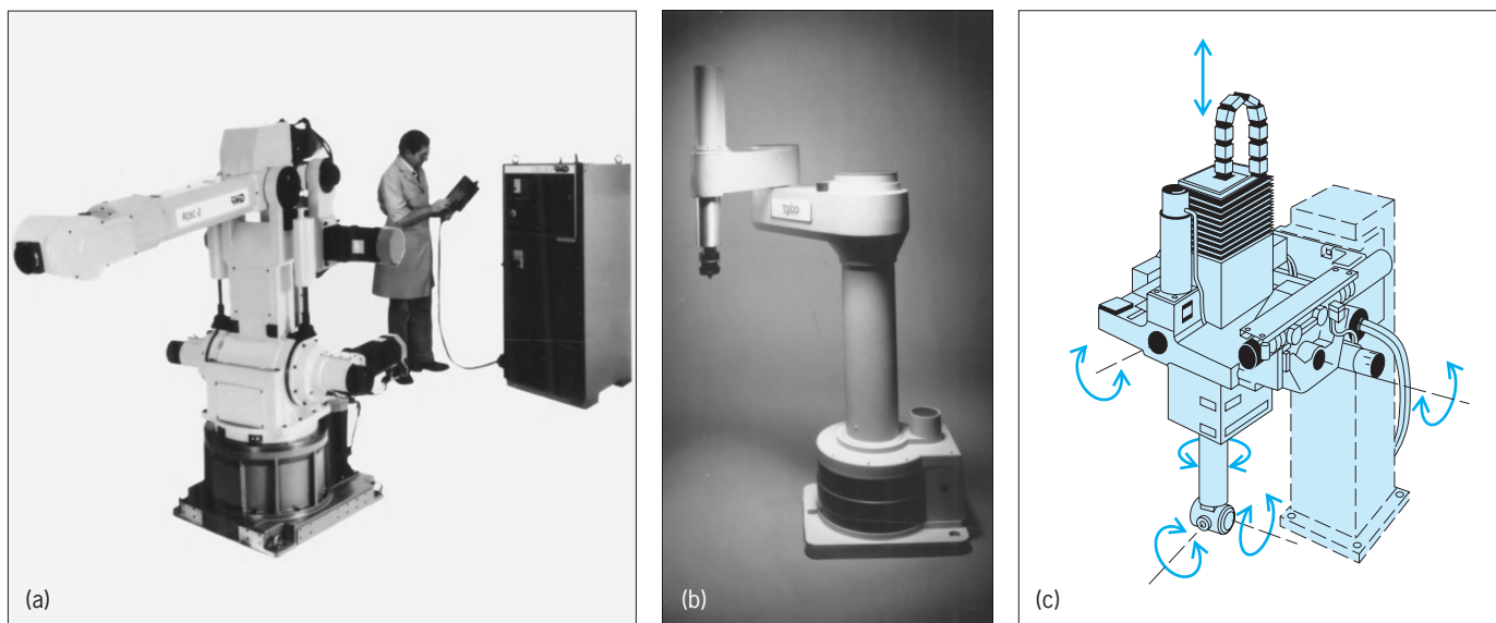
Fig. 1. Industrial robots. (a) Articulated, with rotary joints (GM Fanuc Robotics Corp.). (b) Selective compliance assembly robot arm (SCARA) configuration (Adept Technology, Inc.) (c) Overhead gantry.
