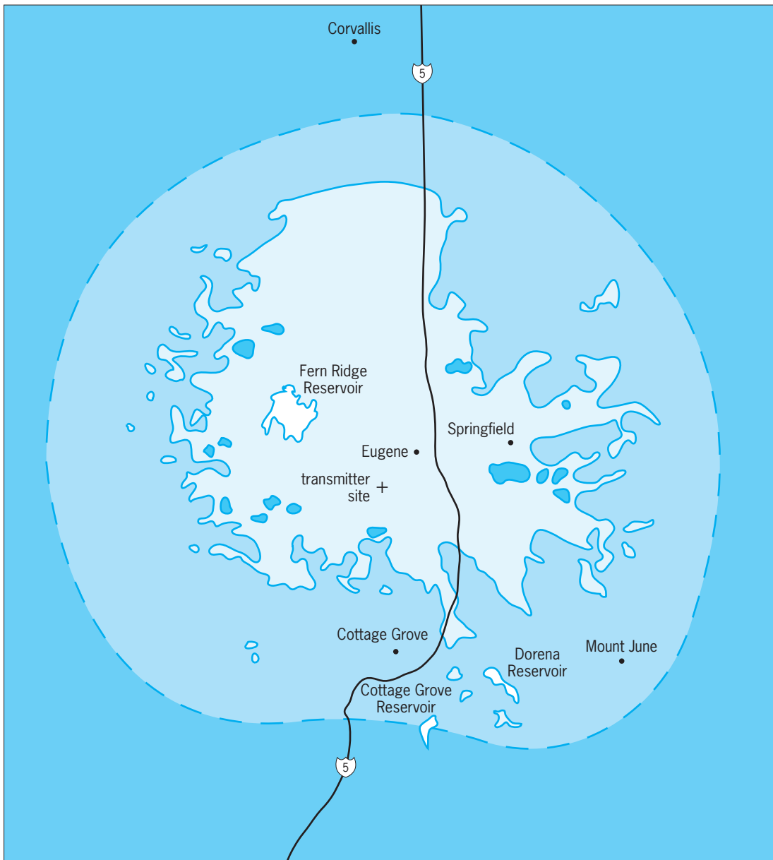
Fig. 5. Predicted 3.16-mV/m coverage contour for the 100-kW station KUGN in Eugene, Oregon. The broken line represents coverage based on FCC field strength curves. The solid lines and “islands” represent a more realistic depiction of coverage that explicitly takes into account terrain obstructions.
