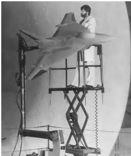
Fig. 1. Scale model of fighter aircraft being mounted inside test section of large wind tunnel. (NASA)
