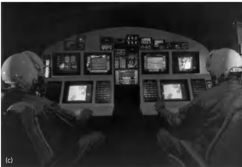
Fig. 9. Military aircraft instrumentation. (a) Soviet Mikoyan MiG-29 cockpit. (b) United States Navy/Marine Corps McDonnell Douglas F/A-18 cockpit (parts a and b from Aviat. Week Space Technol. , 129(12):32, September 19, 1988). (c) Operators' stations for on-board mission management system of advanced strategic aircraft (Boeing Co.). (d) Advanced multirole, multifunction cockpit system (Boeing Co.).
