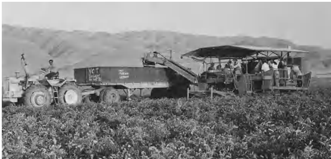
Fig. 6. This tomato harvester cuts the vines, removes the fruit, and then loads it into a truck after the rejected fruit has been removed by the sorters. (Blackwelder Mfg. Co.)
