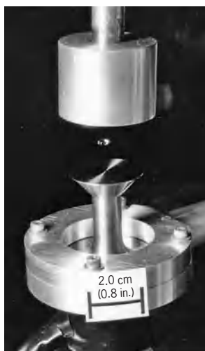
Waterdrop acoustically levitated in air between a vibrating surface (below the drop) and a reflecting surface (above the drop). The drop is located slightly below the pressure antinode of a 21-kHz standing wave. The equilibrium shape of the drop is oblate because of the balance between acoustic radiation pressure and capillary stresses.
