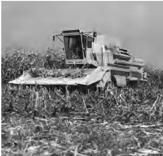
Fig. 5. Self-propelled combined harvester-thresher. (Sperry New Holland, Division of Sperry Rand Corp.)
