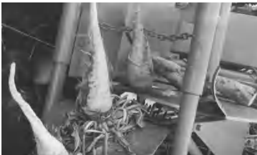
Fig. 10. Detail of spiked-wheel harvester gathering sugarbeets. (Blackwelder Manufacturing Co.)
