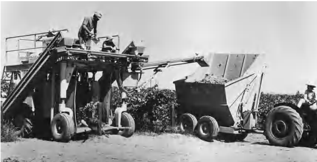
Fig. 8. These grapes are being harvested by beaters which impact the vines. The berries and bunches are collected on conveyors and then delivered to a dump trailer. (Up-Right Inc.)
