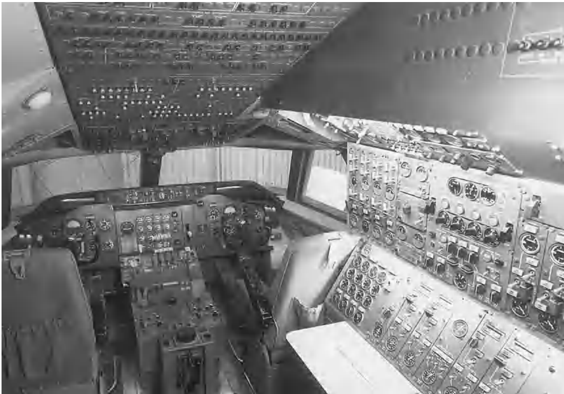
Fig. 1. Cockpit displays and flight engineer's instruments in Boeing 747. (Boeing Co.)
