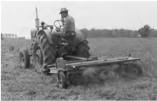
Fig. 18. Forage crusher for cracking or shredding stems to accelerate field drying rate of forage crops.
