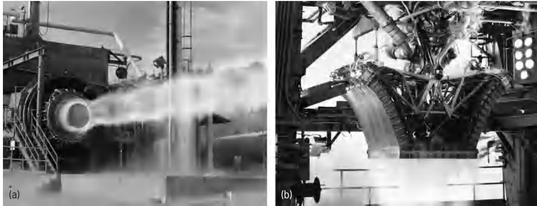
Fig. 1. Static firing tests of (a) aerospike engine with 250,000 pounds (1,112,000 newtons) of thrust, and (b) linear aerospike engine with 125,000 pounds (556,000 newtons) of thrust. Both engines use hydrogen/oxygen propellants. (Boeing Company, Rocketdyne Division)
