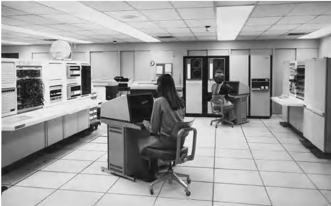
Fig. 2. Analog-hybrid laboratory equipped with a HYSHARE 600 system. This system can include up to six analog computer consoles and one or more digital processors for multiuser, multitask applications. ( Electronic Associates, Inc. )
