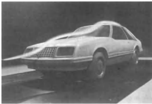
Fig. 2. Aerodynamic flow over an automobile. (Ford Motor Co.)
