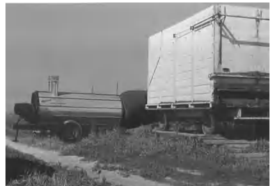
Fig. 16. Special wagon rack attached to portable oil-burning crop drier for finish-drying chopped forage.
