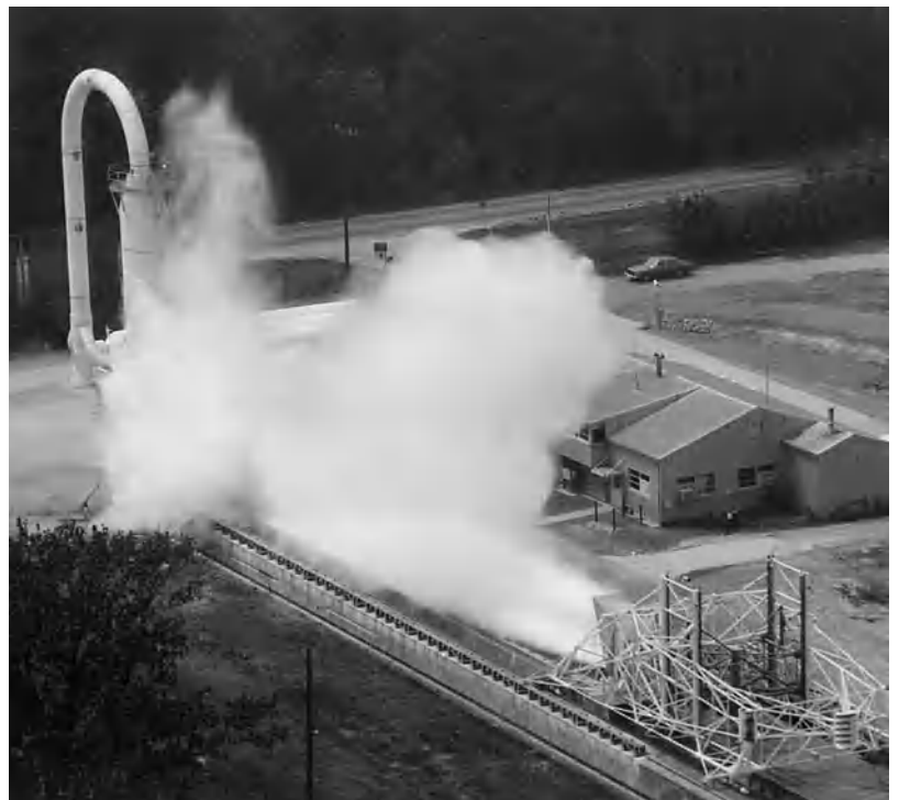
Fig. 4. Test sled propelled down runwaylike track by high-pressure water to test aircraft components during simulated landing. (NASA)
