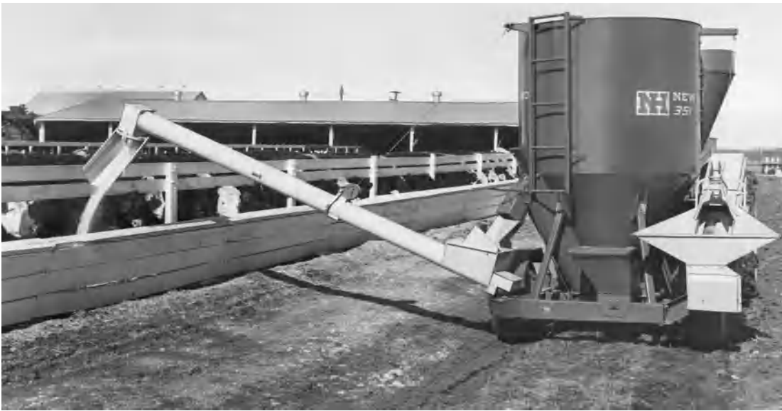
Fig. 3. Portable feed grinder-mixer delivering processed feed to feed bunk. (Sperry New Holland, Division of Sperry Rand Corp.)
