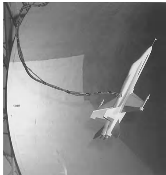
Fig. 2. Free-flying scale model aircraft in wind tunnel; attached cable contains sensors and other measurement instruments. (NASA)
