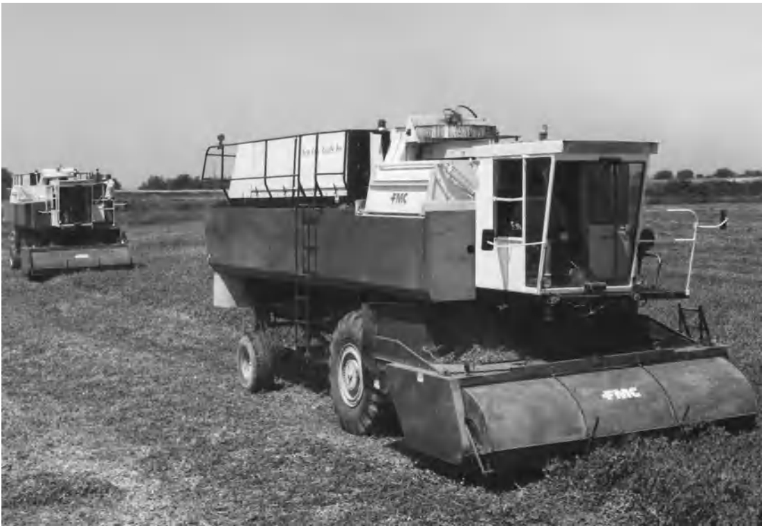
Fig. 7. Pea pods being harvested and threshed by a self-propelled pea viner machine. (FMC Co.)
