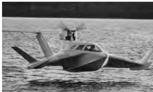
Fig. 3. Wing-in-ground-effect craft used over water as a commuter vehicle. (FlareCraft Corp.)
