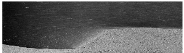
Figure 8 Flow separation visualized behind a dune bedform. Flow right to left. Flow is visualized by the path of neutrally buoyant particles within the water, which shows the recirculating flow within the dune leeside.
