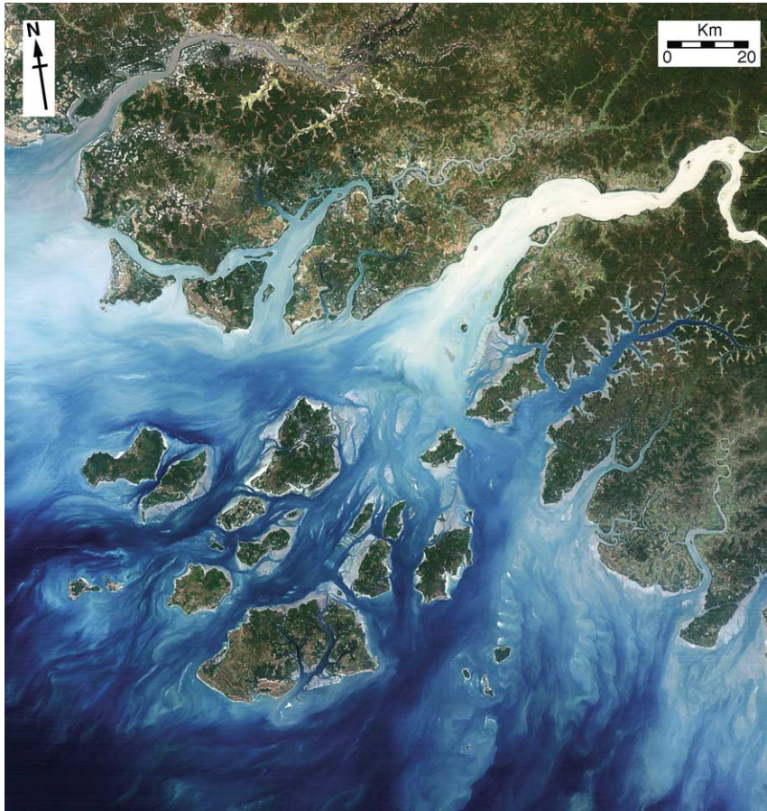
Figure 5 Satellite remote sensing image of tidal sand-banks off the coast of Guinea in West Africa. Note the plumes of sediment moving along the channels between the banks. The high tidal velocities are reworking sediment supplied by local rivers. (Picture taken from LANDSAT-4TM using bands 3, 2, and 1 for red green and blue colour channels, respectively.)
