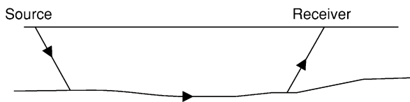
Figure 2 Principle of seismic refraction: a seismic wave travels between a surface source and a receiver along a subsurface boundary across which there is an increase in seismic velocity.
