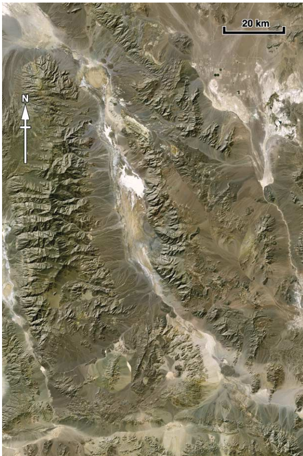
Figure 8 Satellite image of Death Valley, USA, showing clearly the fault scarps and surface deposits. This is a LANDSAT-5 TM image using bands 3, 2, and 1 for red, green, and blue colour channels.
