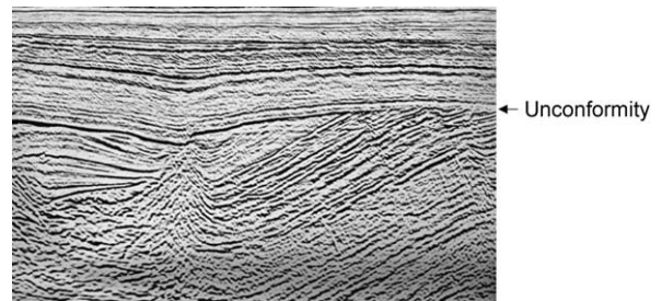
Figure 13 Seismic section showing a prominent angular unconformity.
