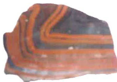
Figure 1 Hand specimen (15cm wide) of folded Archaean BIF from the Yilgarn Craton, Western Australia. The conspicuous red and black banding is mesobanding; the red mesobands are chert and the black mesobands consist mainly of iron oxides and microcrystalline quartz. (Photograph by GJH McCall).
