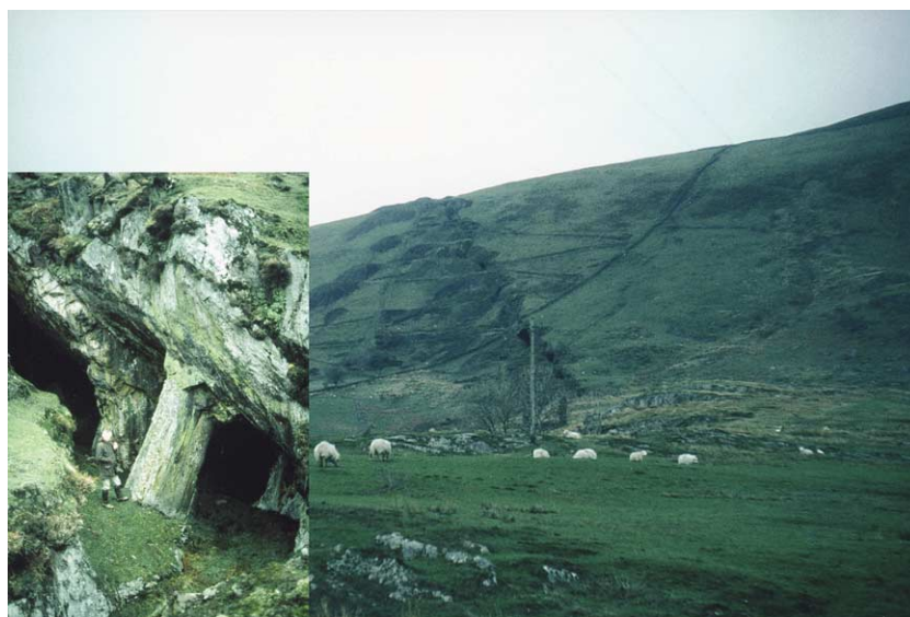
Figure 1 Ordovician ironstones, Betws Garmon, North Wales, UK (inset showing the steeply inclined stoping method of underground mining for the deposit and a residual pillar of magnetite-rich material).
