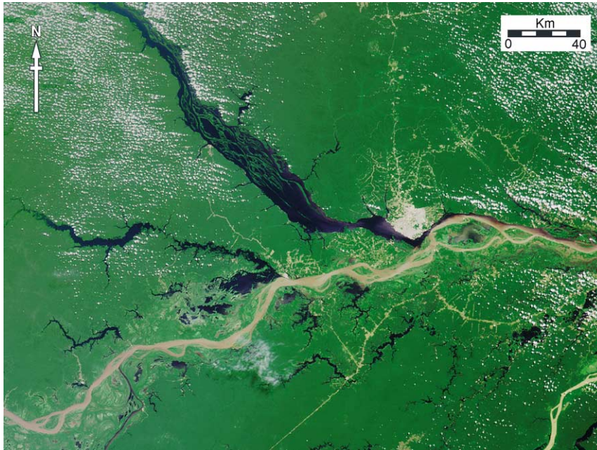
Figure 3 Satellite remote sensing image of the confluence between the sediment laden Rio Solimoes (showing brown) and the clear waters of the Rio Negro (showing black) to form the Amazon River. The Solimoes crosses soft glacial silt and sand, whereas the Negro passes through old hard rocks resistant to weathering. The two water bodies remain essentially separate for tens of kilometres downstream of the confluence. (Picture taken from the TERRA satellite using the multi angle imaging spectroradiometer on 23/7/2000.)
