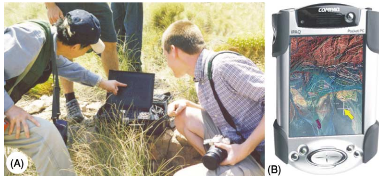
Figure 3 GIS in the field: (A) Staff and students record their observations on a digital map, in real-time, using a GPS handset, GIS and laptop, during fieldwork in Spain; (B) Palm-top computer, displaying a geo-referenced Landsat 7 satellite image being used as a base map, within GIS, for field geological mapping.
