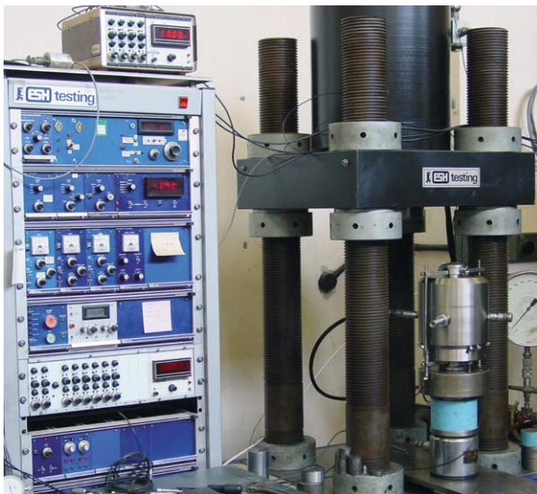
Figure 4 A servo-controlled testing machine. To the left is the stack of control electronics. In front of the loading frame (to the right) is an assembly comprising a triaxial test cell, axial strain transducers, and load cell.
