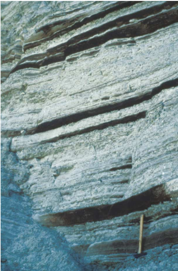
Figure 21 Petroleum migration along high-permeability sandstone beds within a stacked sequence of turbidite sandstones and siltstones. The migration route was exposed during the excavation of a road cutting in Ecuador. Photograph by M. Heffernan. Reproduced from England WA, Mackenzie A, Mann D, and Quigley T (1987) The movement and entrapment of petroleum fluids in the subsurface. J. Geol. Soc. , vol. 144, p. 327. London.
