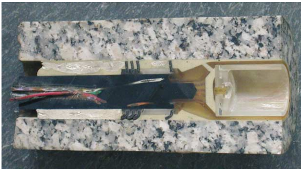
Figure 2 An overcoring device for stress estimation, sectioned after recovery from the test borehole. The control wires enter at the left; the part of the cell carrying the strain gauges, and which is cemented into the borehole, is at the right.
