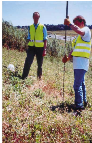
(B) Lightweight dynamic (Mackintosh) hand probing for indication of soil density
