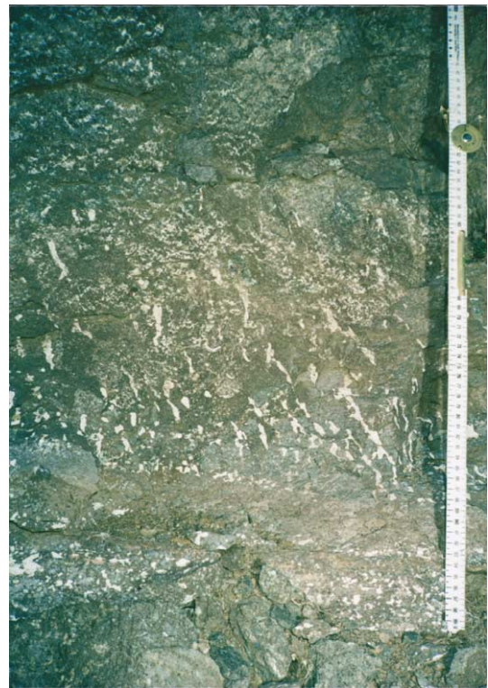
Figure 7 Amygdales and pipes in basalt, exposed in the Transfer Tunnel; Lesotho Highlands Water Scheme.
