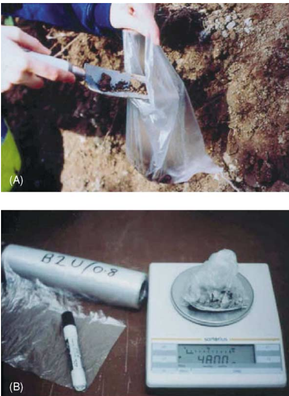
Figure 3 'Moisture in the bag'; an efficient method of determining moisture contents.
