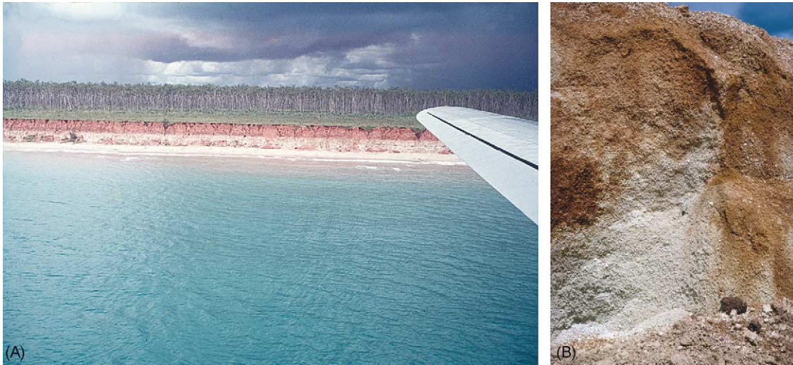
Figure 2 The cliffs facing the Gulf of Carpentaria in Queensland, Australia, and a working face in the vast expanse of pisolitic bauxite. Scale shown by white penknife near the centre. Photos: GR Davis.
