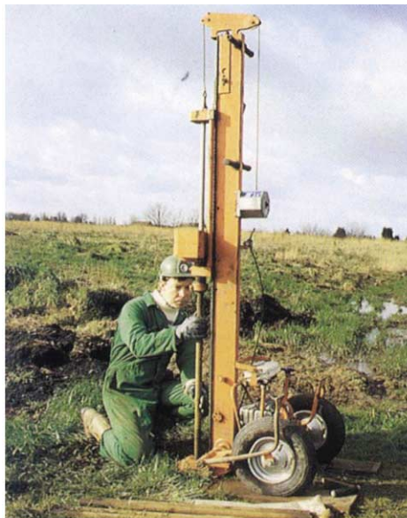
(A) Lightweight drilling, dynamic probe rig (Courtesy Exploration Associates)
