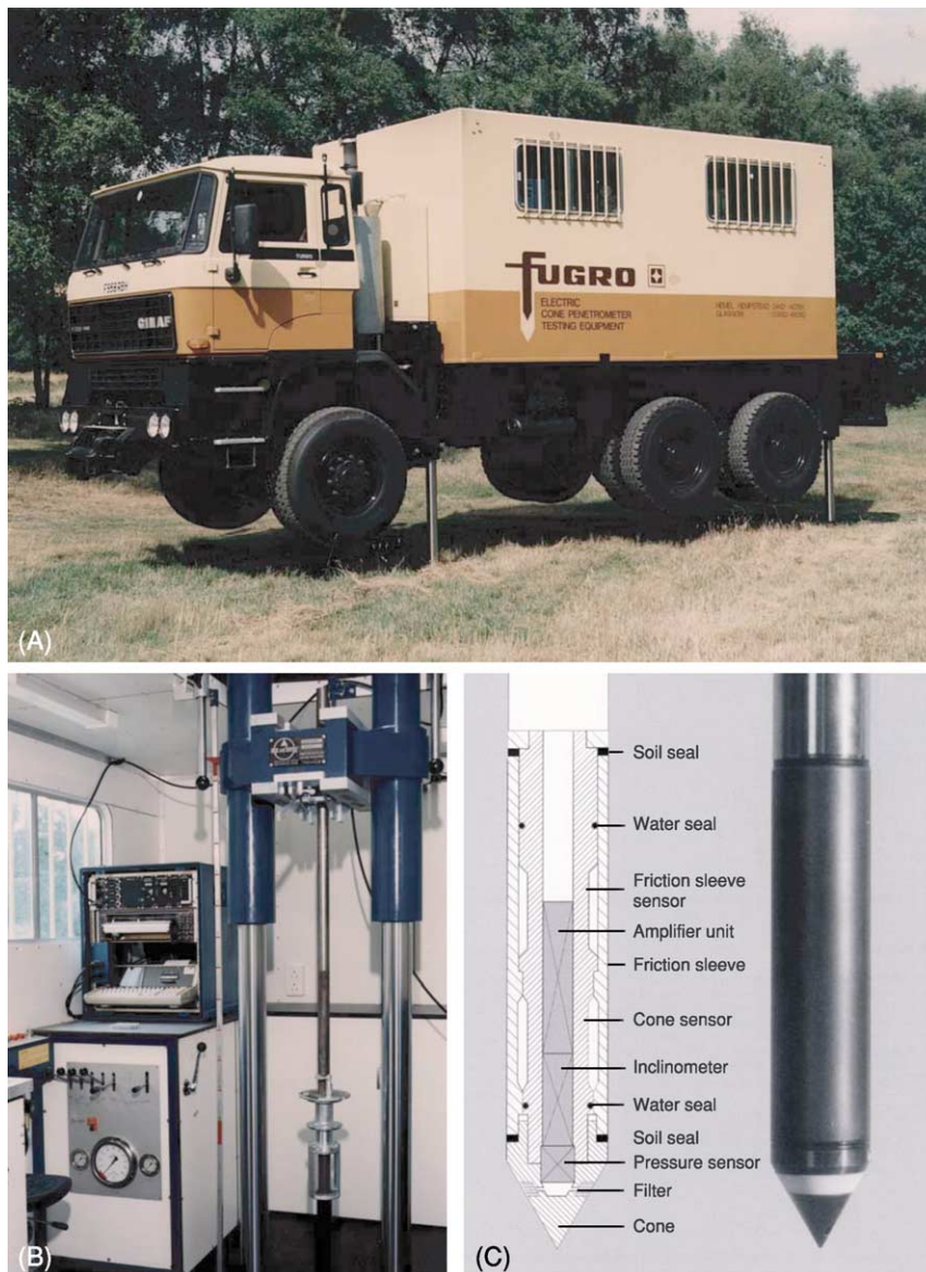
Figure 5 The static cone apparatus. (A) 'Dutch' cone penetrometer testing truck with (B) control console and (C) electric static cone (photographs courtesy of Fugro Ltd).
