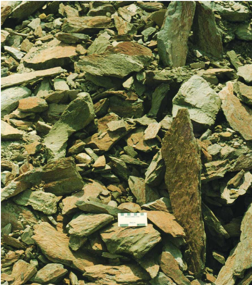
Figure 1 Engineering geologists generally work with already flawed earth materials. This weak rock of Pennsylvanian age at Little Rock, Arkansas, needs to be ripped on excavation, yet it is wholly discontinuous and platy.
