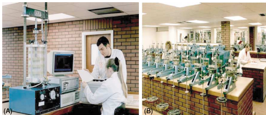
Figure 7 Commercial laboratory testing for shear strength and consolidation. (A) A 100 mm triaxial test cell. (B) A bank of consolidation (oedometer) test machines. (Photographs courtesy of CSL Ltd.)
