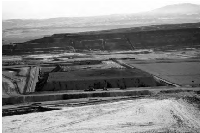
Figure 6. One of the three biooxidation pretreatment heaps measuring approximately 1,000 by 500 feet, with ore stacked to 30 feet, containing 709,000 tons of low-grade refractory ore. Courtesy of Dr. J. Brierley, Newmont Mining Corporation. See color insert.
