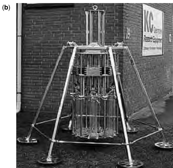
Figure 9. Examples of sediment corers. (a) Diagram of a box corer with the frame, weights, and sample tube enumerated, respectively. (b) Image of a multicorer with detachable legs, gyro-suspension, and polycarbonate sampling tubes. Both images were provided courtesy of KC Denmark ( http://www.kc-denmark.dk/ ). See color insert.
