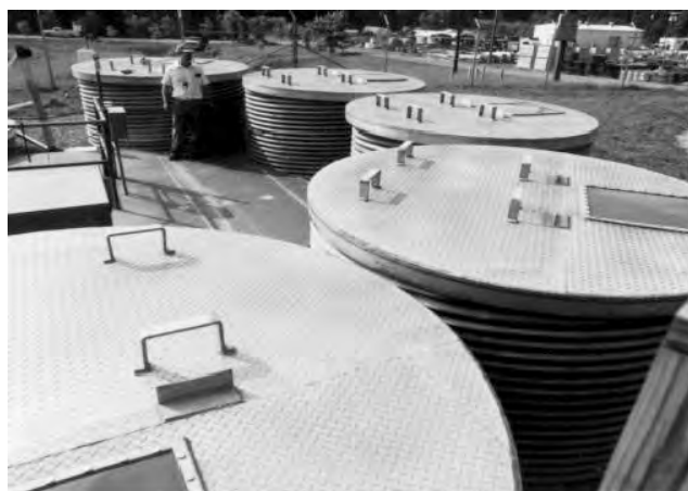
Figure 2. Physical containment of GEMs within a lysimeter structure. Lysimeters were 4 m deep by 2.5 m in diameter and filled with polyaromatic hydrocarbon-contaminated soil to study bioremediation-monitoring capabilities of an introduced GEM (33).
