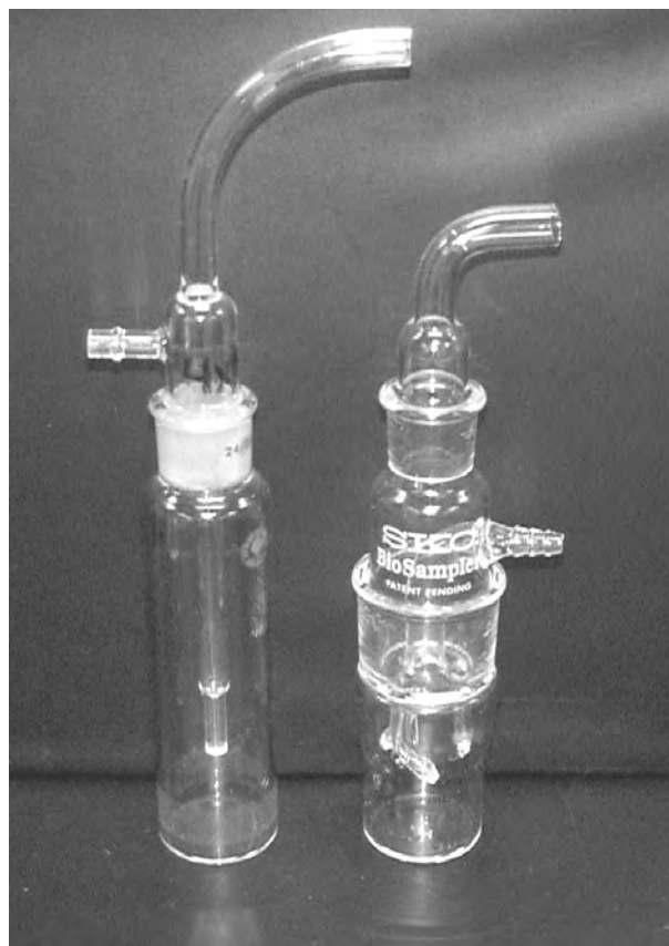
Figure 4. AGI-30 sampler (left) and SKC BioSampler (right) (courtesy of Paula Jacoby-Garrett, UNLV).
