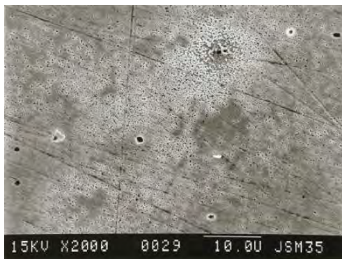
Figure 4. Scanning electron micrograph demonstrating localized corrosion on the surface of AISI 316 stainless steel following the removal of a 14-day-old biofilm formed in a pure culture of the marine sulfate-reducing bacterium Desulfovibrio indonensis . Corrosion is visible as pitting attack of varying intensity.
