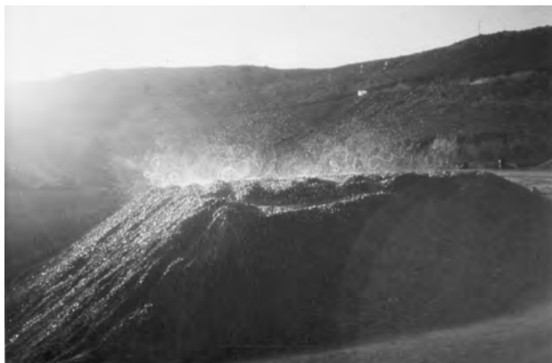
Figure 2. Dump bioleaching of copper ore in Peru. The dump is irrigated by sprinklers with acidified water.
