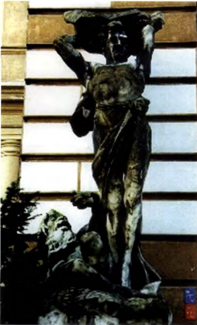
Biodeterioration of Mineral Materials, Figure 1. Discolored stone statue in Karlovy Vary, Czech Republic, showing growth of mainly mitosporic fungi and cyanobacteria.
