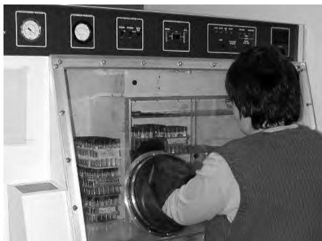
Figure 3. Anaerobic chambers can be used to grow bacteria under defined atmospheric conditions. The gaseous composition can be manipulated to mimic natural environmental conditions. See color insert.
