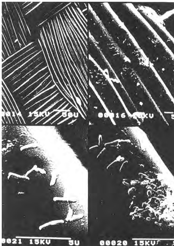
Figure 2. Permeate side of a reverse osmosis membrane; bacteria are attached and can contaminate the permeate (Courtesy of H. F. Ridgway, in B. S. Parekh, ed., Reverse Osmosis Technology , Marcel Dekker, New York, Basel, 1988, pp. 429–481).
