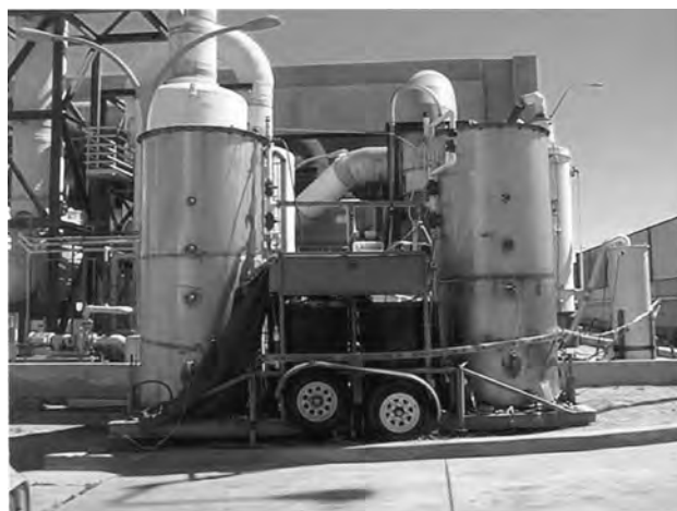
Figure 5. Picture of the UCR biotrickling filter installed at Hyperion Wastewater Treatment Plant in Los Angeles.
