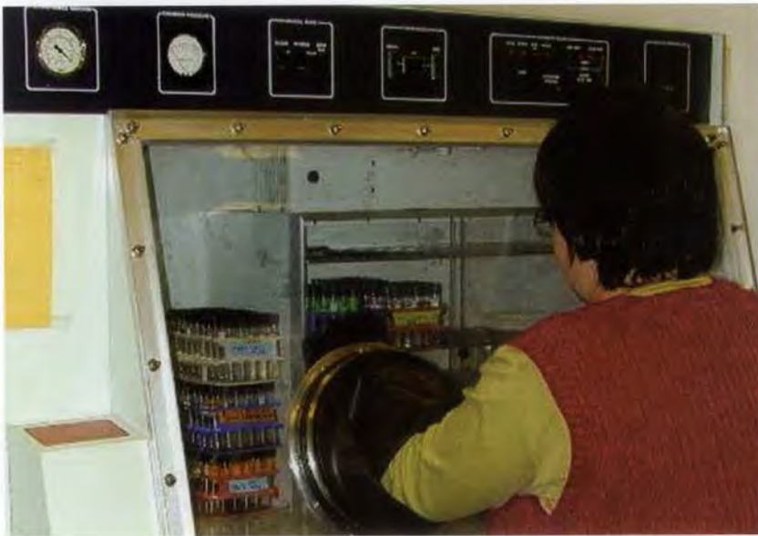
Methods for the Identification of Microbial Isolates, Figure 3. Anaerobic chambers can be used to grow bacteria under defined atmospheric conditions. The gaseous composition can be manipulated to mimic natural environmental conditions.
