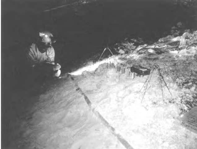
Figure 4. Long-term aerial colonization study is set in place by caver D. Hamer. Country rock machined into slides, polished, sterilized, and hung on a sterile apparatus will be left in place in an off-limits area of Lechuguilla Cave, New Mexico. This experiment is testing whether there is aerial transport of organisms through the cave air circulation cells and colonization on new rock surfaces. Experiments of this nature can run for many years before showing results. Image courtesy of V. Hildreth-Werker.
