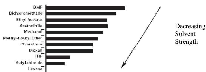
Fig. 3 Solvent strength data on porous graphitized carbon columns for the retention of aniline, naphthalene, ethyl benzene, and phenol.
