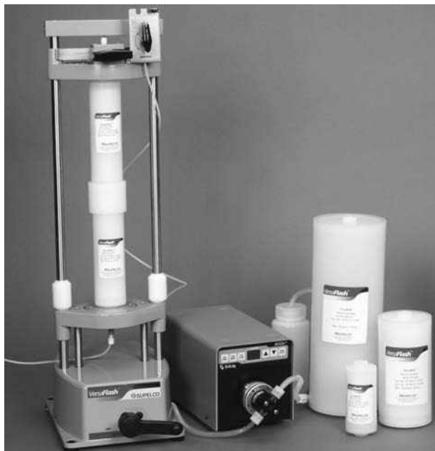
Fig. 1 VersaFlash high throughput flash purification (HTFP) system shown with two stacked prepacked 40 \times 75 mm (51 g) cartridges inserted in the support stand and 110 \times 300 mm (1.35 kg), 80 \times 150 mm (410 g), and 23 \times 110 mm (23 g) cartridges on the right side of the eluent pump. The 3-way valve injector at the upper right allows direct application of sample onto cartridges using a syringe. The outlet tubing can be used for manual sample collection or connection to an automated fraction collector or UV detector.
