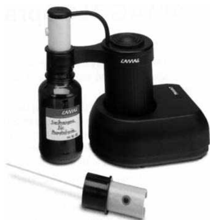
Fig. 3 TLC sprayer consisting of a charger and pump unit; homogeneous reagent aerosol particles in the 0.3–10 µm range are formed. Source: Photograph supplied by Camag, Wilmington, North Carolina.
