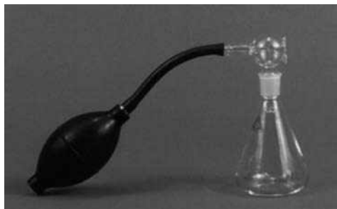
Fig. 2 Glass TLC reagent sprayer for use with an air line or the rubber bulb shown. Source: Photograph supplied by Analtech.
