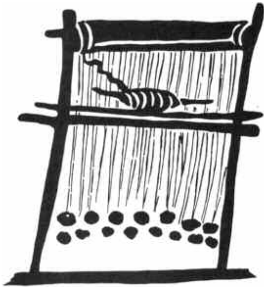
5.4 Various elements of the upright loom, as depicted on a black figure vase, including the vertical warp threads with weights
